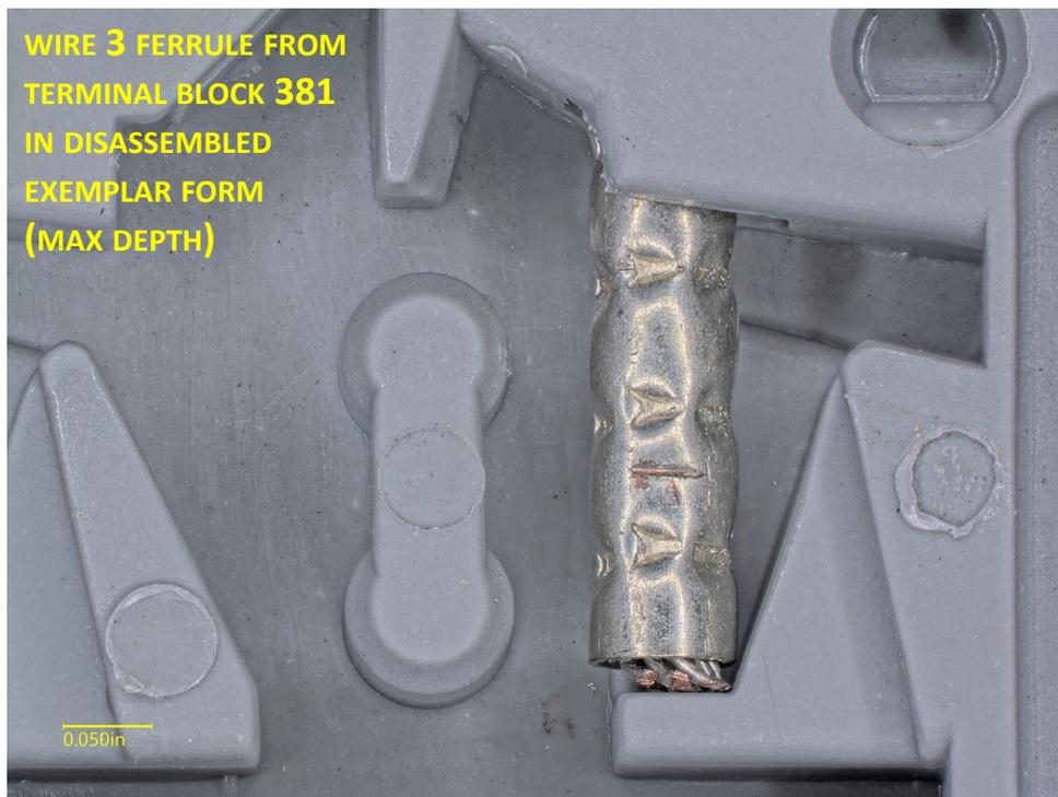
**Figure 34.** Digital microscope images of the ferrules from wires 1 and 3 from Terminal Block 381 inserted inside the corresponding connection points in a disassembled polymer form from an exemplar terminal block. Both wires were inserted to the maximum depth possible into the cage areas of the connection points.
