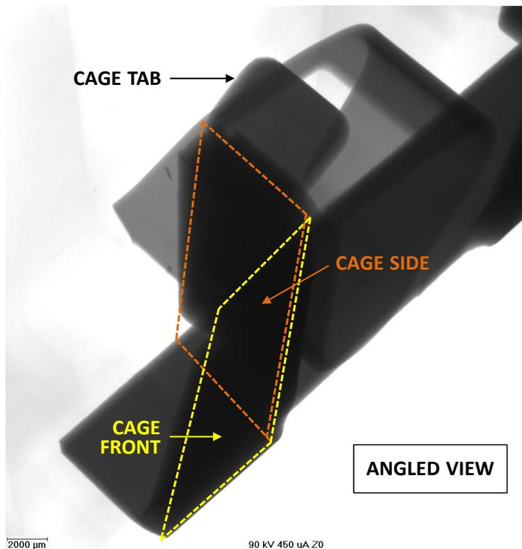
**Figure 6.** Digital microscope and x-ray images (top and bottom, respectively) of a terminal block with conductor bar cage components labeled.
