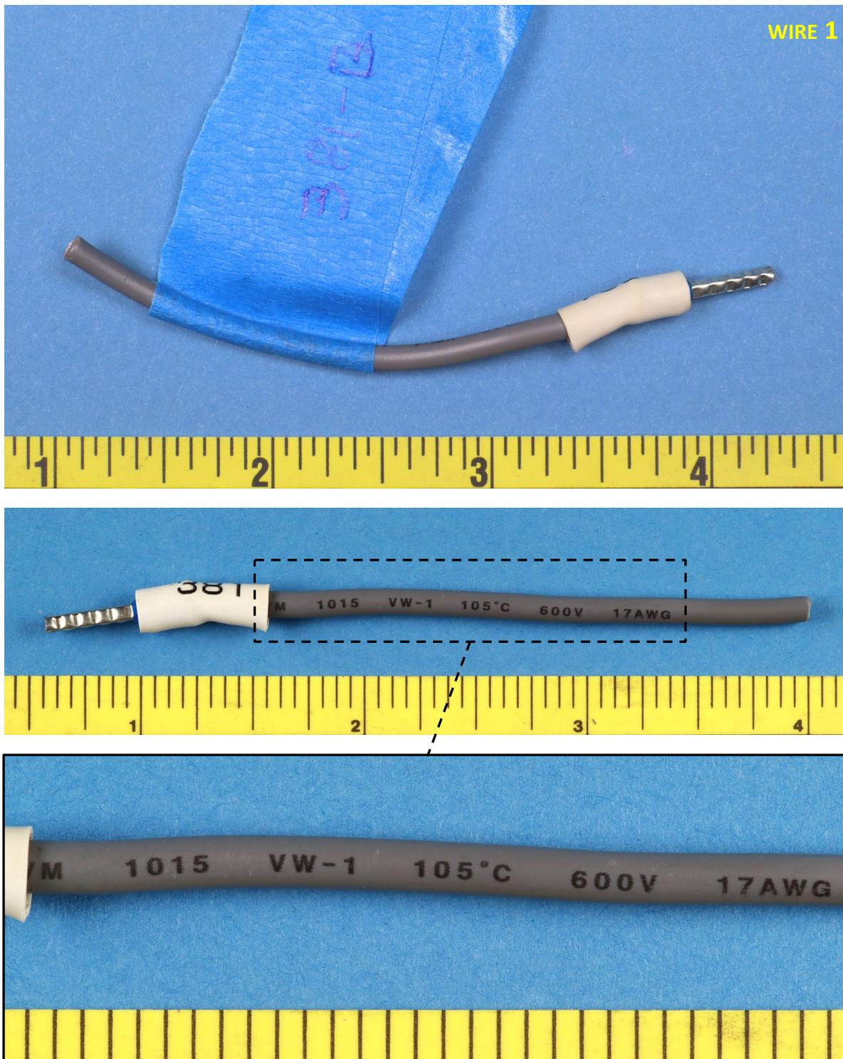
**Figure 20.** Macro photos of the submitted portion of the wire assembled to connection point 1 in Terminal Block 381 in the as-submitted condition and after identifying tape was removed (first and second images, respectively). A close-up photo of the identifying marks on the wire is shown in the third image.
