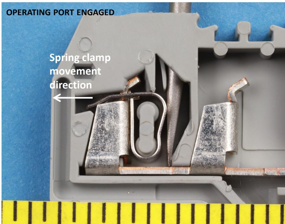
**Figure 7.** Close-up photos showing the movement of a spring clamp when a tool is installed in the operating port of connection point 1 on an exemplar terminal block.
