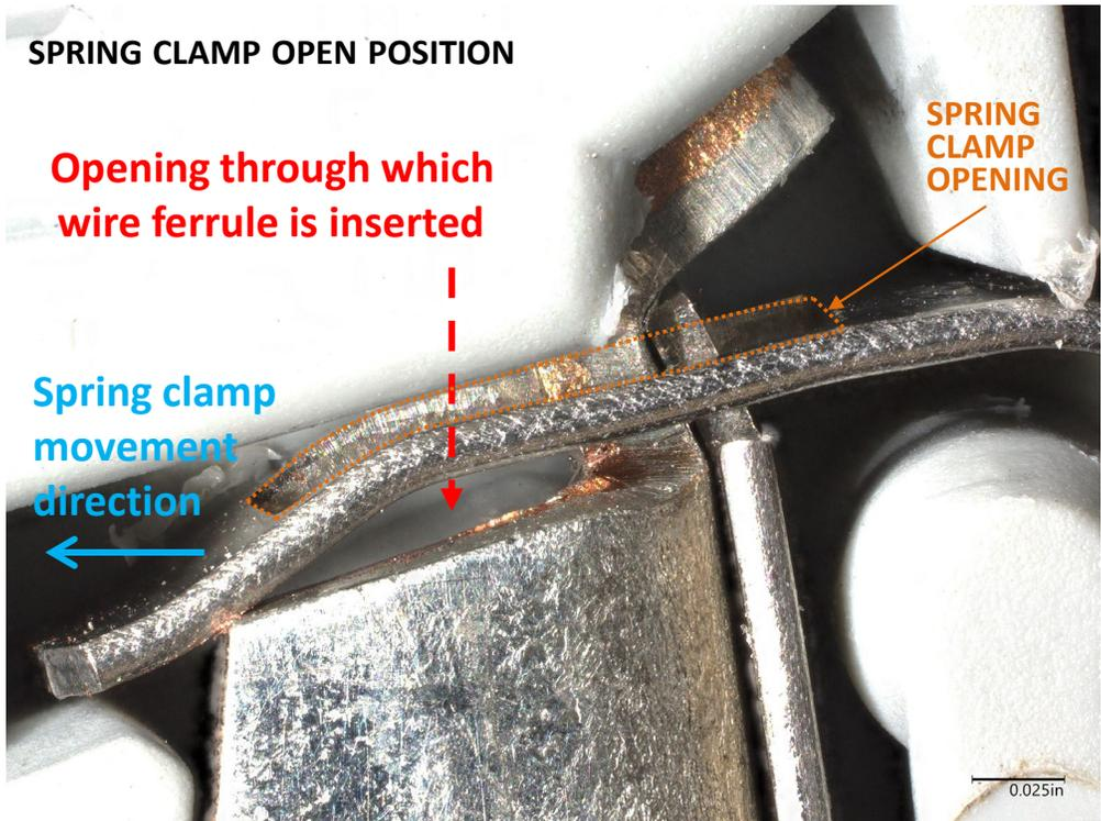
**Figure 8.** Digital microscope images showing the movement of a spring clamp when a tool is installed in the operating port of connection point 1 on an exemplar terminal block.
