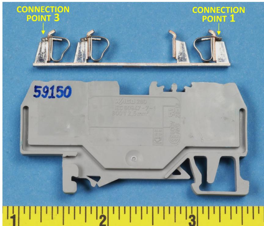
**Figure 15.** Close-up photos showing the two sides of Terminal Block 381 after disassembly.
