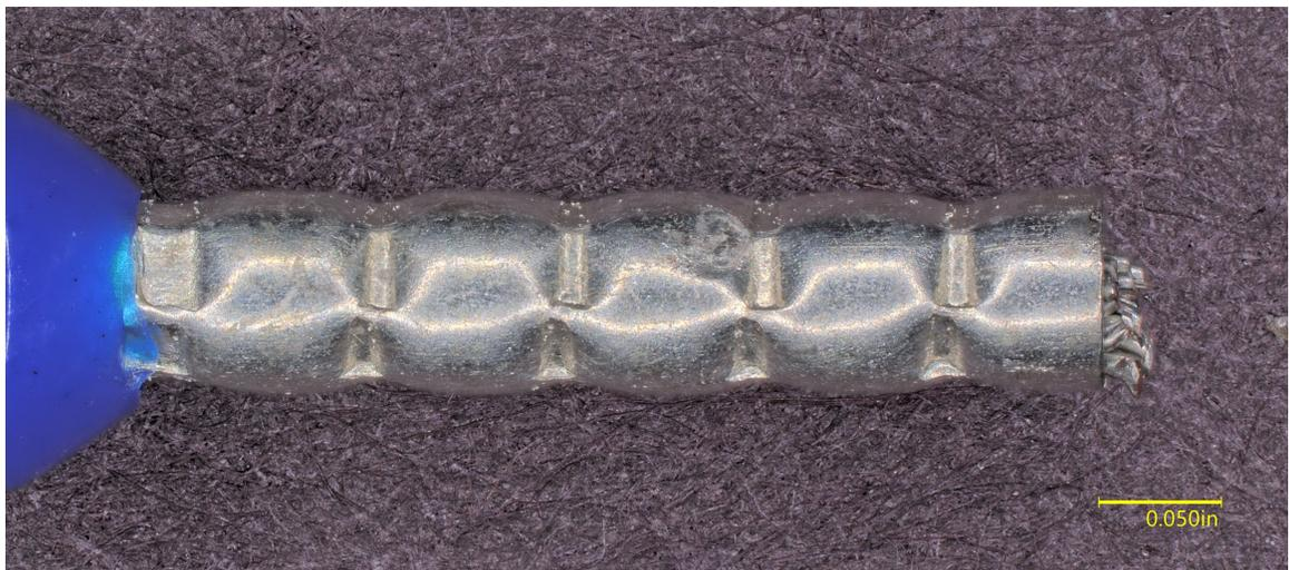
**Figure 25.** (Top) Macro photo of the submitted portion of the wire assembled to connection point 3 in Terminal Block 381. (Middle and Bottom) Digital microscope images of opposing sides of the wire 3 ferrule.
