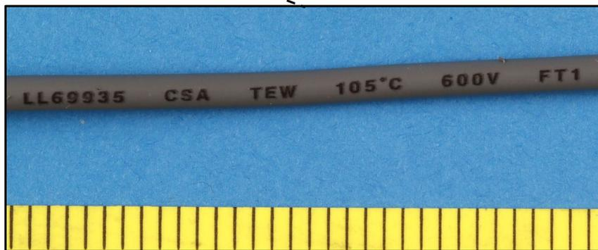
**Figure 24.** Macro photos of the submitted portion of the wire assembled to connection point 3 in Terminal Block 381 in the as-submitted condition and after identifying tape was removed (first and third images, respectively). Close-up photos of the identifying marks on the wire are shown in the second and fourth images.
