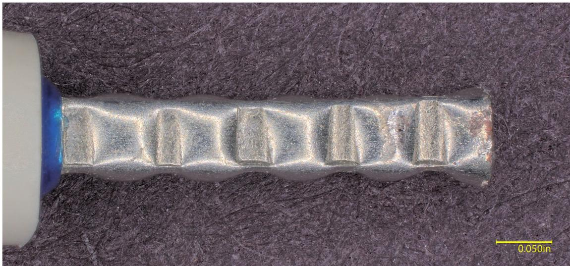
**Figure 21.** (Top) Macro photo of the submitted portion of the wire assembled to connection point 1 in Terminal Block 381. (Middle and Bottom) Digital microscope images of opposing sides of the wire 1 ferrule.
