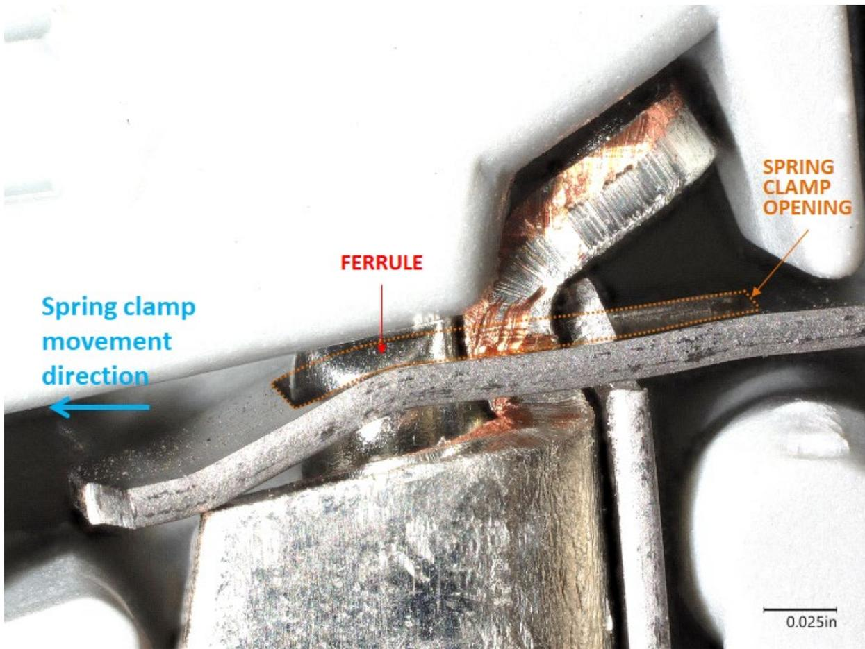
**Figure 9.** Digital microscope image showing a wire ferrule installed within a cage and secured by a spring clamp in connection point 1 on an exemplar terminal block.
