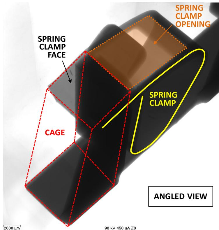
**Figure 5.** Digital microscope and x-ray image (top and bottom, respectively) of a terminal block with conductor bar spring clamp components labeled.
