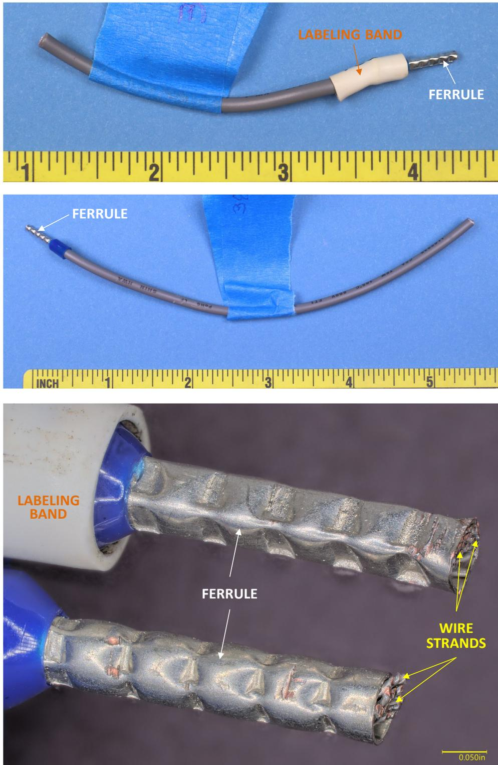
**Figure 3.** Macro photos (top and middle) and digital microscope image (bottom) of wires with components labeled.
