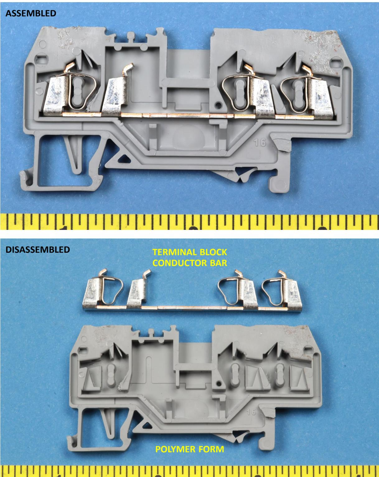
**Figure 1.** Macro photos showing a terminal block assembled and disassembled.
