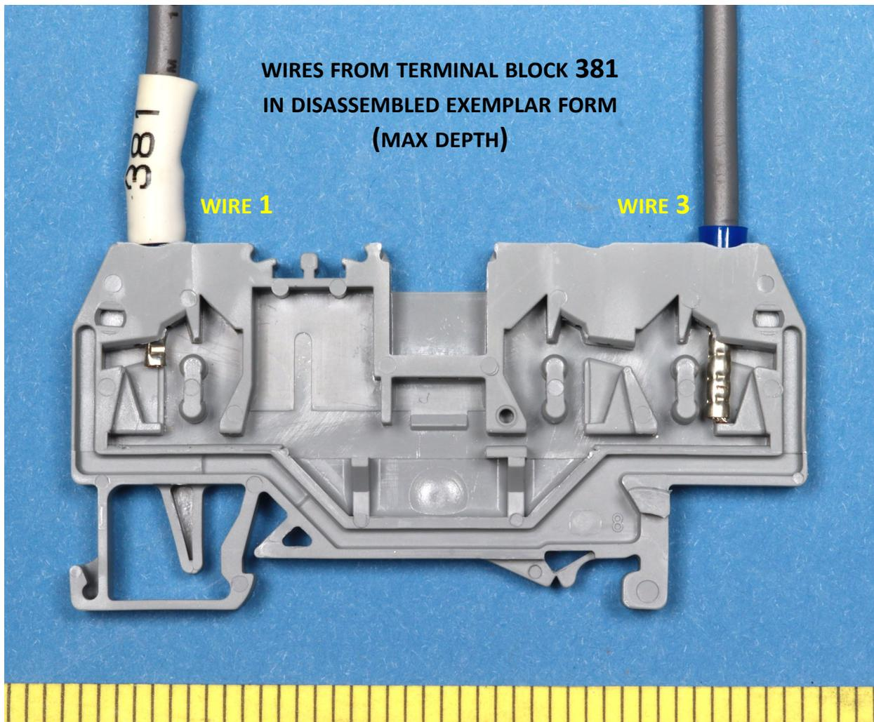
**Figure 35.** Macro photo showing wires 1 and 3 from Terminal Block 381 inserted inside the corresponding connection points in a disassembled polymer form disassembled from an exemplar terminal block. Both wires were inserted to the maximum depth possible into the cage areas of the connection points.
