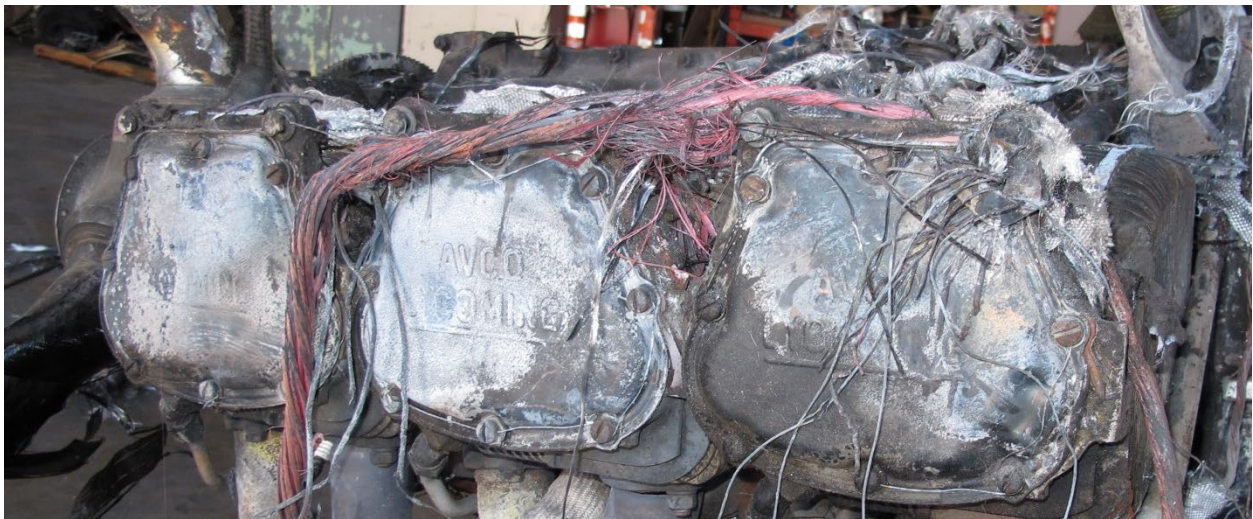
Figure 7. Thermal damage to cylinder covers (Cylinders 2, 4 & 6).
