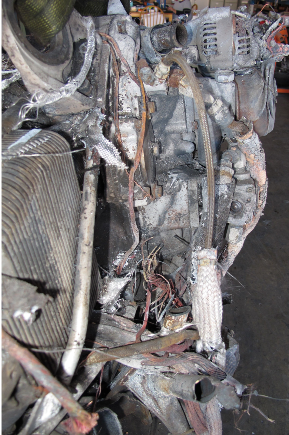
Figure 9. Burn pattern on accessory case.
