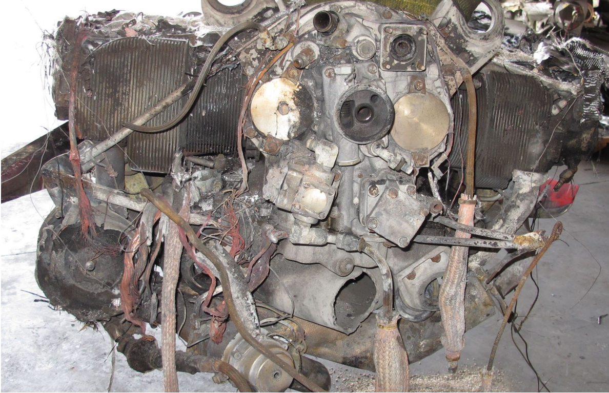
Figure 8. Accessory area of engine (forward section of engine).
