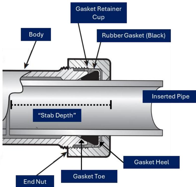
**Figure 14.** Cross-section drawing of a Dresser "Seal Only" Style 90 gas service fitting. Adapted from recent Dresser marketing materials.<sup>32</sup>
