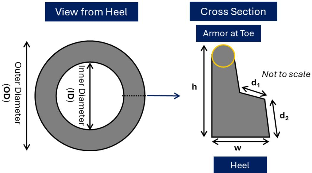
**Figure 24.** Schematic of the measurements taken on the deformed gaskets using calipers.
