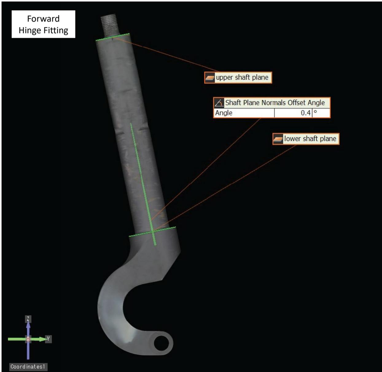
**Figure 6.** Modeled view of the forward hinge fitting showing planes constructed on the top surface and base of the shaft and measured bend angle between the plane normal vectors.
