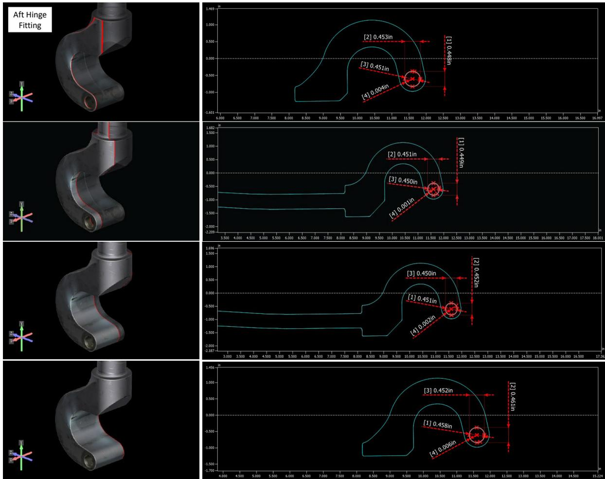
**Figure 8.** Section cut locations through the aft hinge fitting (left, red lines) and the associated 2D profile of the part at the section cut (right) progressing from forward to aft (top to bottom). Measured values of the attachment hole are indicated in the 2D profile views.
