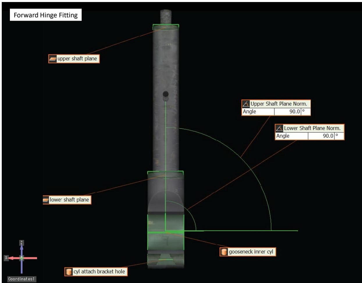
**Figure 7.** Modeled view of the forward hinge fitting showing cylinder elements constructed along the internal gooseneck and attachment hole regions, planes constructed on the top surface and base of the shaft, and measured bend angles between the cylinder axes and plane normal vectors.
