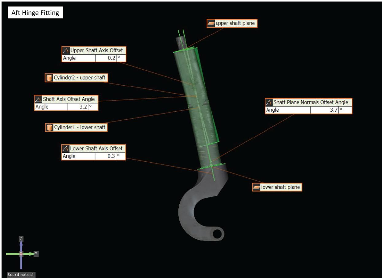
**Figure 4.** Modeled view of the aft hinge fitting showing cylinder elements constructed along the upper and lower shaft regions, planes constructed on the top surface and base of the shaft, and measured bend angles between the cylinder axes and plane normal vectors.
