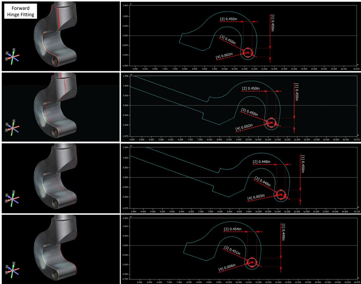
**Figure 9.** Section cut locations through the forward hinge fitting (left, red lines) and the associated 2D profile of the part at the section cut (right) progressing from forward to aft (top to bottom). Measured values of the attachment hole are indicated in the 2D profile views.
