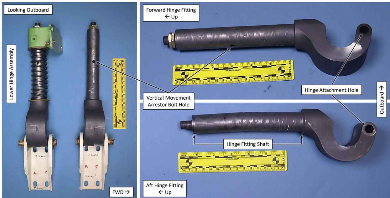
**Figure 1.** Photographs showing the MED plug hinge assemblies (left) and after disassembly to isolate the forward and aft hinge fittings (right).
