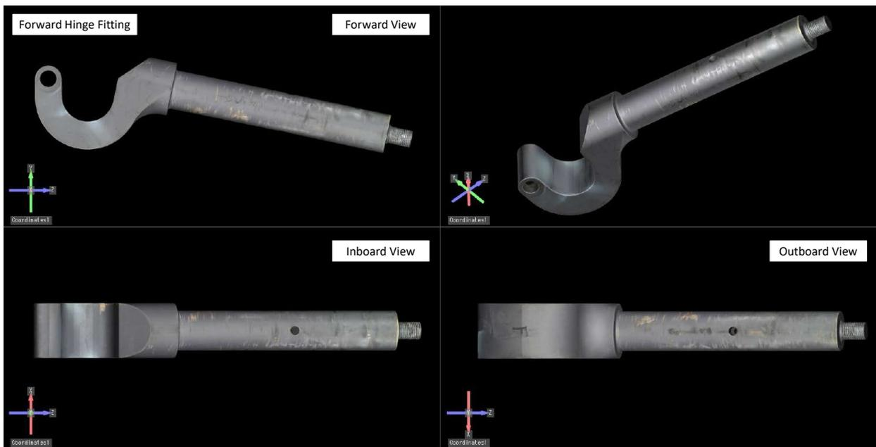
**Figure 3.** Modeled views of the forward hinge fitting from 3D scan data.
