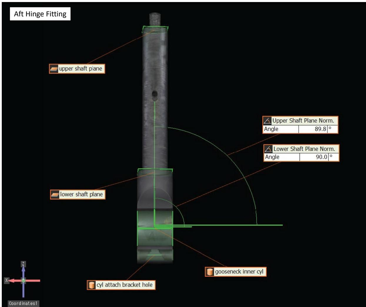
**Figure 5.** Modeled view of the aft hinge fitting showing cylinder elements constructed along the internal gooseneck and attachment hole regions, planes constructed on the top surface and base of the shaft, and measured bend angles between the cylinder axes and plane normal vectors.
