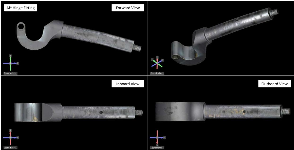
**Figure 2.** Modeled views of the aft hinge fitting from 3D scan data.
