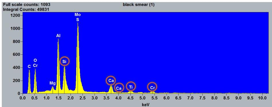
**Figure 41.** EDS spectrum of a smeared black deposit below the vertical movement arrestor bolt hole shown at the right in figure 40. Circled peaks were also detected in the enamel and/or primer spectra shown in the next figure and were largely absent from other sampled areas of the hinge fitting.
