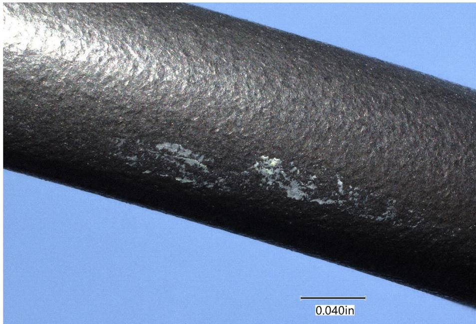
**Figure 44.** White and green material deposited on the surface of the aft lift assist spring.
