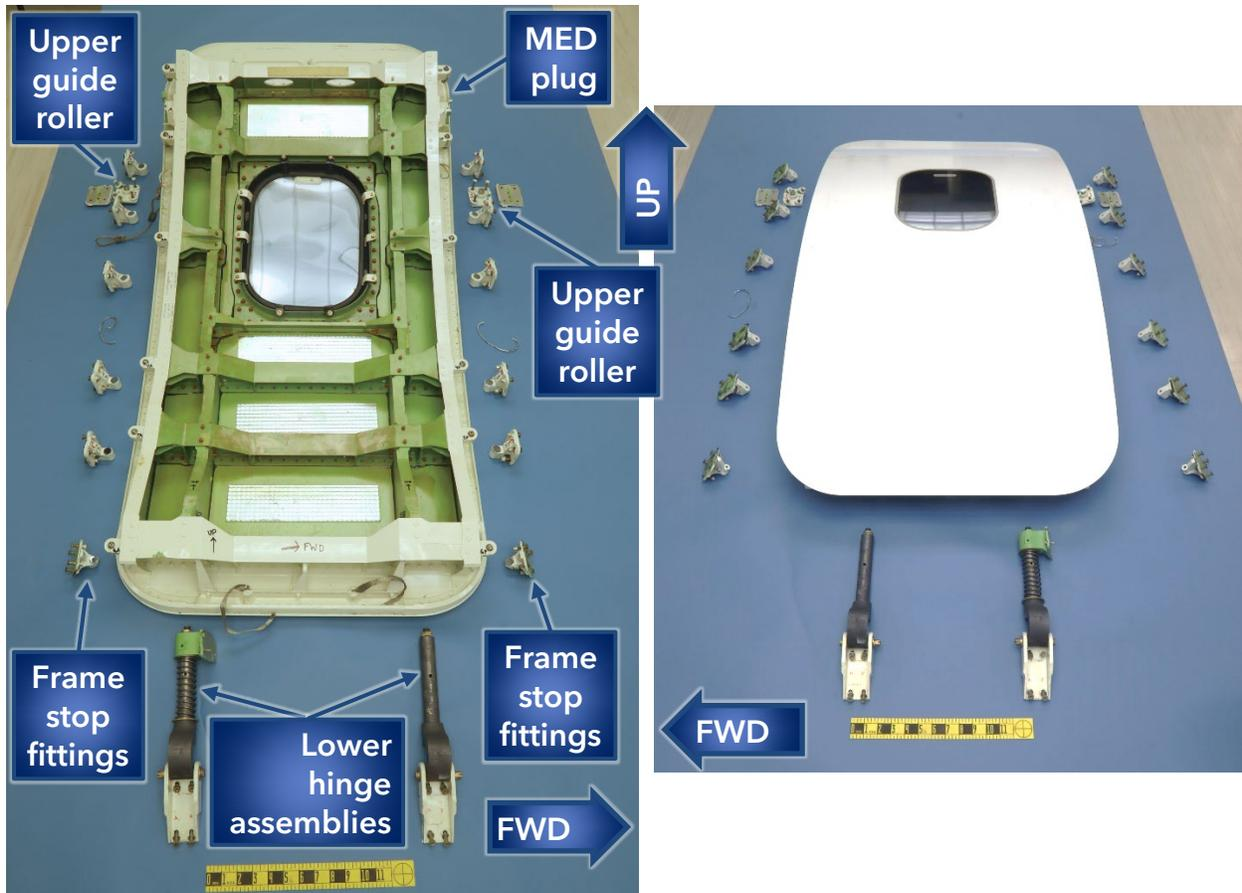
**Figure 1.** Overall views of the submitted left MED plug and associated components showing an interior view (left image) and exterior view (right image).
