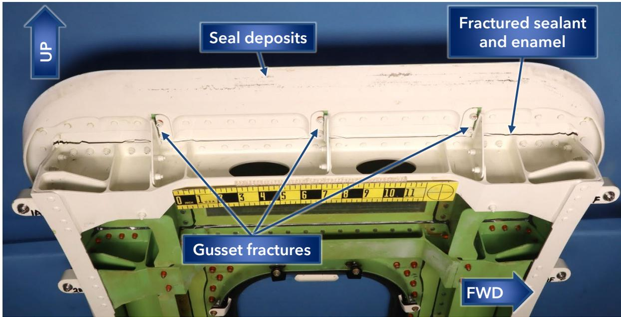
**Figure 47.** Overall view of the upper end of the left MED plug.
