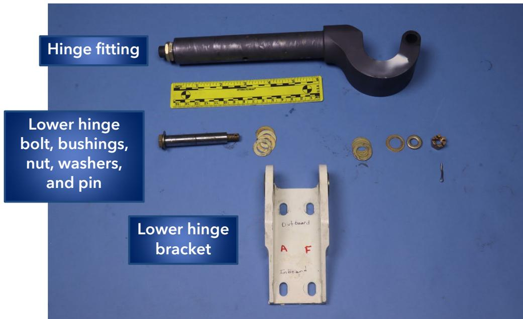
**Figure 35.** Forward lower hinge assembly components, lower hinge bracket assembly, and associated hinge fitting attachment hardware after disassembling the hinge fitting from the lower hinge bracket assembly.
