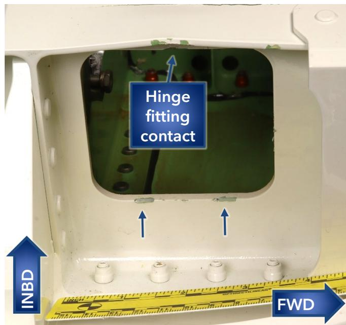
**Figure 45.** The left image shows a contact mark (unlabeled arrow) observed on the upper end of the forward hinge shaft, outboard side. The right image shows another view of the forward hinge opening in the lower end of the left MED plug where unlabeled arrows point to contact marks on the outboard edge of the opening with a spacing corresponding to the distance between the hinge guide flange and the hinge shaft centerline.
