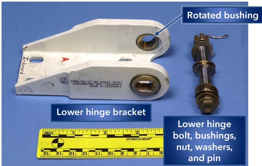
**Figure 36.** Aft lower hinge bracket assembly and associated hinge fitting attachment hardware after disassembly.
