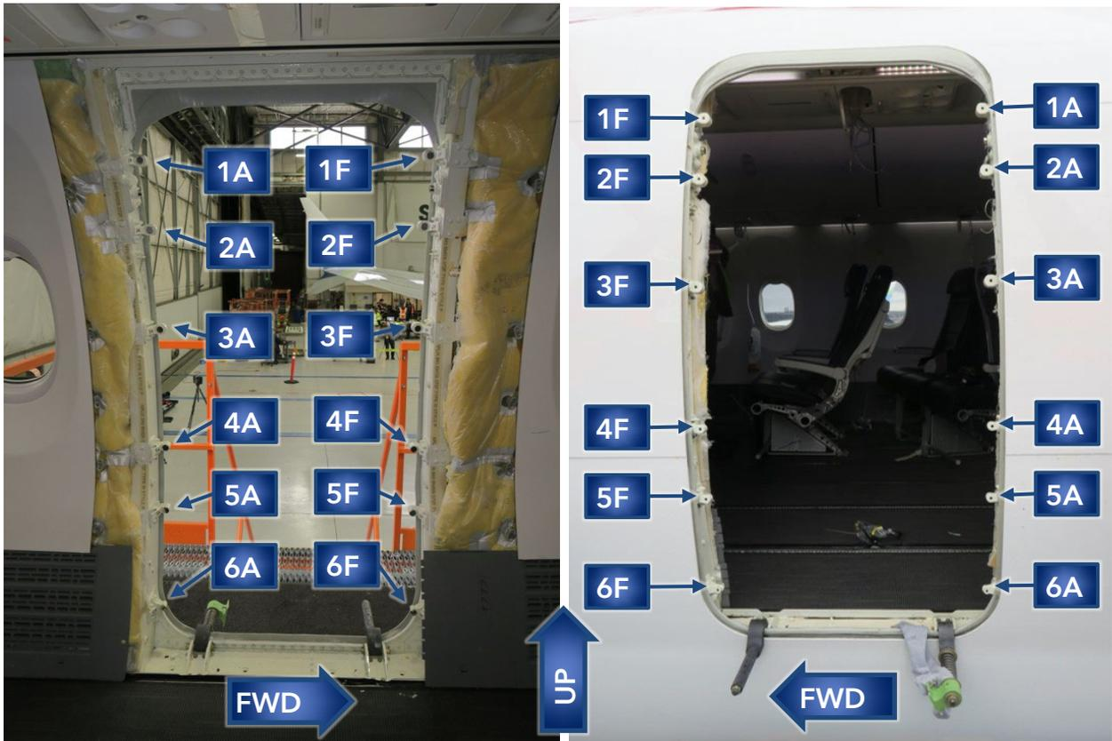
**Figure 8.** Interior (left image) and exterior (right image) views of the left MED opening in the fuselage after nearby passenger seats were removed. Frame stop fittings are indicated as labeled on scene.
