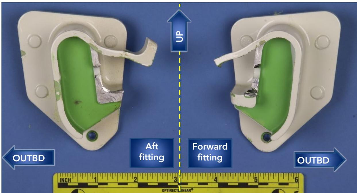
**Figure 21.** Forward and aft upper guide fittings after disassembly from the left MED plug.
