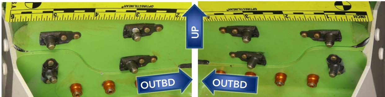
**Figure 28.** Nut plates and threaded ends of the hinge guide fitting attachment bolts for the forward (right image) and aft (left image) hinge guide fittings on the left MED plug.
