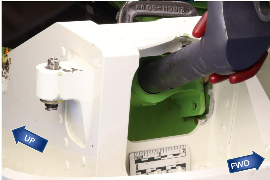
**Figure 43.** Images of the partially reassembled aft hinge fitting assembly with the hinge shaft positioned next to corresponding contact damage at the lower end of the MED plug as viewed from below (lower image) and from above (upper image).
