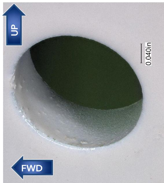
**Figure 23.** Close views of the upper guide track bolt holes in the aft upper guide fitting from the left MED plug. The forward face of the inboard hole is shown in the upper image, and views of the lower side of the hole bores on the inboard and outboard holes are shown in the lower left and lower right images, respectively. Unlabeled arrows in the upper image indicate faint dark deposits in a circular area around the hole.
