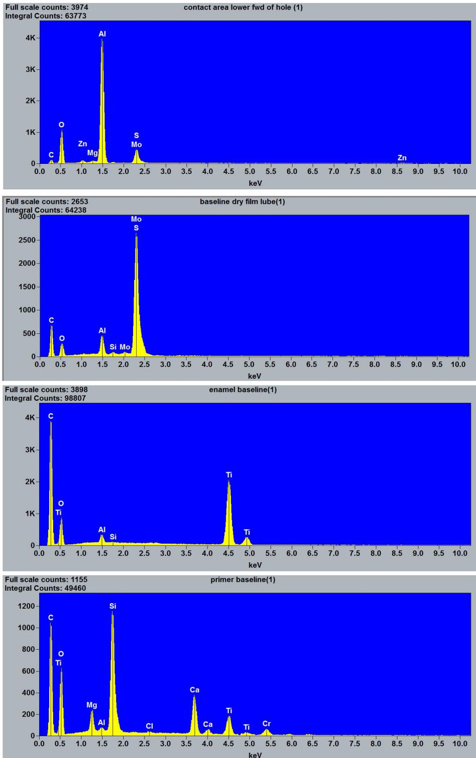
**Figure 42.** EDS spectra of a gold-colored area at the lower forward side of the hole shown in the right image in figure 40 (upper spectrum), an undisturbed surface on the hinge fitting (upper middle spectrum), a sample of the enamel coating on one of the upper guide fittings (lower middle spectrum) and the primer on the same upper guide fitting (lower spectrum).
