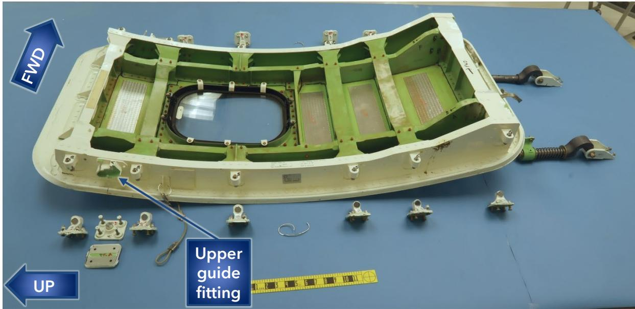
**Figure 3.** Overall view of the aft side of the submitted left MED plug and associated components.
