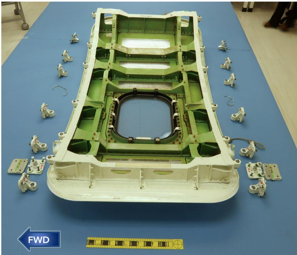
**Figure 4.** Overall view of the upper side of the submitted left MED plug and associated components.
