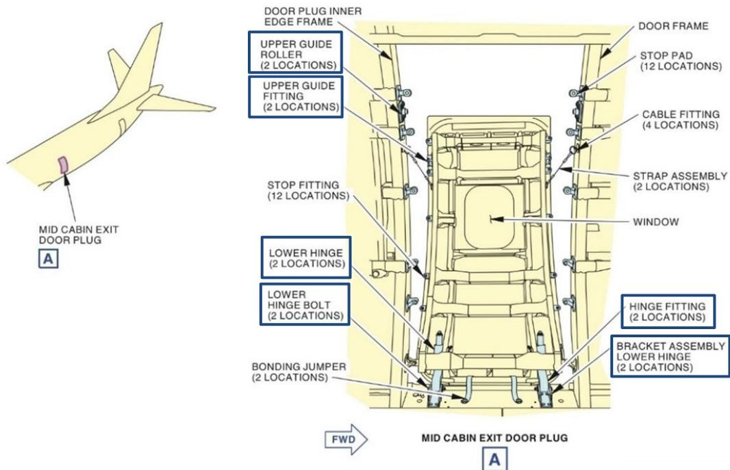
**Figure 5.** Diagram of a left MED plug in the opened condition. Items highlighted with rectangles are shown in the next figure. (Source: Boeing. Image Copyright © Boeing. Reproduced with permission.)
