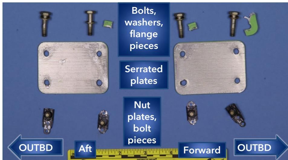
**Figure 29.** Hinge guide fitting serrated plates, attachment hardware, and flange pieces after disassembly from the left MED plug.
