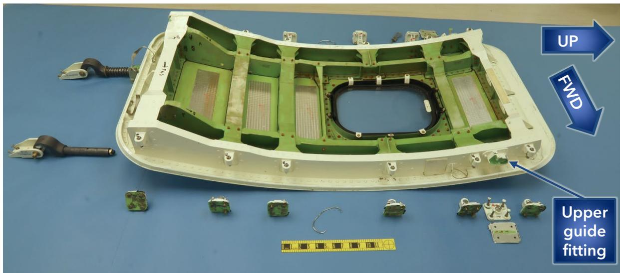
**Figure 2.** Overall view of the forward side of the submitted left MED plug and associated components.
