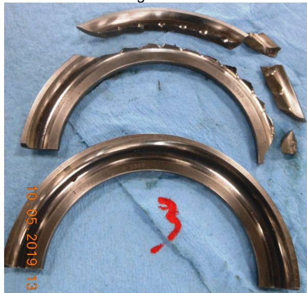
Photo #4 - Blade #3 bearing race fractured with ball imprints
