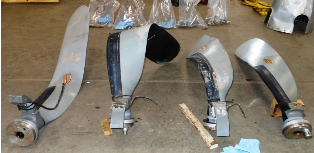
Photo #8 - Blade bend and twist comparison
