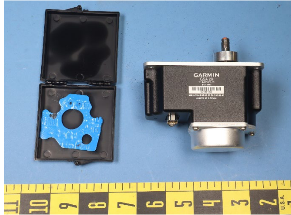
Figure 1. Overall view of the submitted servo with a separate box containing the blue thermal pad.
