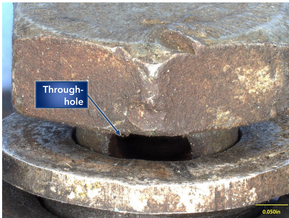
Figure 4. View of the through-hole in the shank of the trim tab attachment bolt with the spacer positioned against the nut.
