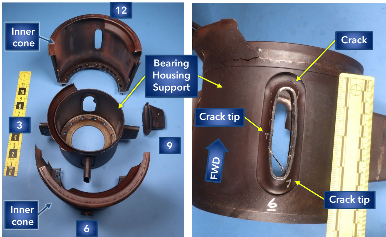
Figure 25. Views of the bearing housing support and inner struts after separating the inner cone from the support.
