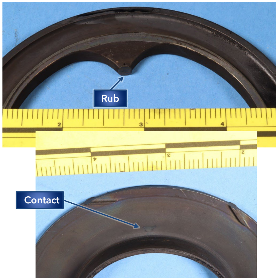
Figure 13. Retaining plate (above) and aft oil impeller (below).
