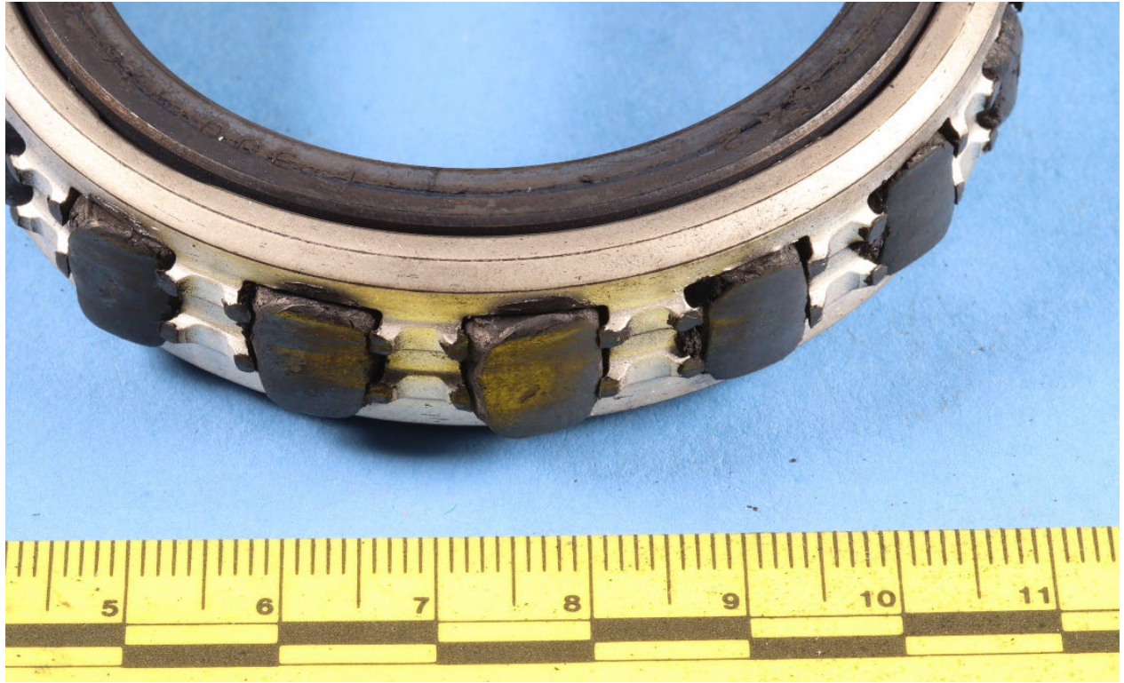
Figure 8. Number 2 bearing inner race, cage, and rolling elements (metric side of ruler shown).
