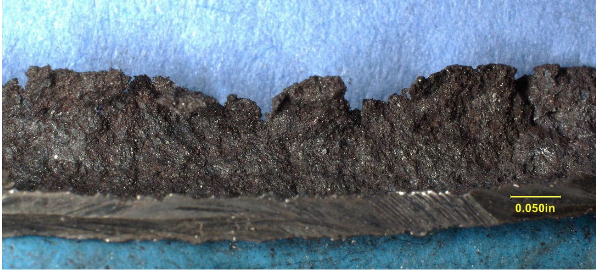
Figure 18. Piece of the rear bearing cover outer diameter flange cut from the forward piece showing the flange remnant surface on the inside of the curl.
