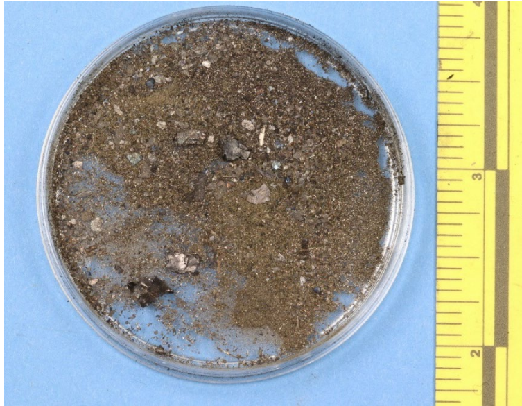
Figure 10. Debris removed from the air diffuser scavenge oil tube after cutting using an abrasive cutting tool.
