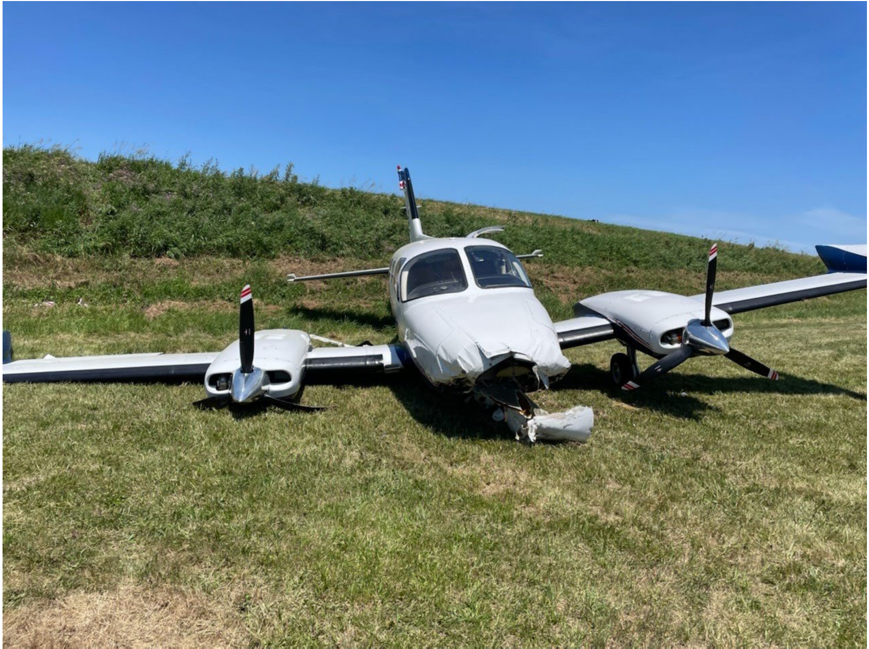
Photo 3 – View of Damaged Nose Compartment (FAA)
