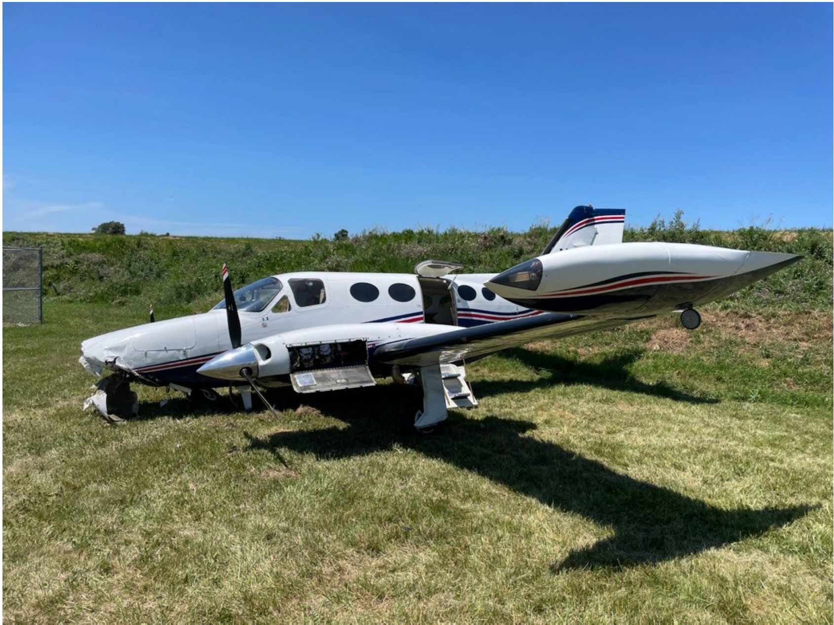
Photo 4 – View of Collapsed Nose Gear (FAA)
