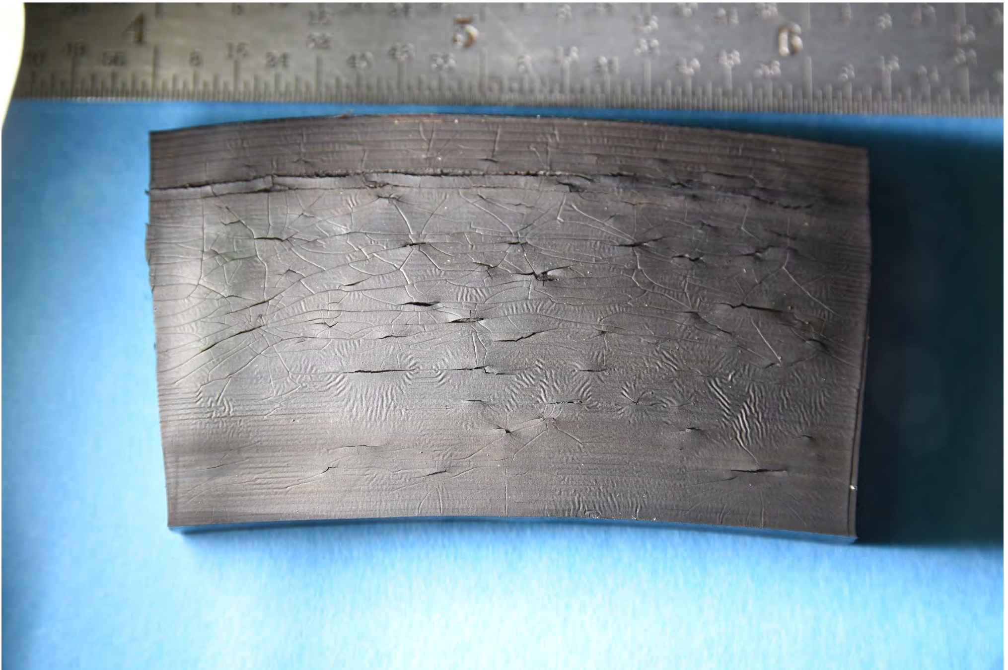
300 degrees Celsius front side burn tested
