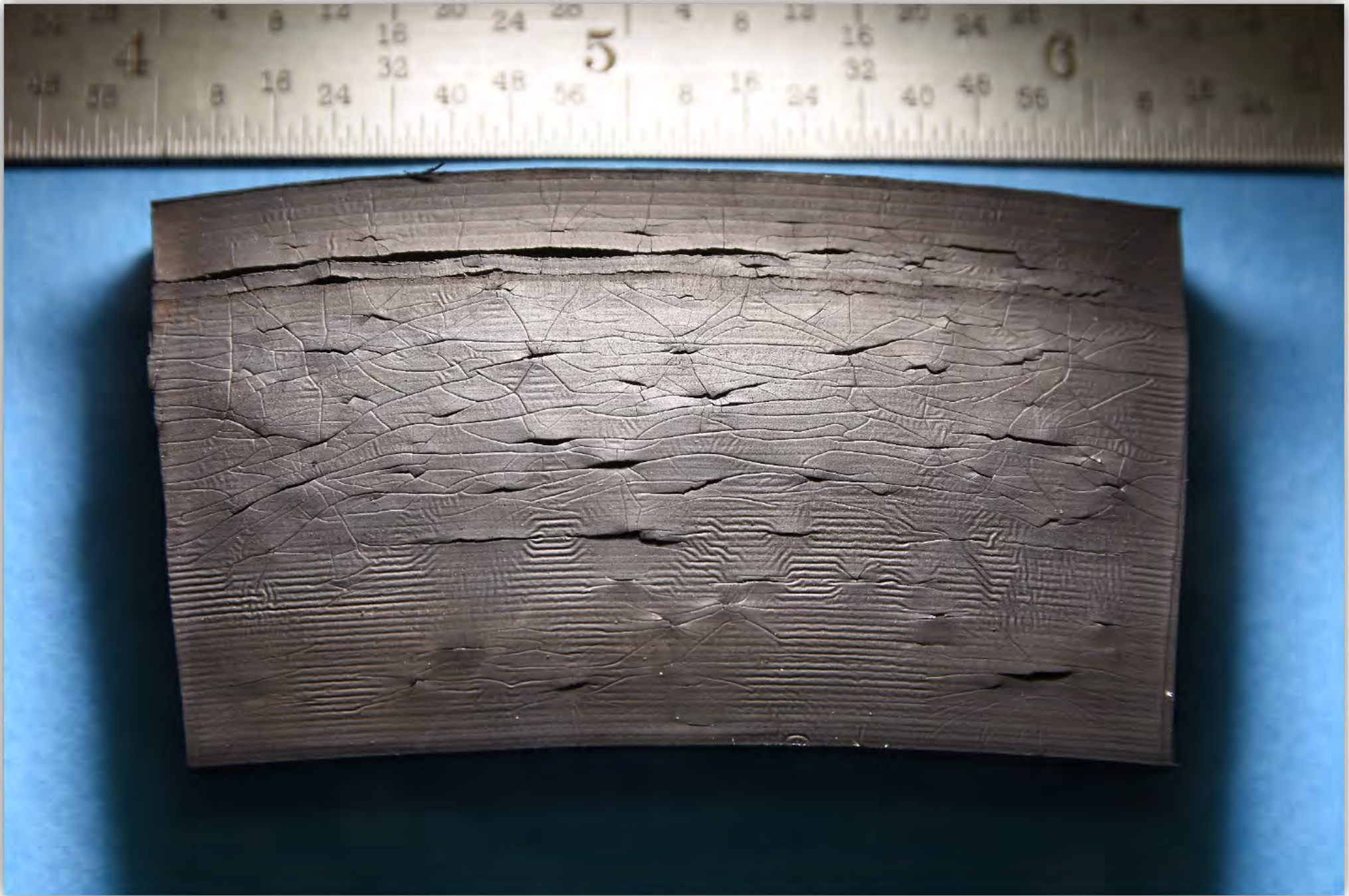
300 degrees Celsius front side burn tested
