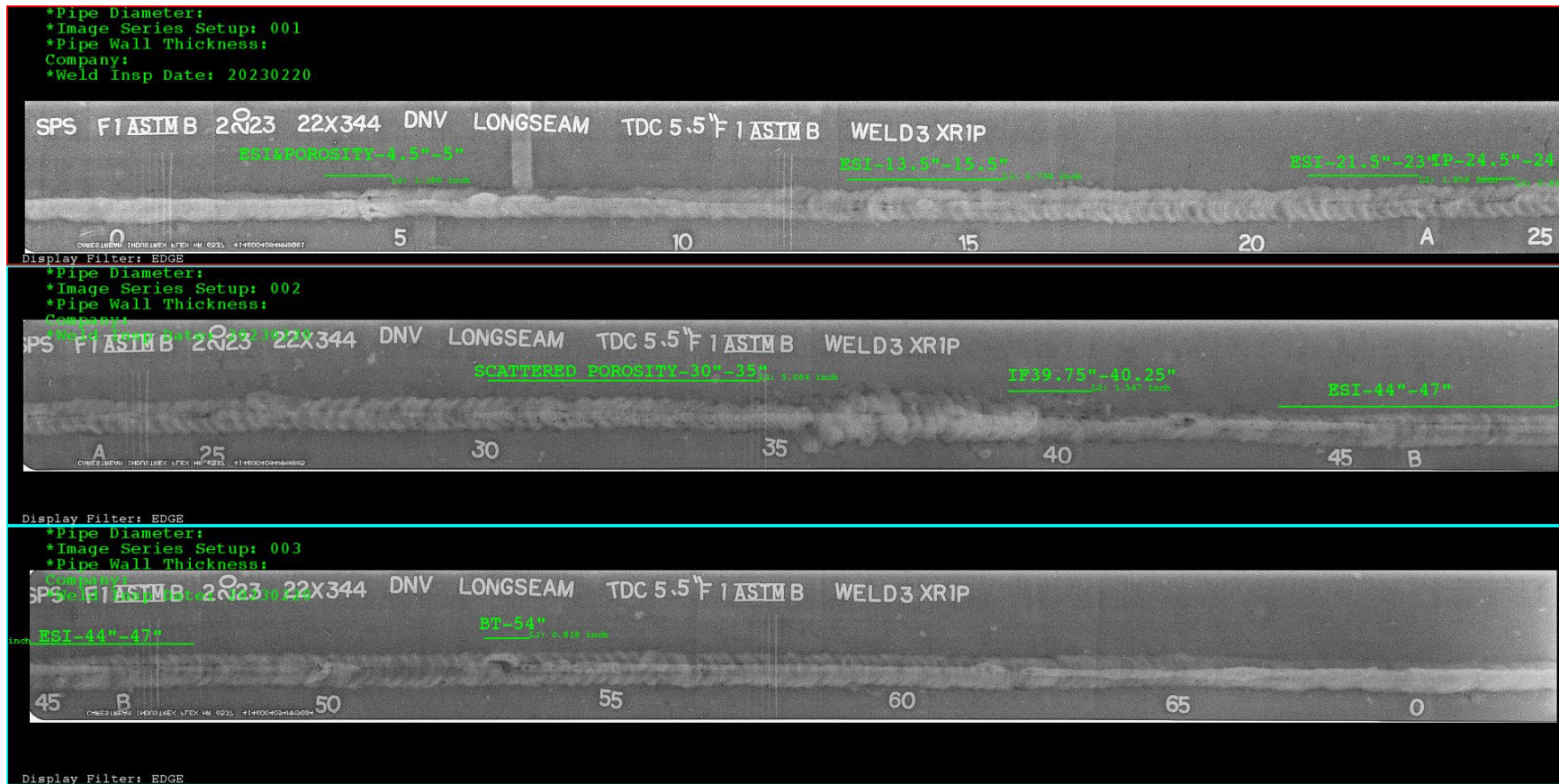
Figure 87. Montage of the radiographs from the girth weld of Pipe 3. The 0 represents 12 o'clock top dead center, with the remaining numbers indicating distances clockwise in inches. The seam welds are visible between the 5 and 10 locations.
