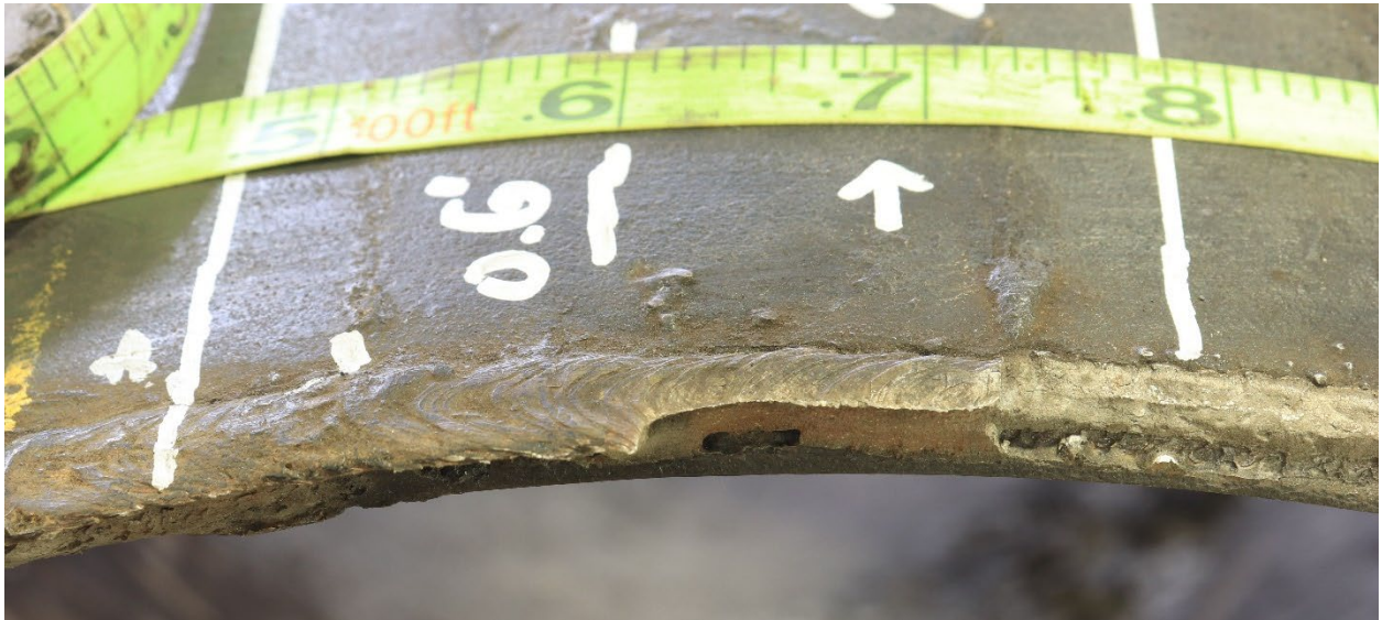
Figure 13. An angled view of an area of the Pipe 1 fracture surface annotated for sectioning.
