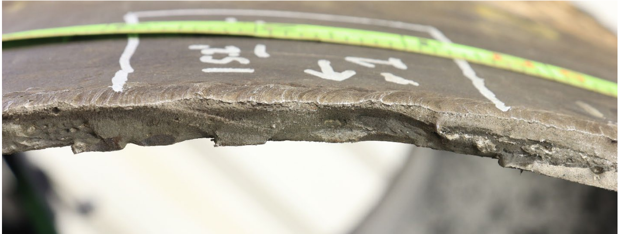
Figure 12. An oblique view of an area of the Pipe 1 fracture surface annotated for sectioning.
