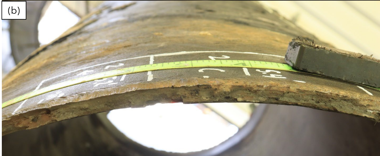
Figure 14. An (a) angled and (b) oblique view of an area of the Pipe 1 fracture surface annotated for sectioning.
