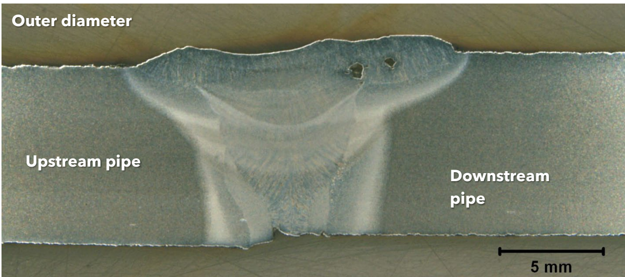
Figure 91. BF optical micrograph of the Pipe 3 girth weld at location M3-2, sectioned 2.08 feet clockwise of top dead center (~5X, etched 2% Nital).
