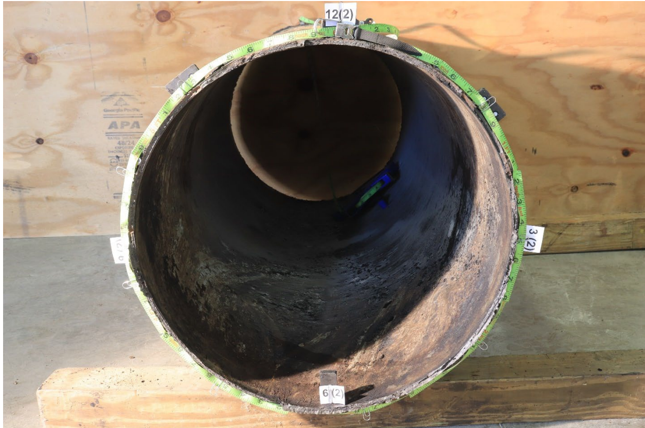
Figure 25. View of the entire fracture surface of Pipe 2 that had mated to that of Pipe 1.
