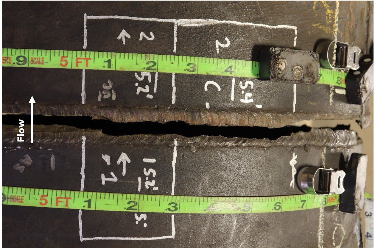
Figure 9. Mating fracture surfaces along the girth weld between Pipes 1 and 2, showing areas to be sectioned.
