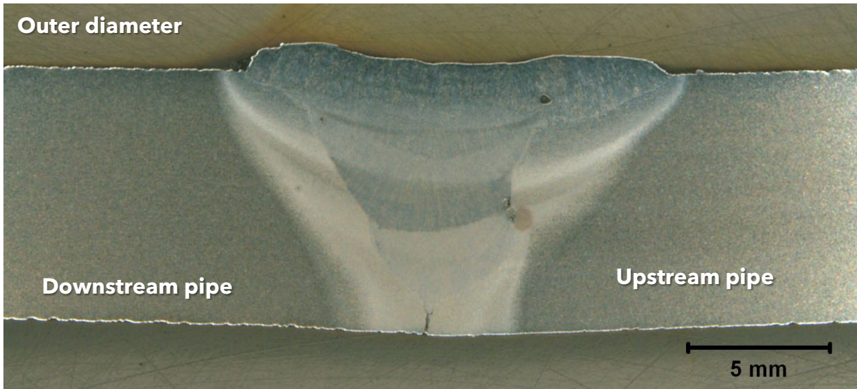
Figure 88. BF optical micrograph of the Pipe 3 girth weld at location M3-1, removed 1.06 clockwise of 12 o'clock top dead center (5X, etched 2% Nital).
