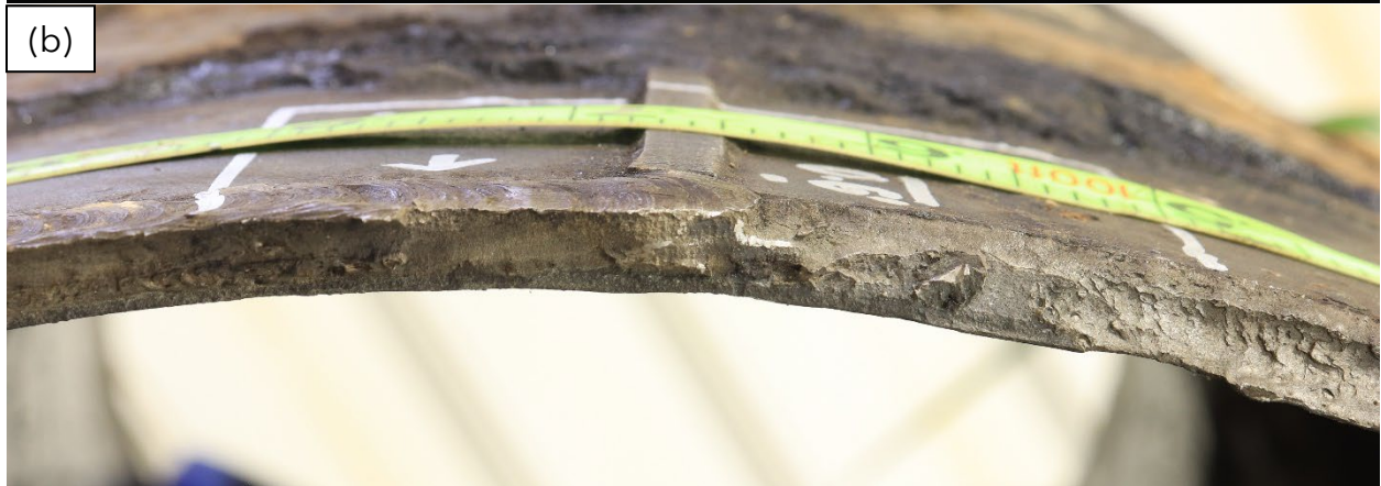
Figure 10. An (a) angled and (b) oblique view of an area of the Pipe 1 fracture surface annotated for sectioning.
