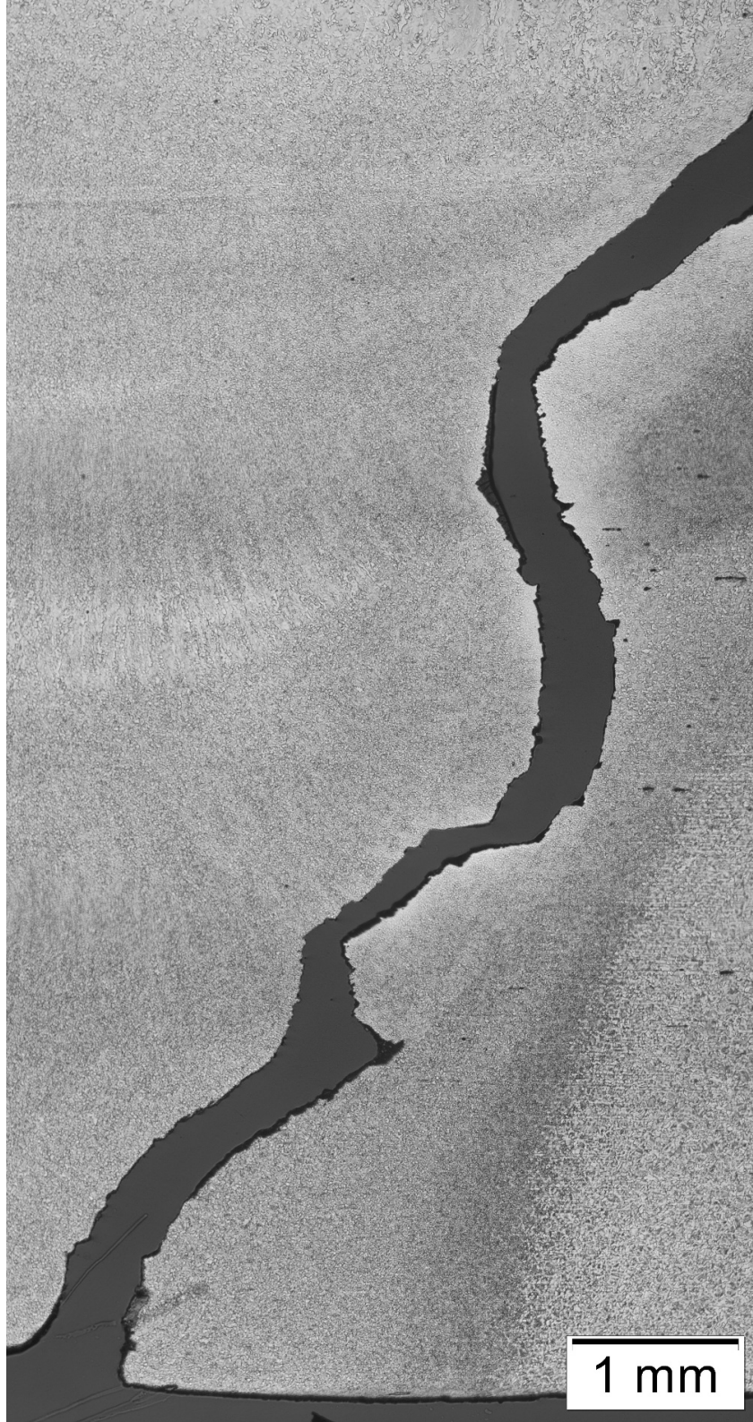
Figure 53. BF optical micrograph montage of the fracture through weld M1_5b (~25X, etched 2% Nital).
