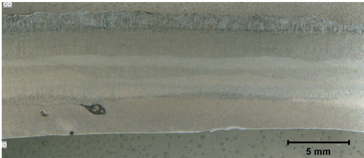
Figure 62. BF optical micrograph of M2C (location in Figure 6), parallel to the girth weld showing the multiple passes along the weld (~5X, etched 2% Nital).
