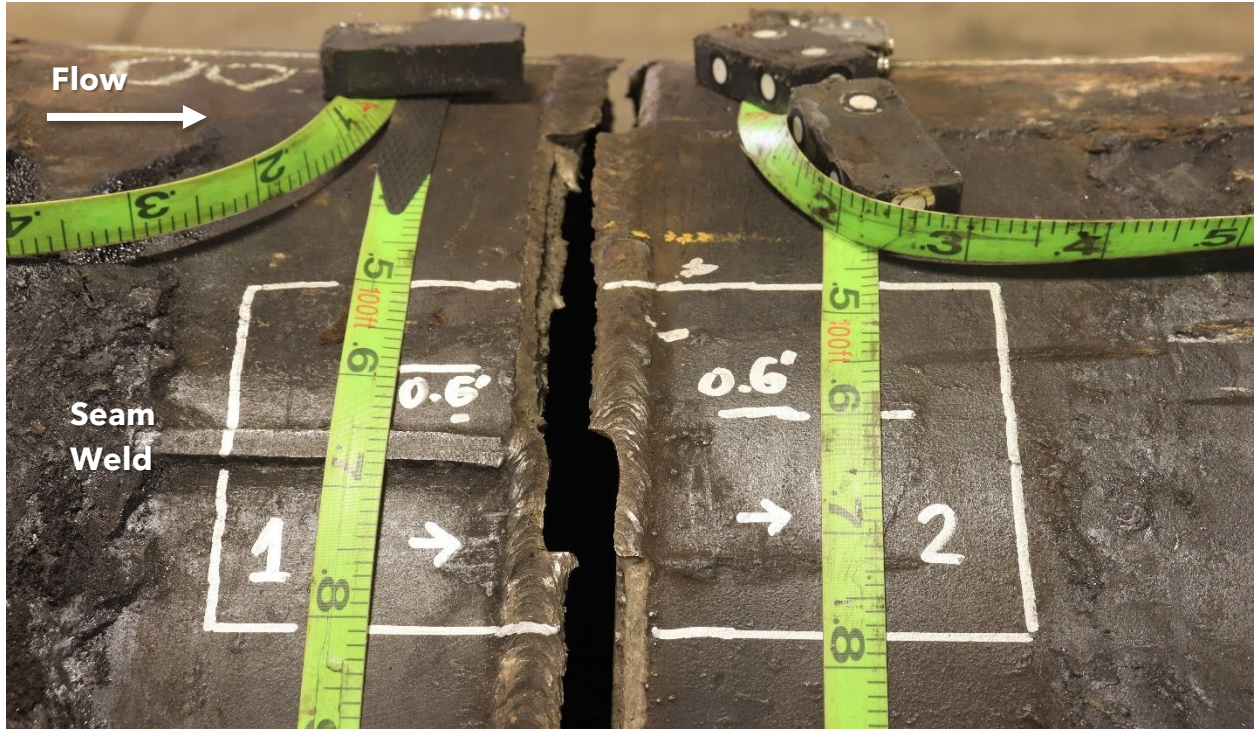
Figure 7. Mating fracture surfaces along the girth weld between Pipes 1 and 2, showing areas to be sectioned.
