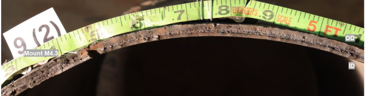
Figure 32. View of the Pipe 2 fracture surface clockwise of the 9 o'clock position, annotated to show the location of one of the metallographic cross section.
