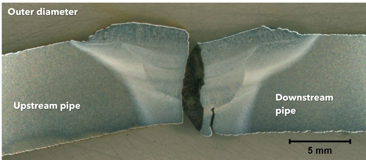
Figure 60. BF optical micrograph of the fracture at the weld at location M5_2, approximately 5.29 feet counterclockwise of top dead center (5X, etched 2% Nital).
