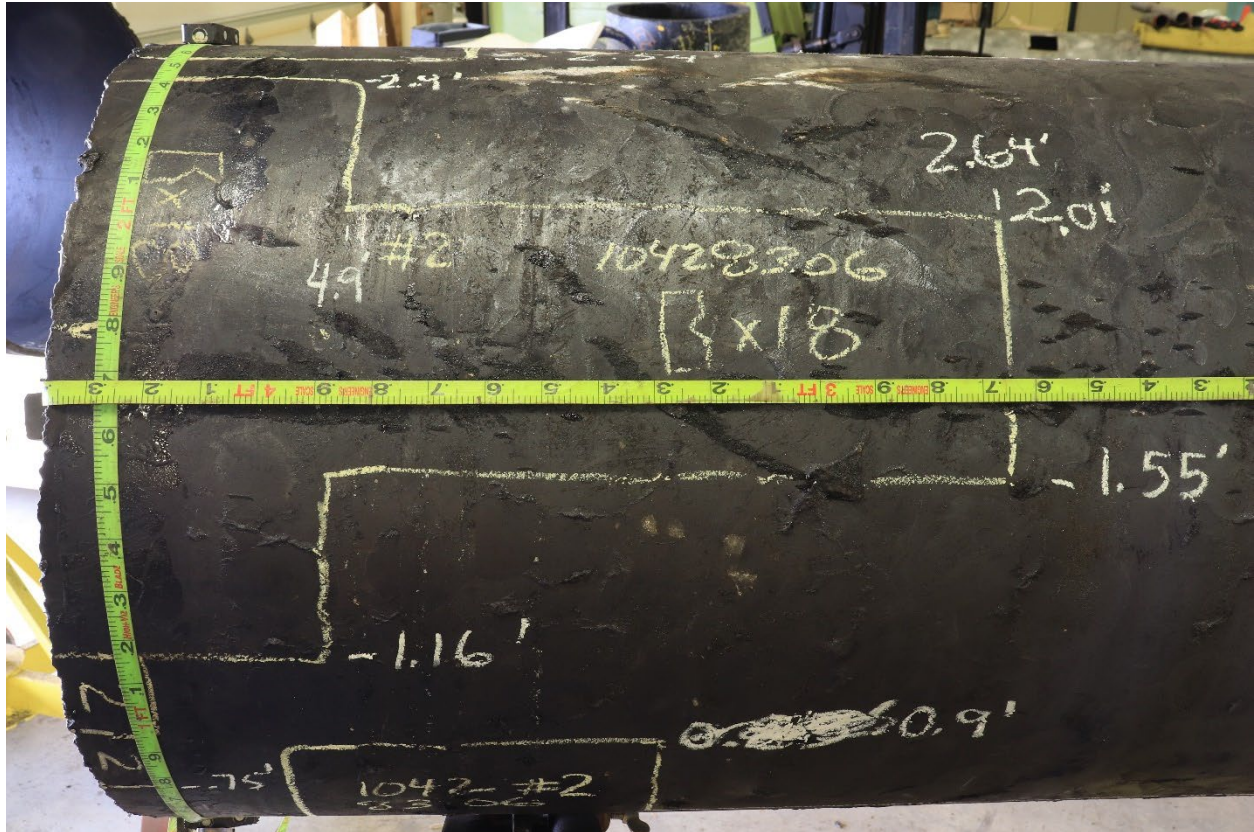
Figure 23. View of the outer surface of Pipe 1, showing areas annotated for extracting impact specimens, their numbers, and orientations.
