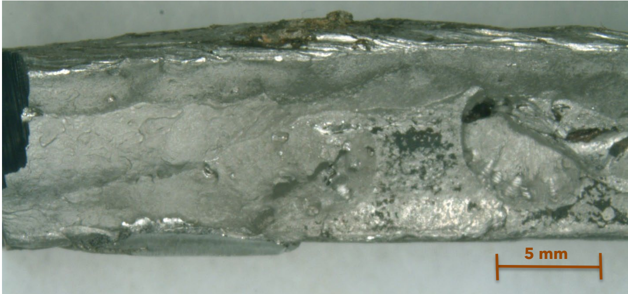
Figure 70. Closer view of the left edge of the Pipe 2 fracture surface section at 1:15 o clock position, shown in Figure 69.
