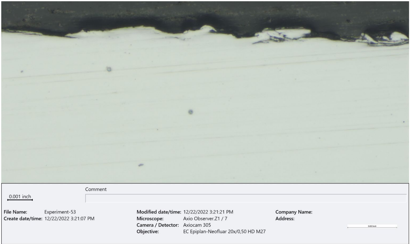
Figure 35. BF optical micrograph of fretting wear in the outboard axle areas (~500X, as polished).
