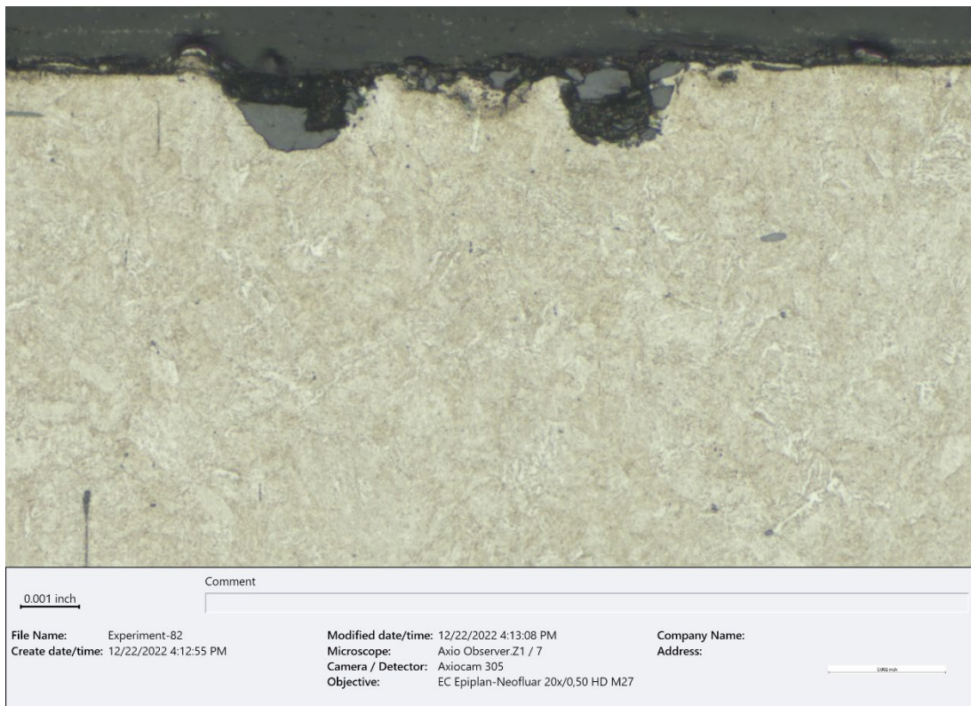
Figure 30. BF optical micrograph of embedded particles in B (~500X, etched 2% Nital).
