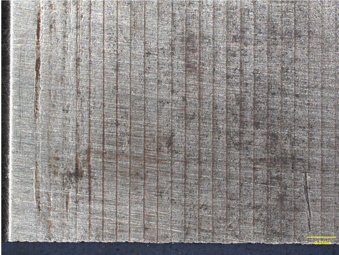
Figure 10. View on the inboard corner of Area A, showing brinelling of the surface from the wheel bore.
