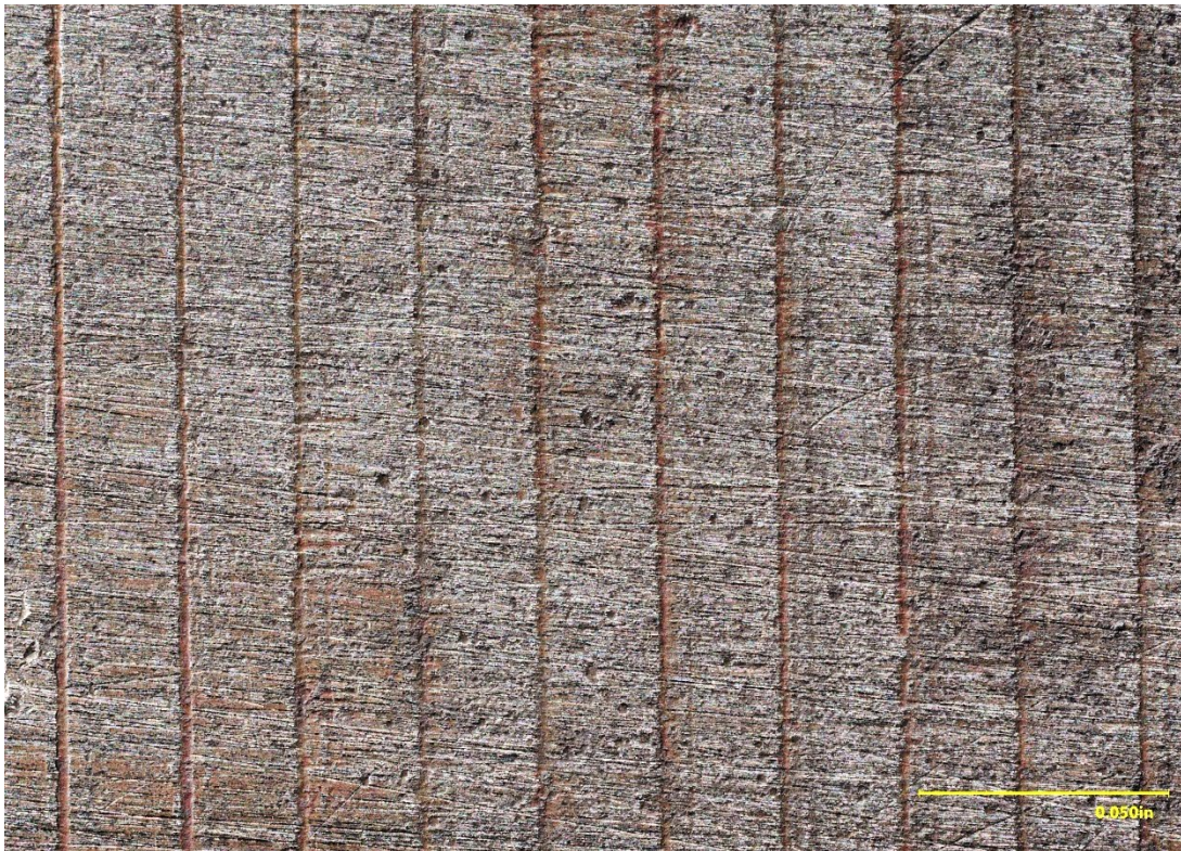
Figure 12. Closer view of the brinelling marks in Figure 11 .
