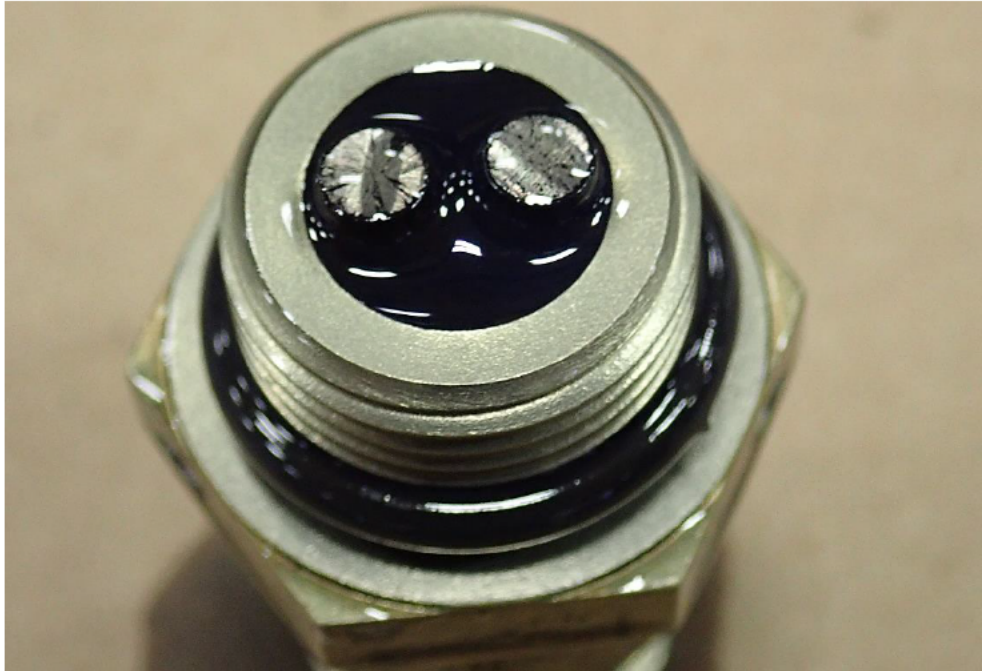
Photo No. 26, view of the accessory gearbox chip detector
