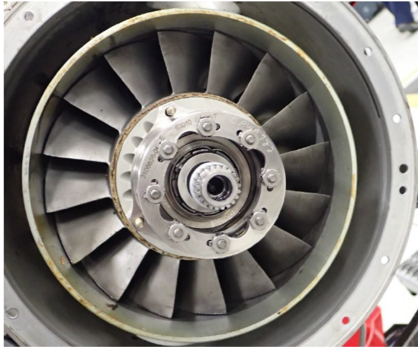
Photo No. 38, view of the No. 1 bearing
