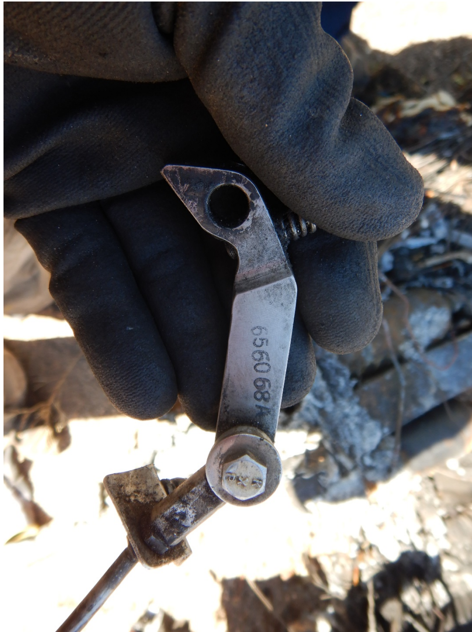
Photo 34 - Supplied close-up view of the throttle linkage.
