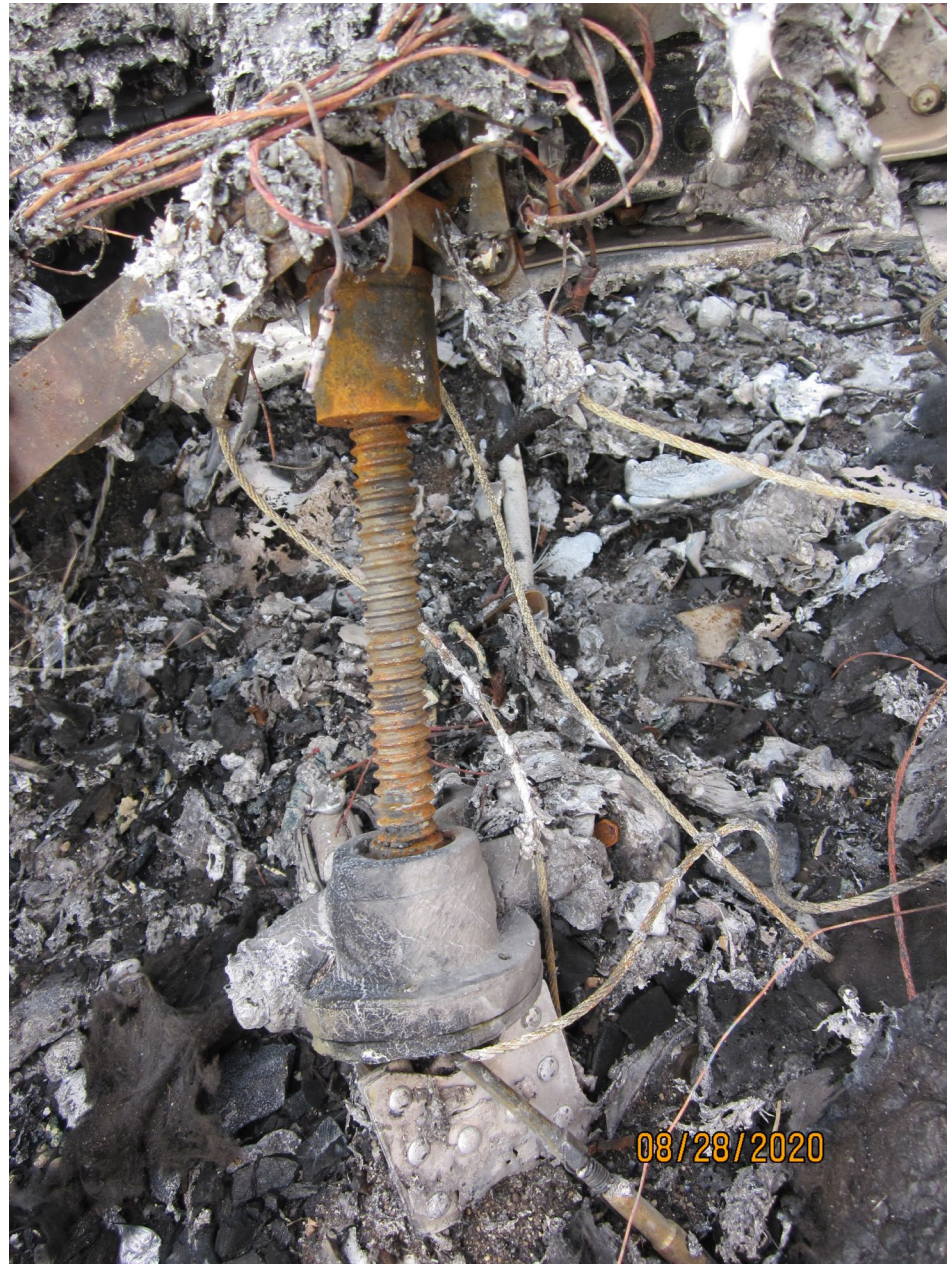
Photo 9 - Supplied photo of the flap jackscrew.
