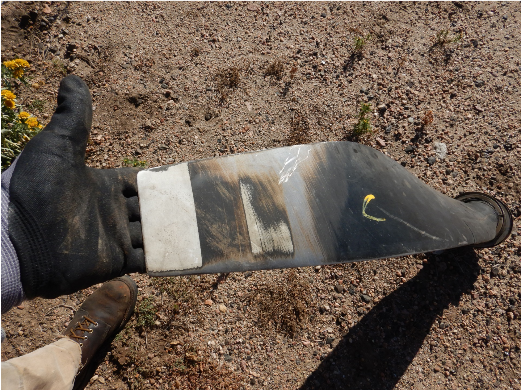
Photo 19 - Supplied close-up photo of a propeller blade. The blade exhibits chordwise abrasion.
