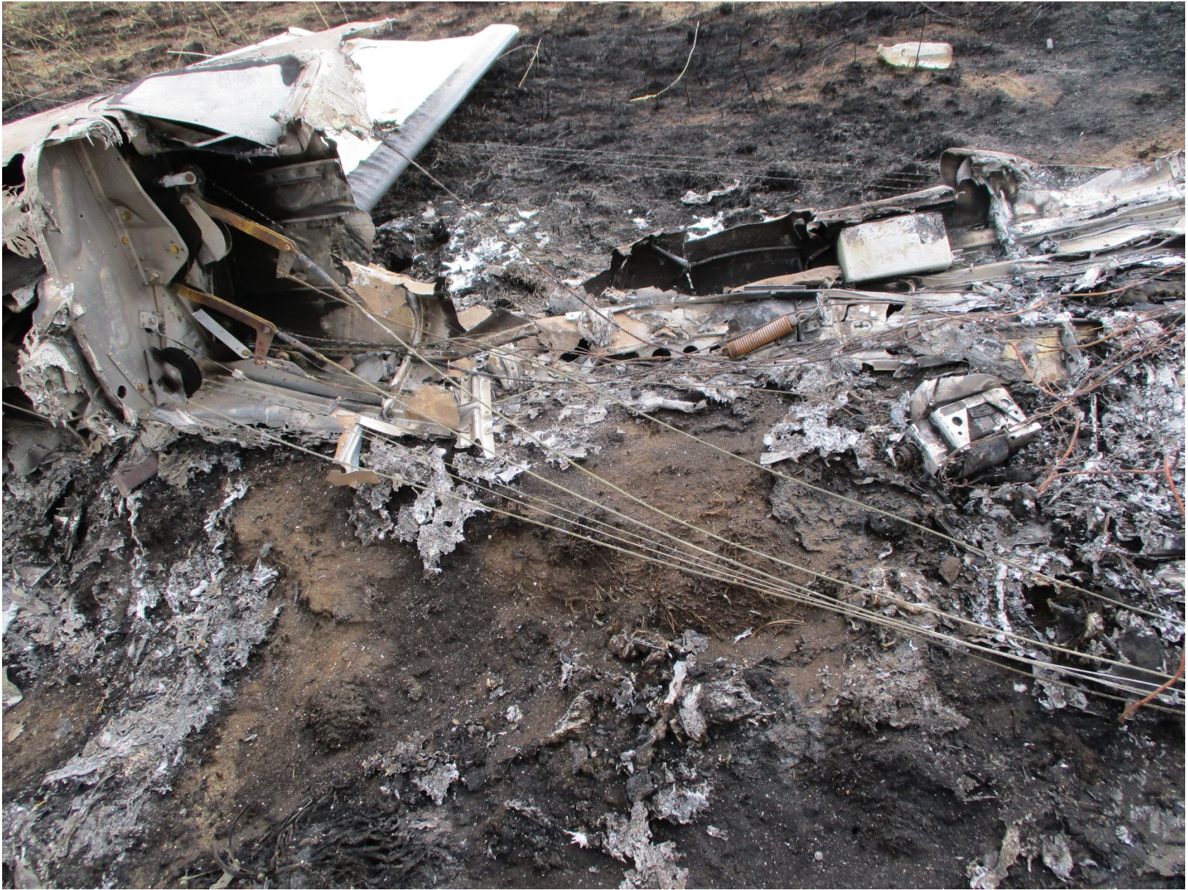
Photo 16 - Supplied photo of flight control cables near the empennage.
