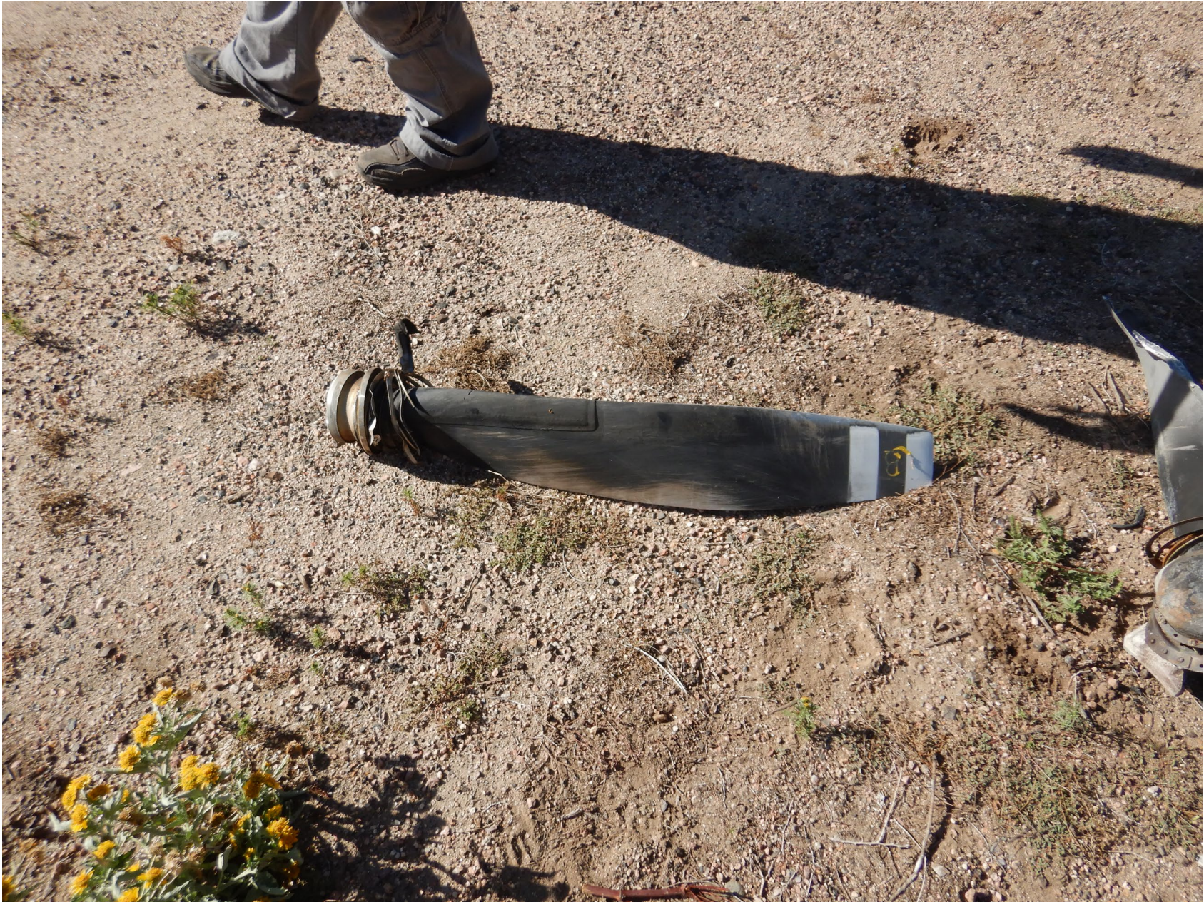
Photo 18 - Supplied photo of a propeller blade. The blade exhibits leading edge abrasion.
