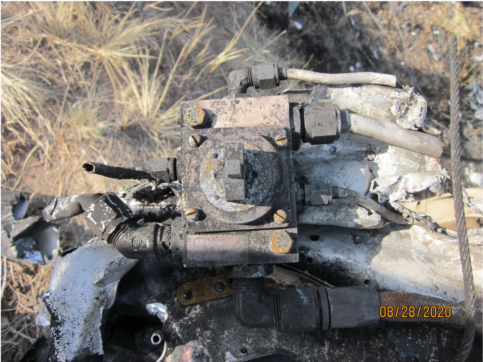
Photo 11 - Supplied photo of the fuel tank selector valve.
