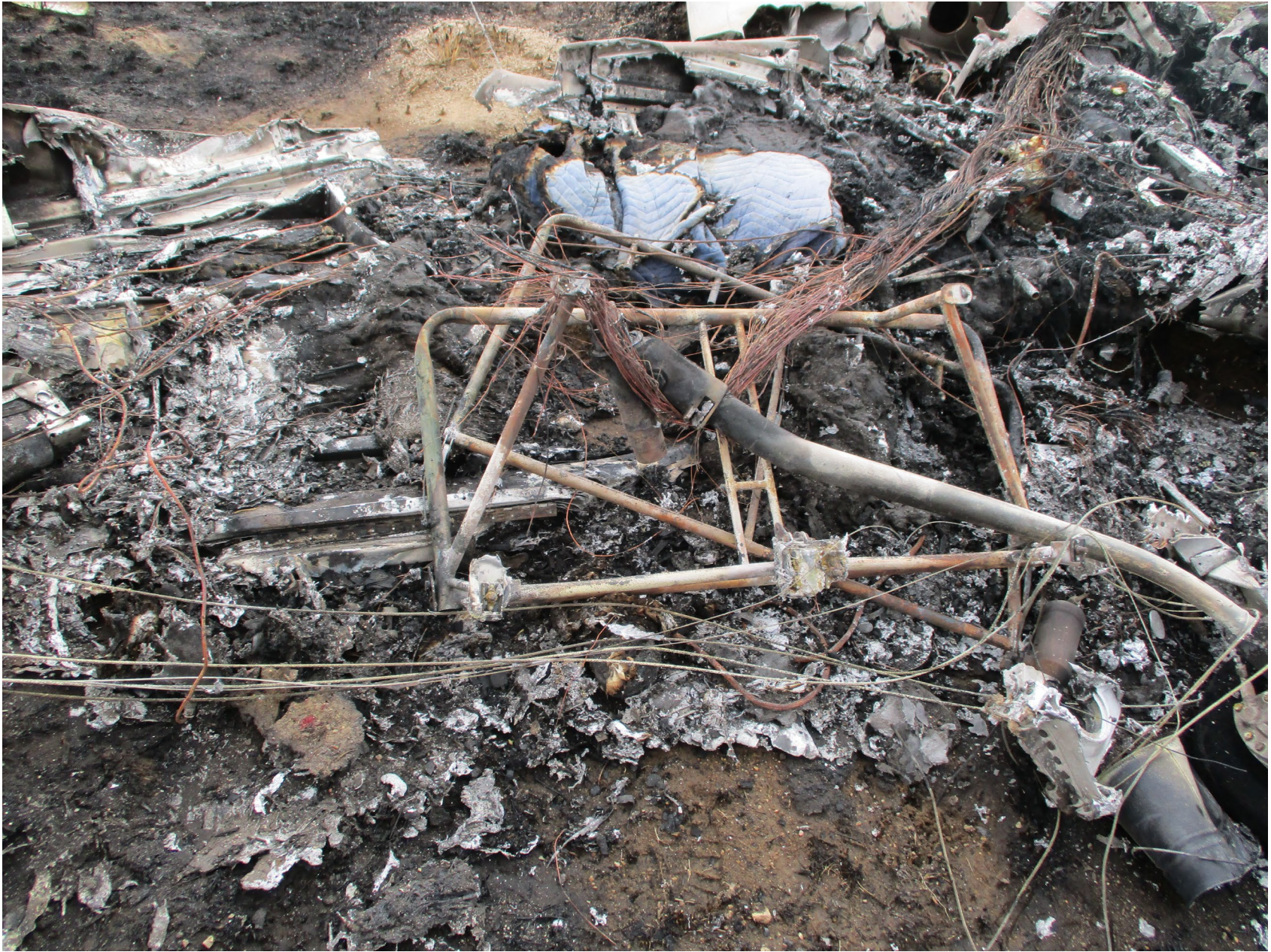
Photo 15 - Supplied photo of flight control cables.
