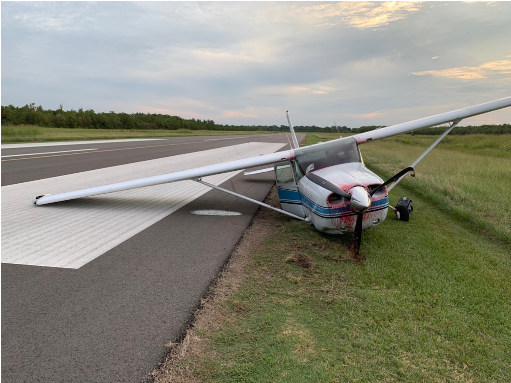
Photo 1 – Supplied photo of the front of the airplane with its nose and right landing gear collapsed.
