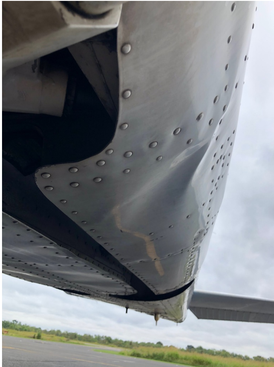
Photo 6 - Supplied photo of the airplane fuselage showing skin deformation around the left main landing gear.
