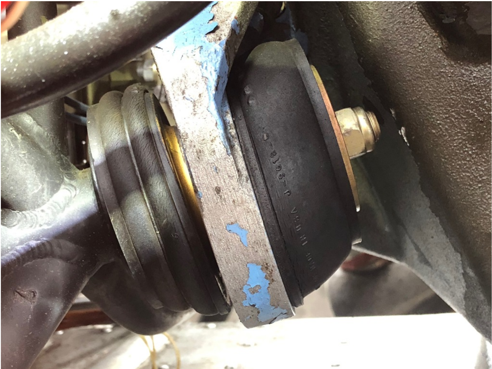
Photo 8 - Supplied photo of the engine mount showing displaced vibration isolation material.
