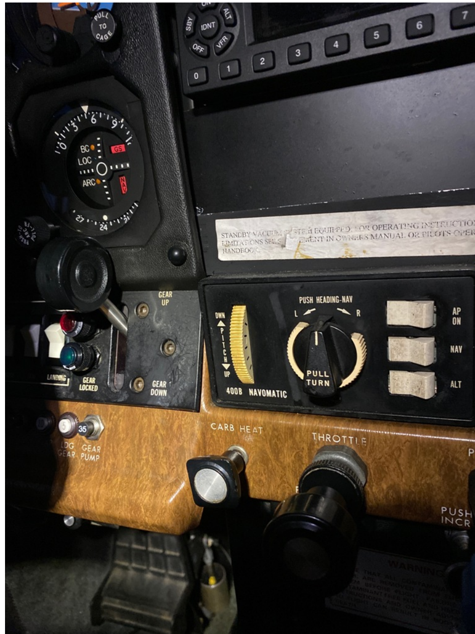
Photo 3 - Supplied photo of the instrument panel with the landing gear handle in the up position.
