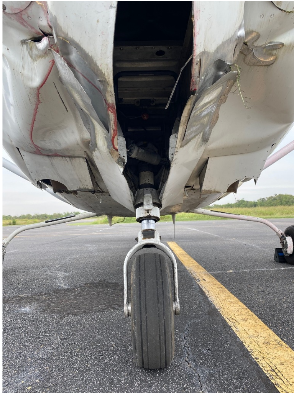
Photo 5 - Supplied photo of the airplane cowling showing skin deformation around the nose landing gear.
