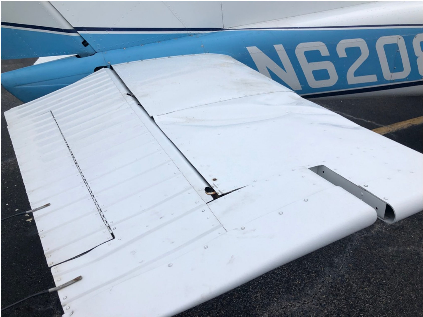
Photo 9 - Supplied photo of the right elevator showing upper skin deformation,
