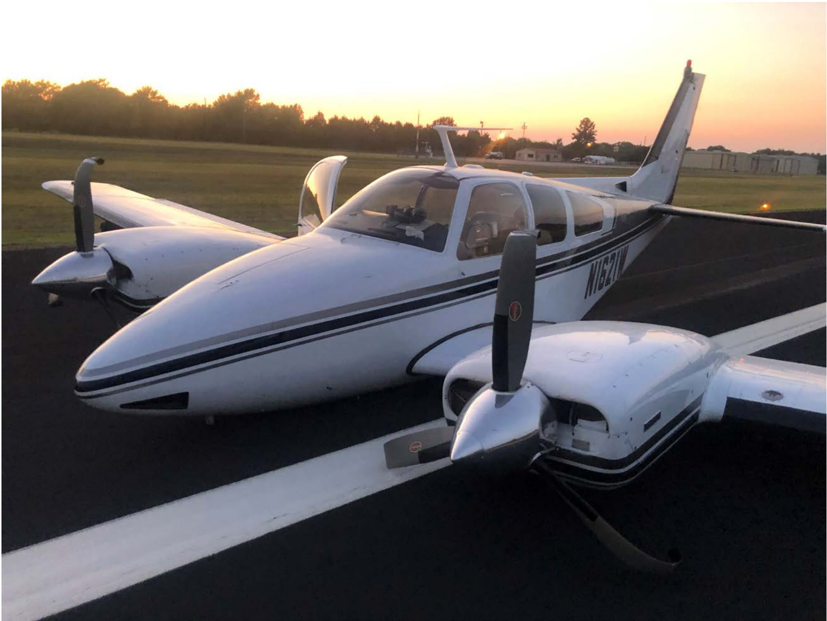
Photo 1 – Supplied view of the accident airplane on a runway. The landing gear are not extended and the propellers exhibit tip damage.
