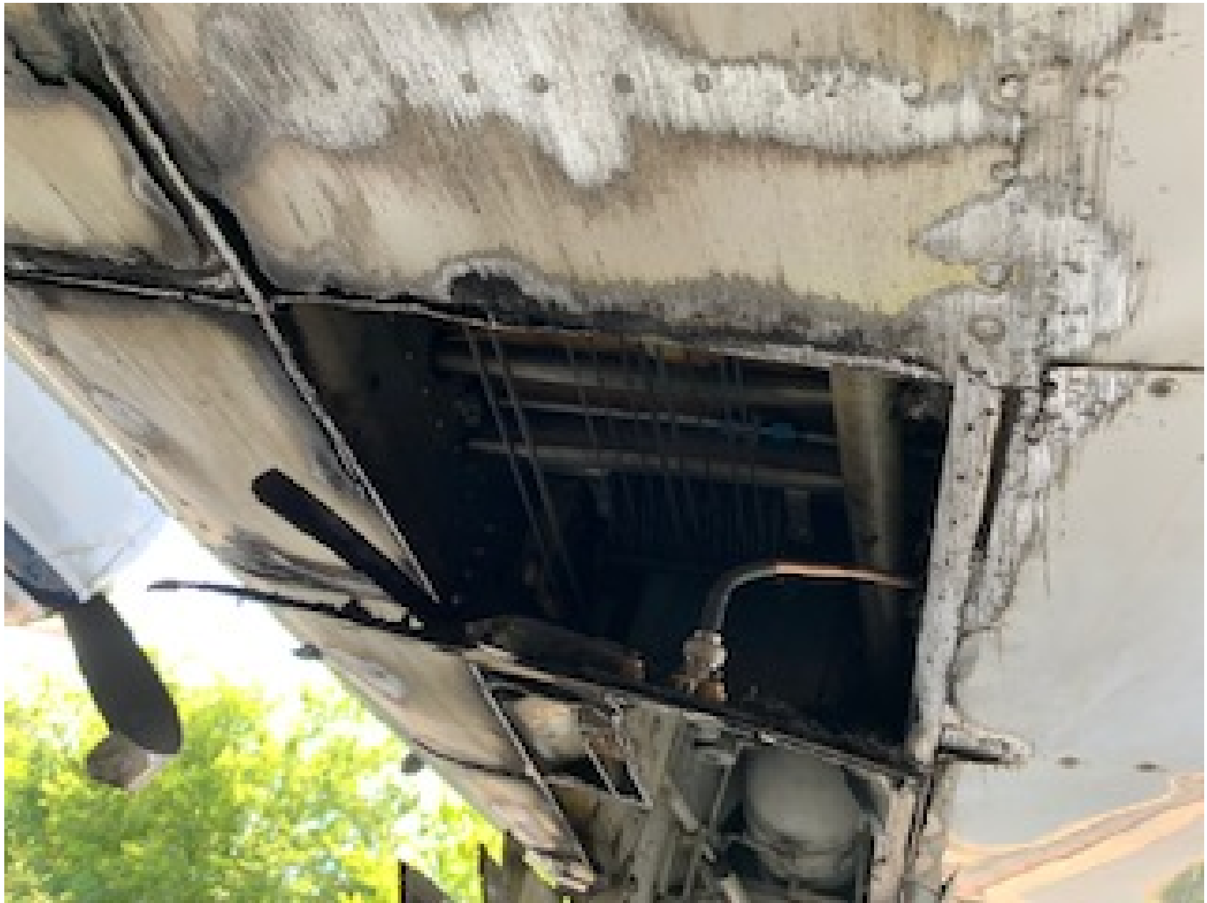
Photo 2 - Supplied view of the fuselage belly. A skin panel is detached from its damaged ribs and stringers.
