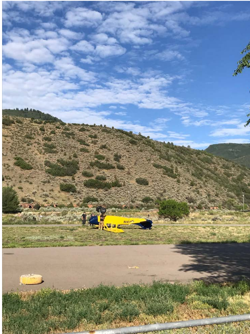
Photo 1 – Supplied photo of the inverted airplane. The airplane exhibits empennage and fuselage deformation.
