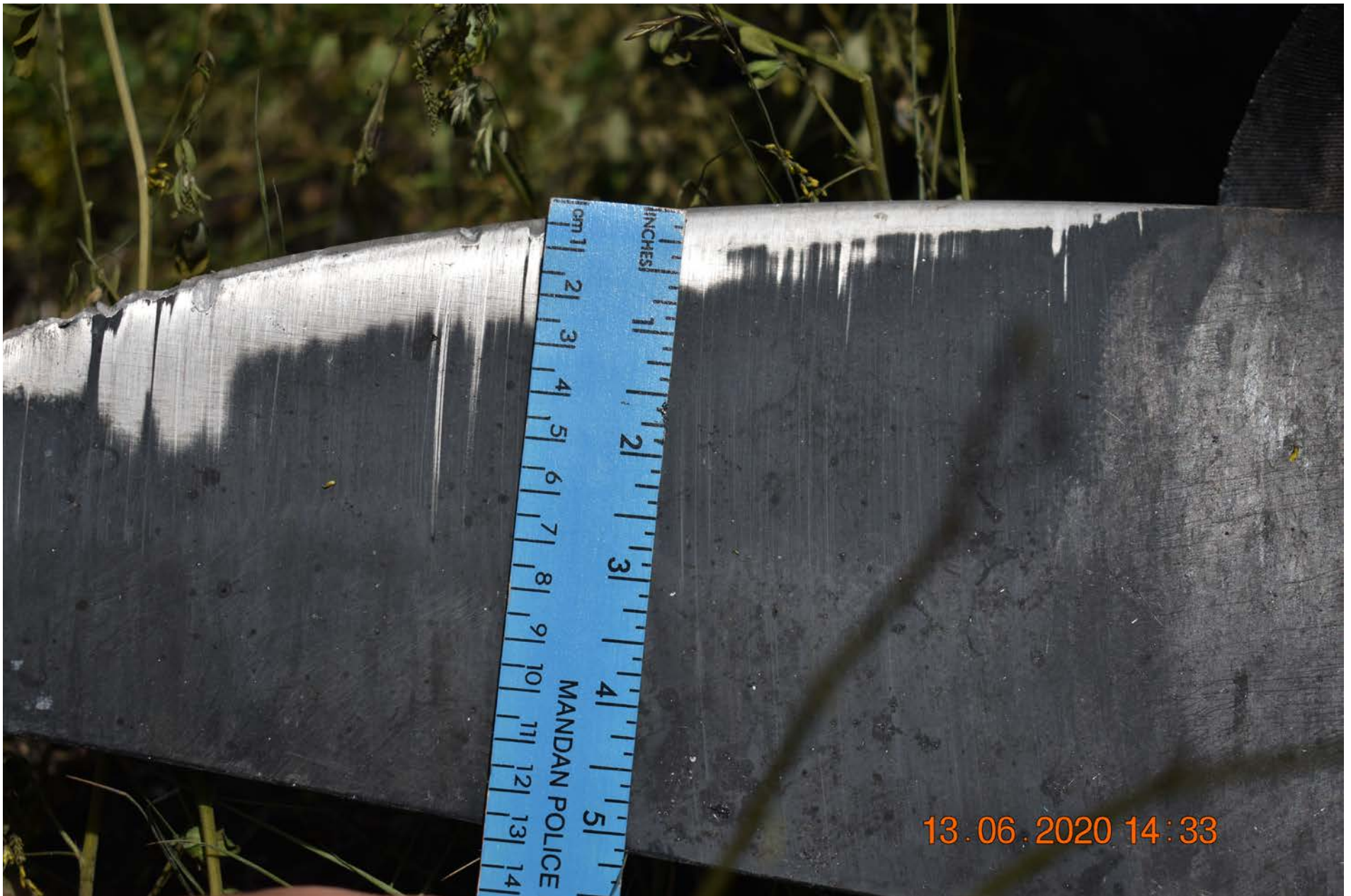
Photo 6 - Supplied photo of a propeller blade exhibiting chordwise abrasion.
