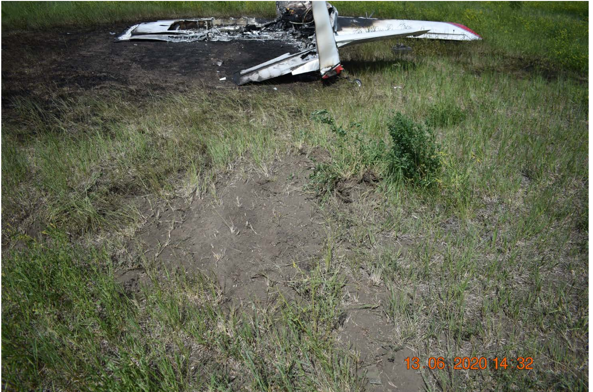
Photo 4 - Supplied photo of the rear of the airplane wreckage in the background and a ground scar in the foreground.
