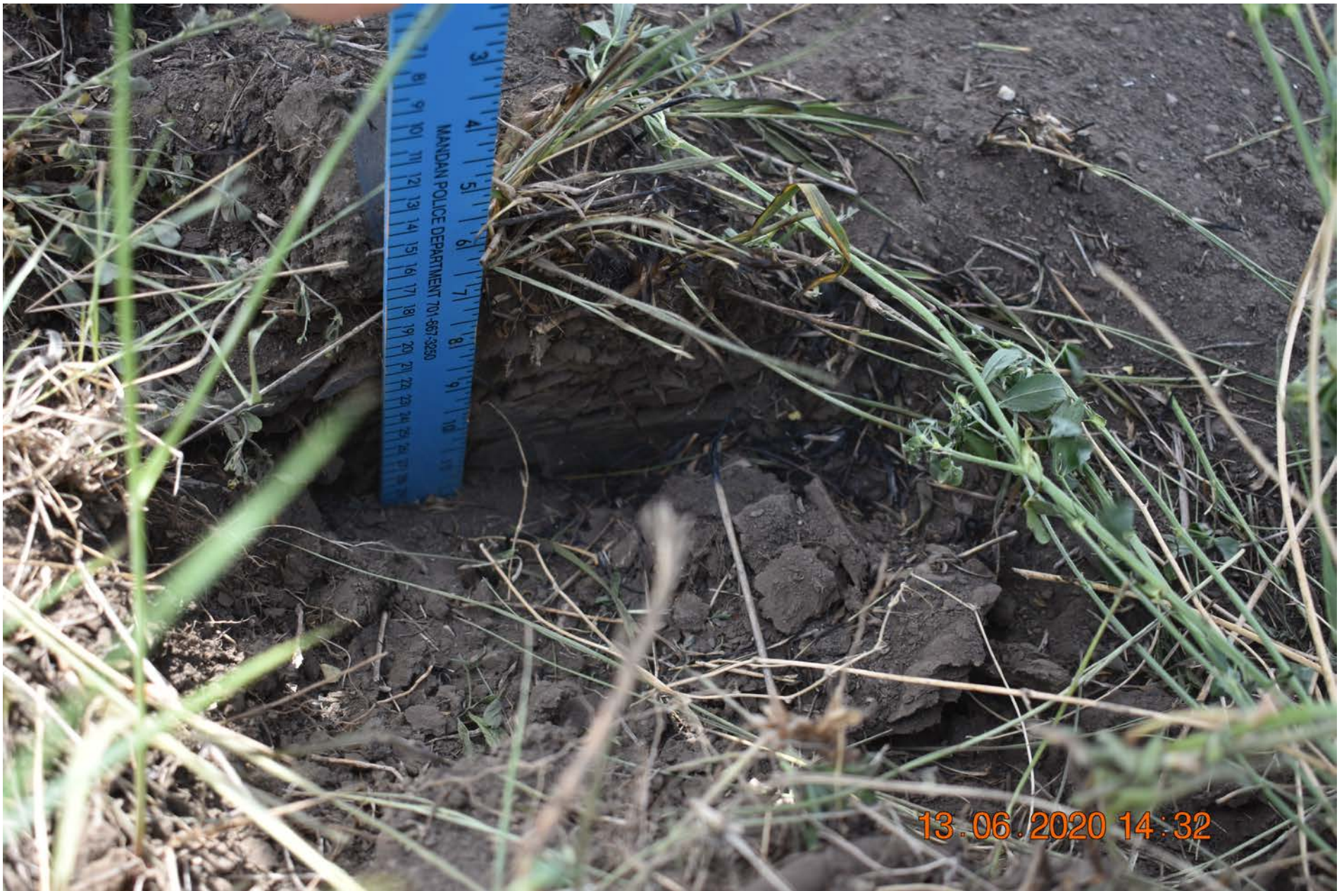
Photo 5 - Supplied photo of a linear ground scar about 6 inches deep.
