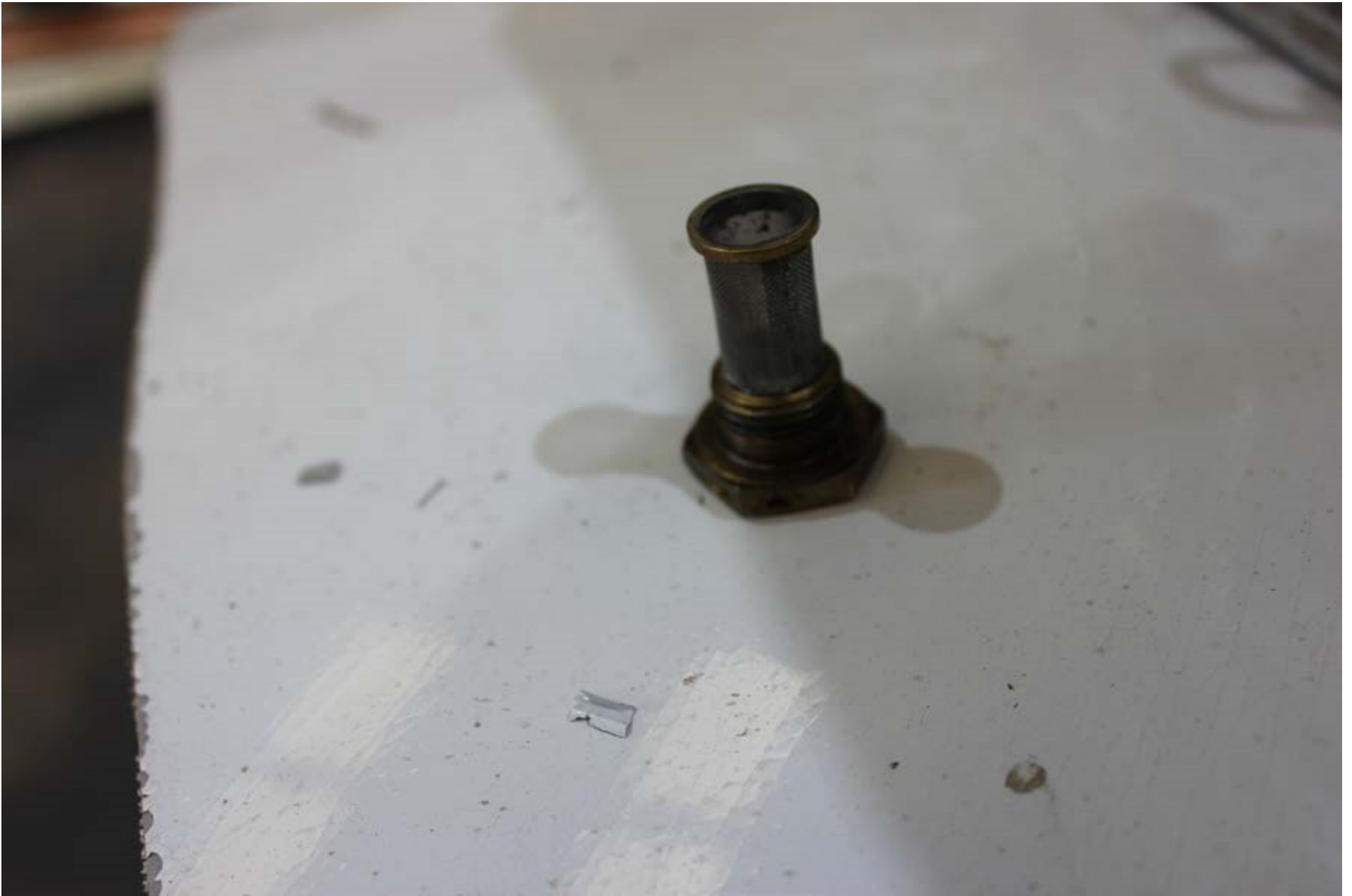
Photo 6 - Supplied close-up photo of the fuel filter screen.
