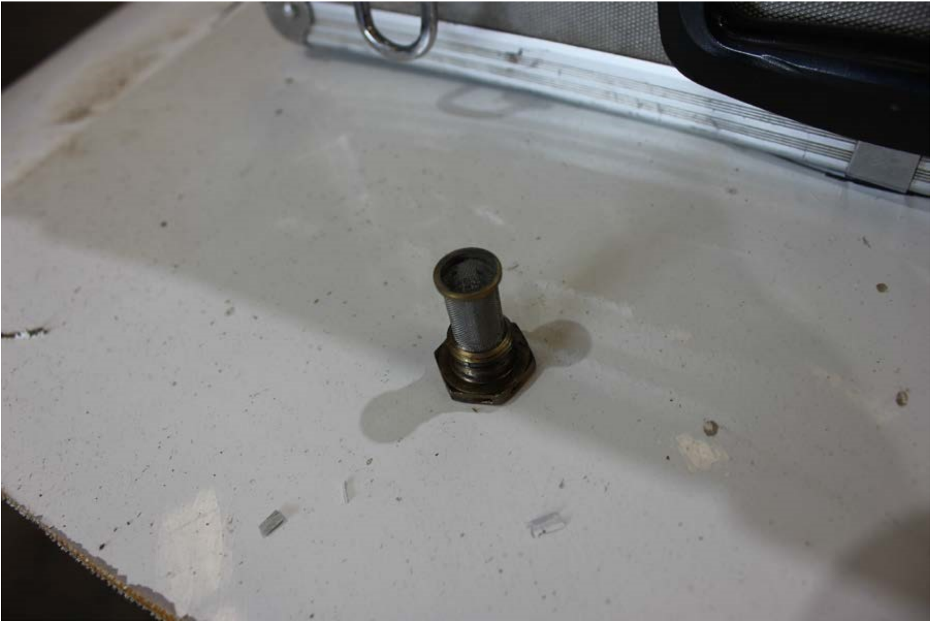
Photo 5 - Supplied photo of the fuel filter screen.
