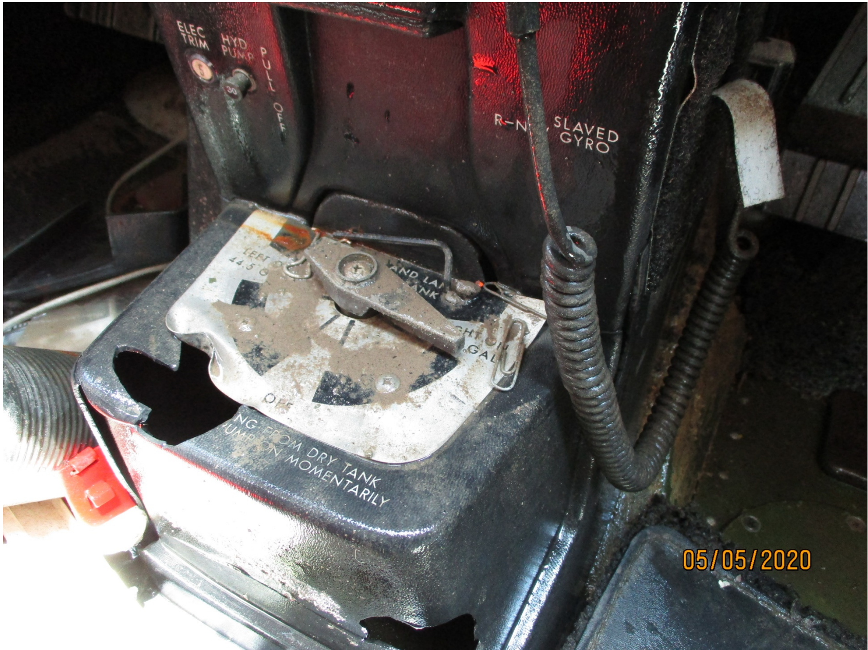
Photo 4 - Supplied close-up photo of the fuel tank selector.
