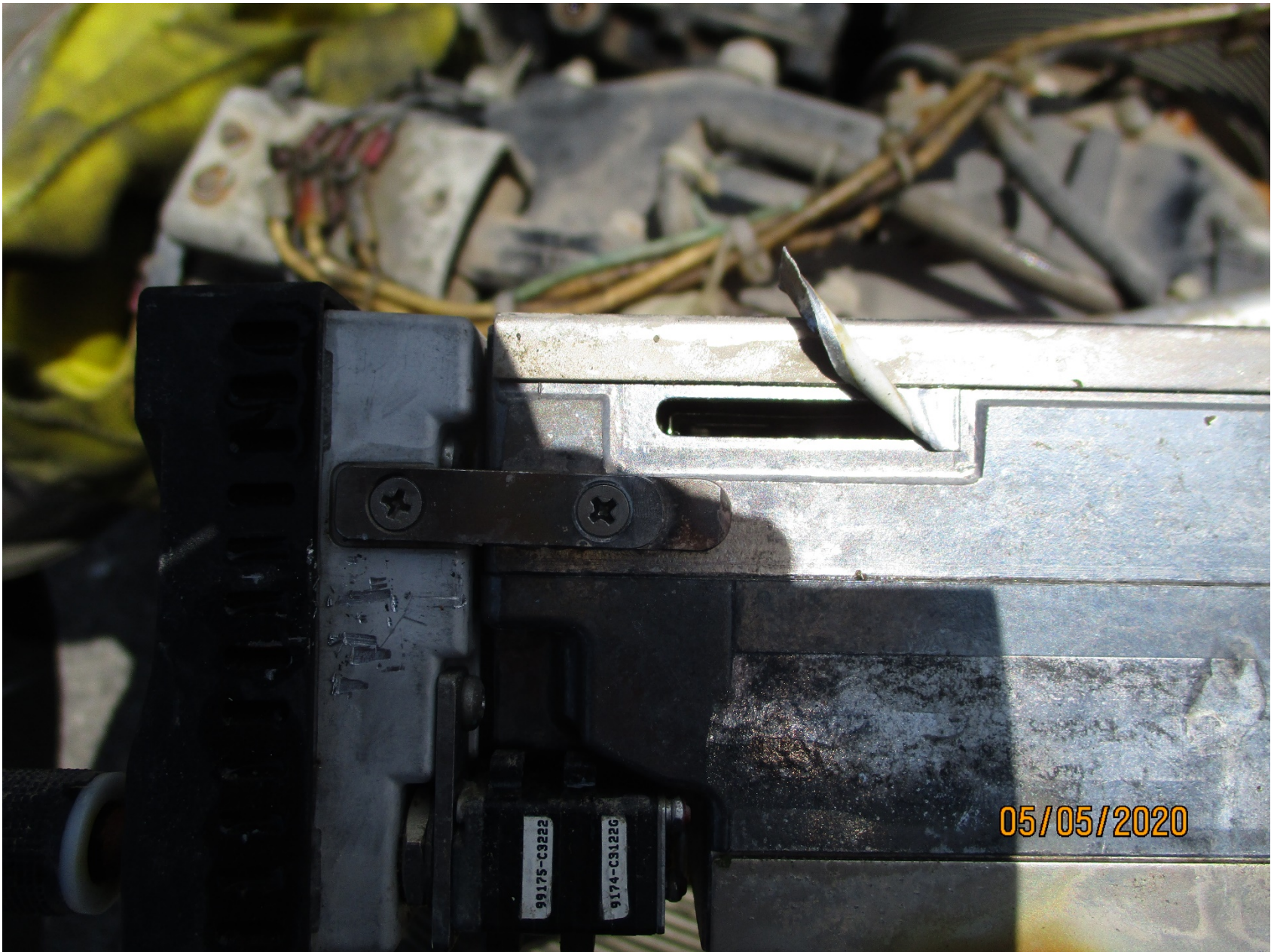
Photo 12 - Supplied close-up photo the removed Garmin GTN 650 unit. A secure data card was removed from the uncovered slot.
