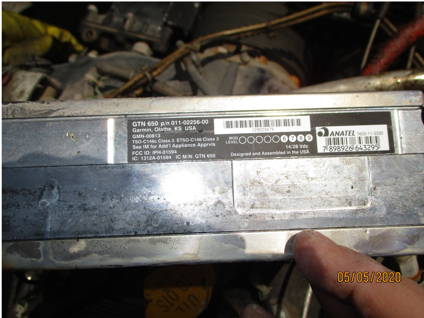
Photo 11 - Supplied close-up photo the removed Garmin GTN 650 unit.
