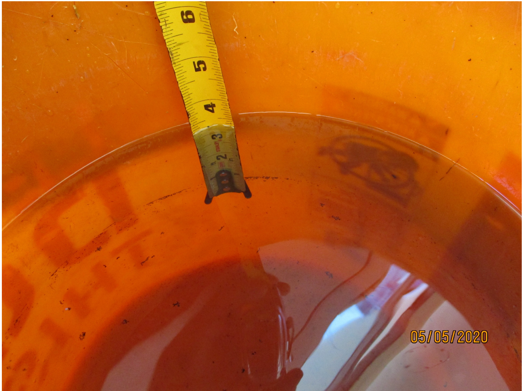
Photo 9 - Supplied close-up photo of liquid recovered from a fuel tank.
