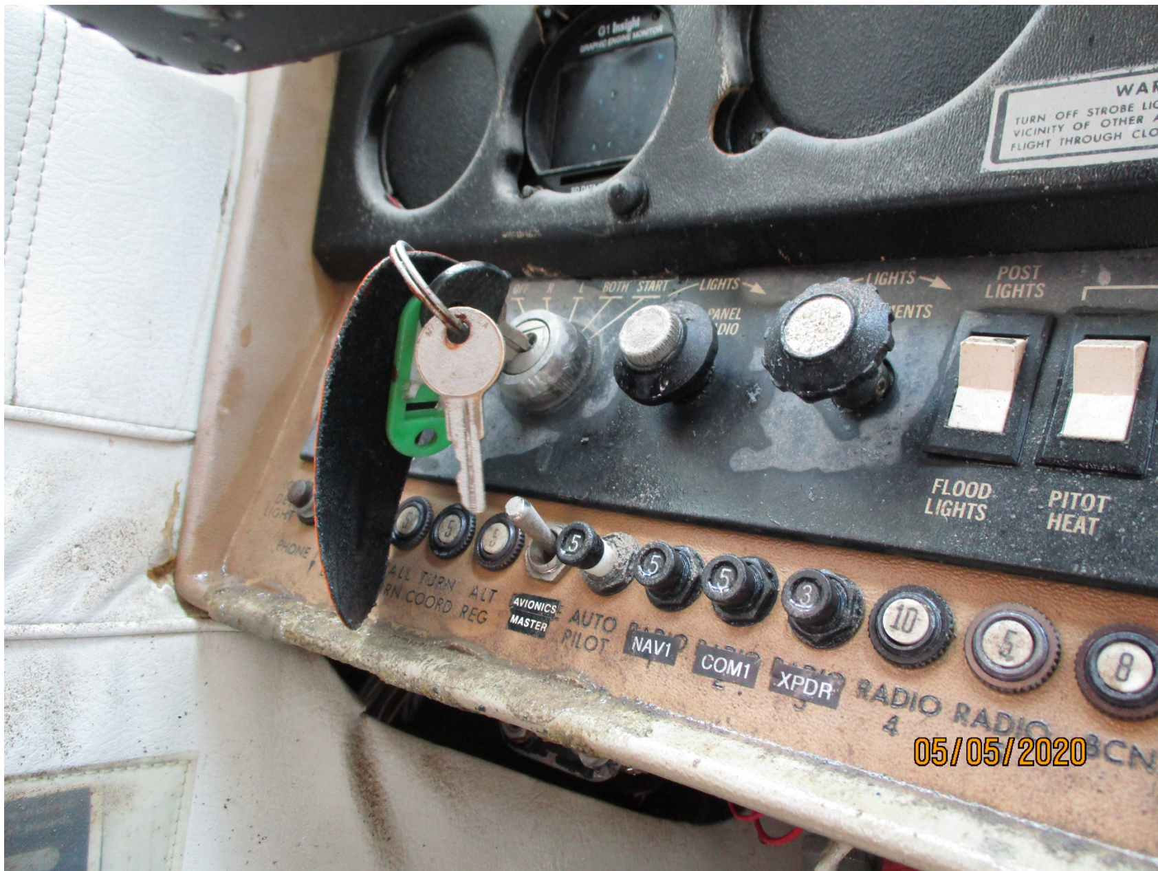
Photo 5 - Supplied close-up photo of the ignition switch.
