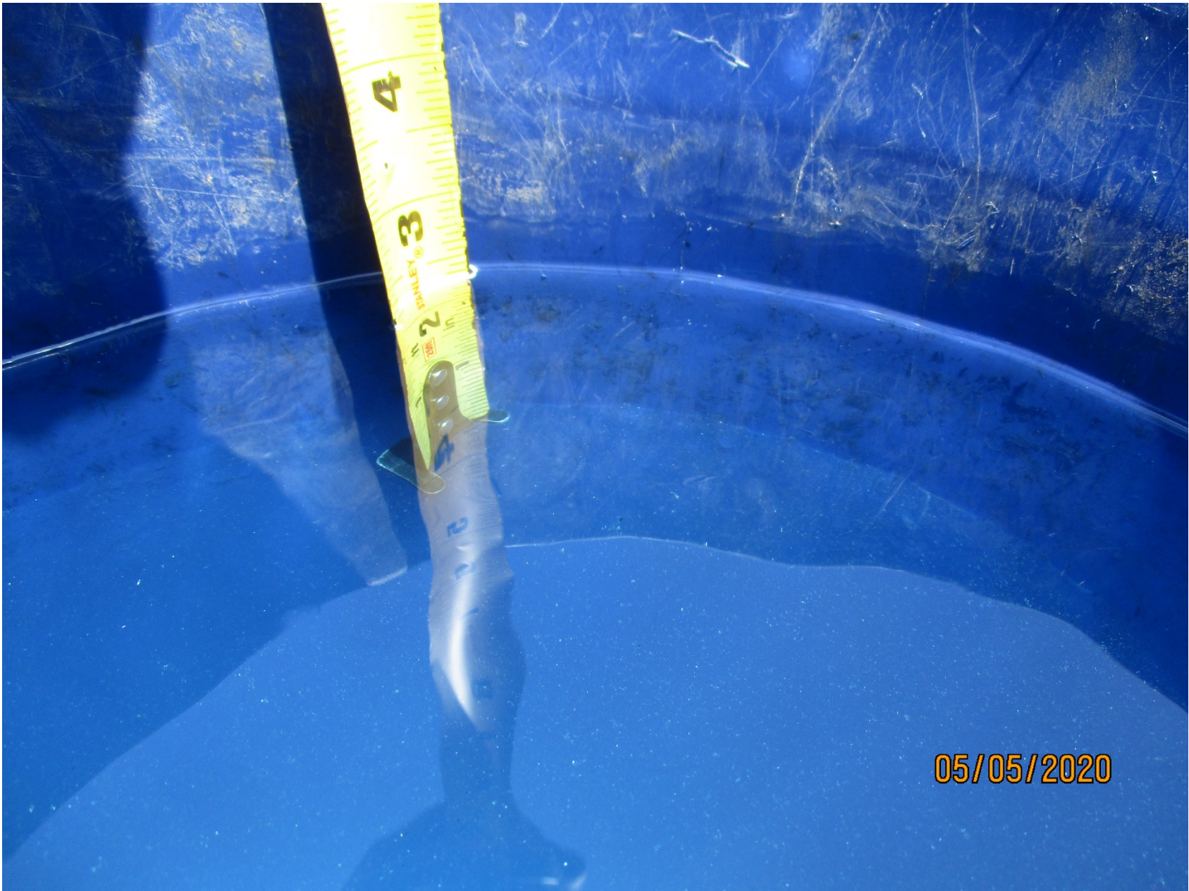
Photo 8 - Supplied close-up photo of liquid recovered from a fuel tank.
