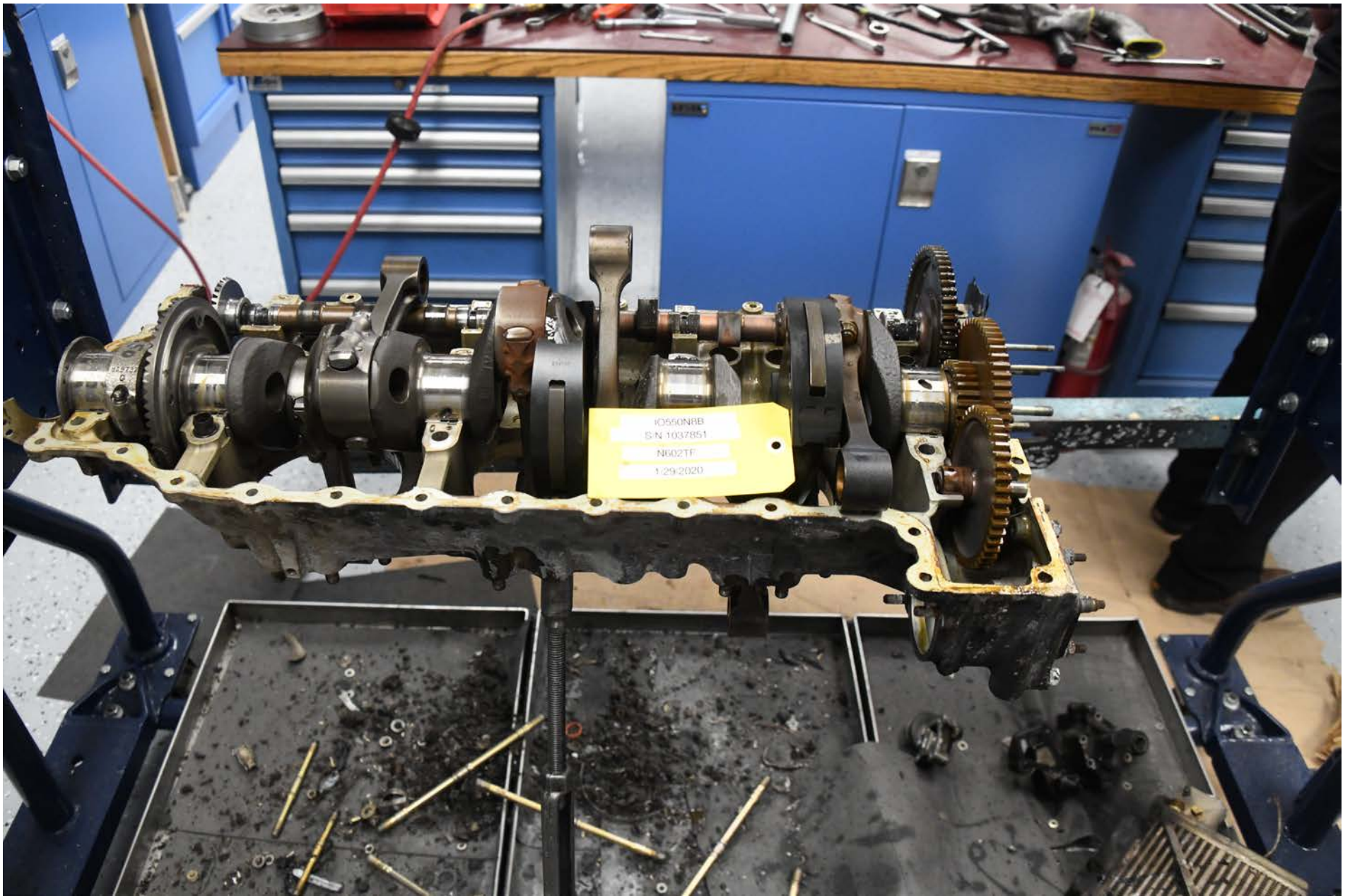
Photo 31 - View inside the crankcase. The crankshaft and connecting rods are present.
