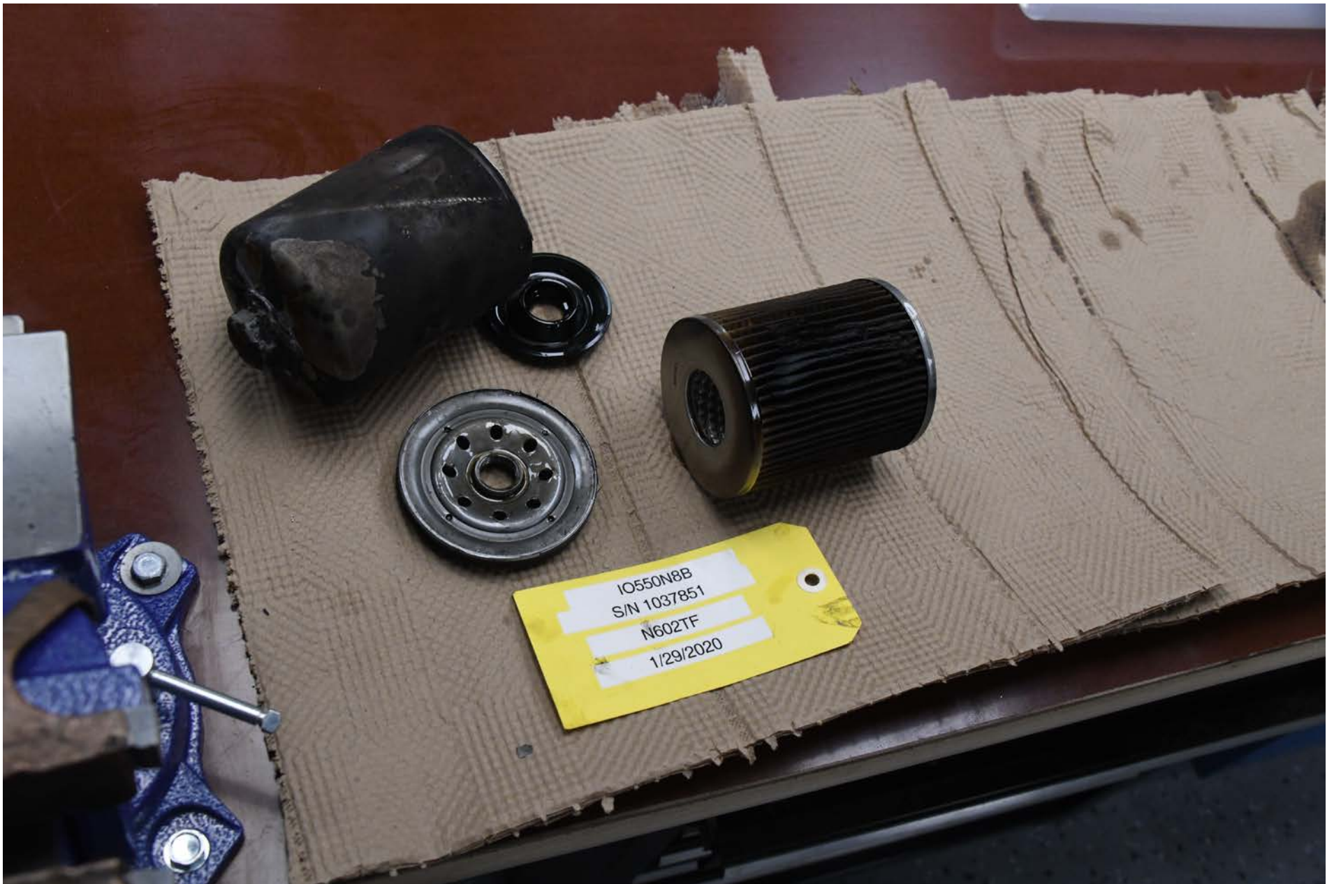
Photo 37 - View of the disassembled engine oil filter.
