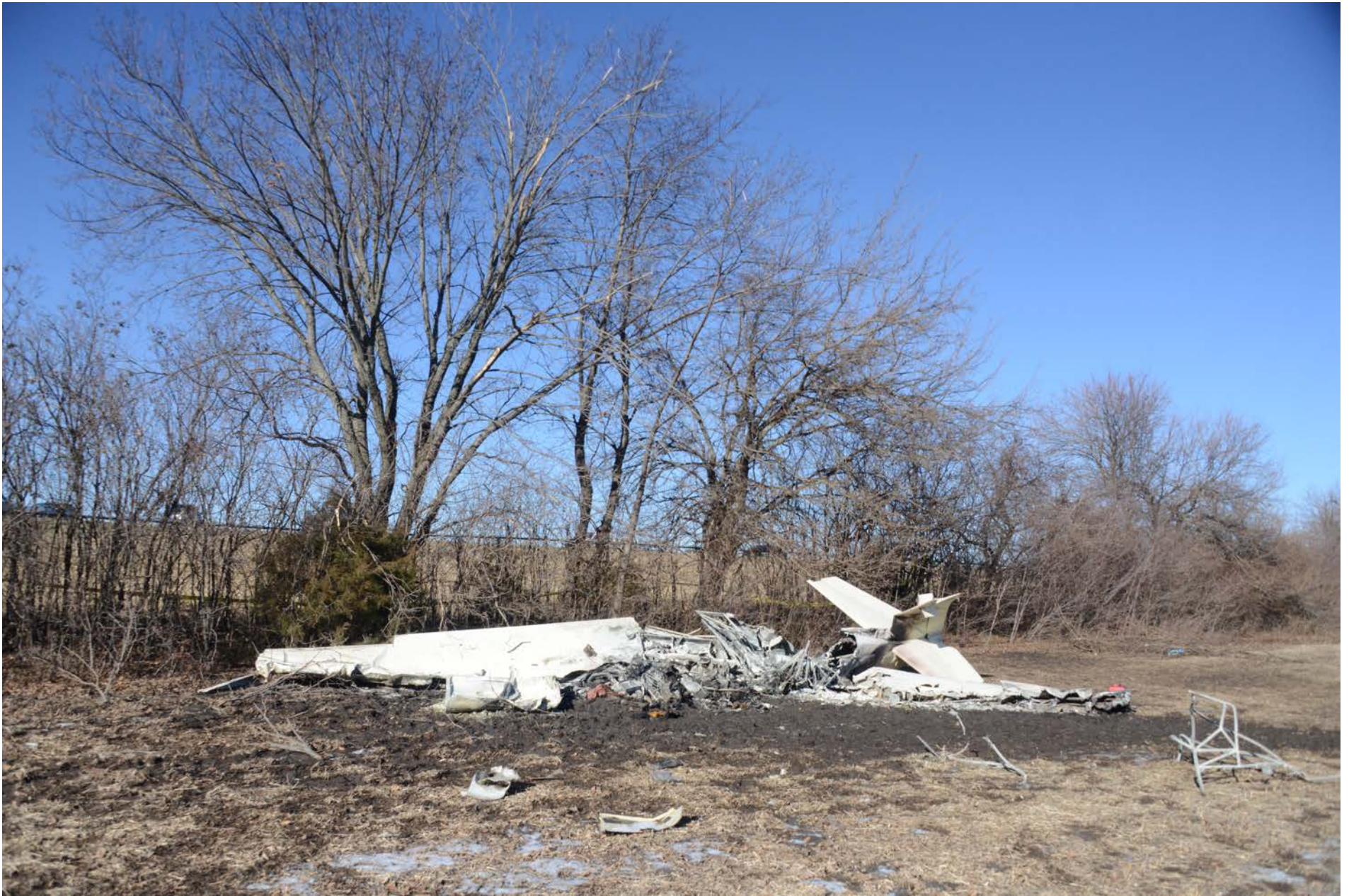
Photo 3 - View of the front side of the airplane at the accident site. Broken branches are present on the tree in the background.
