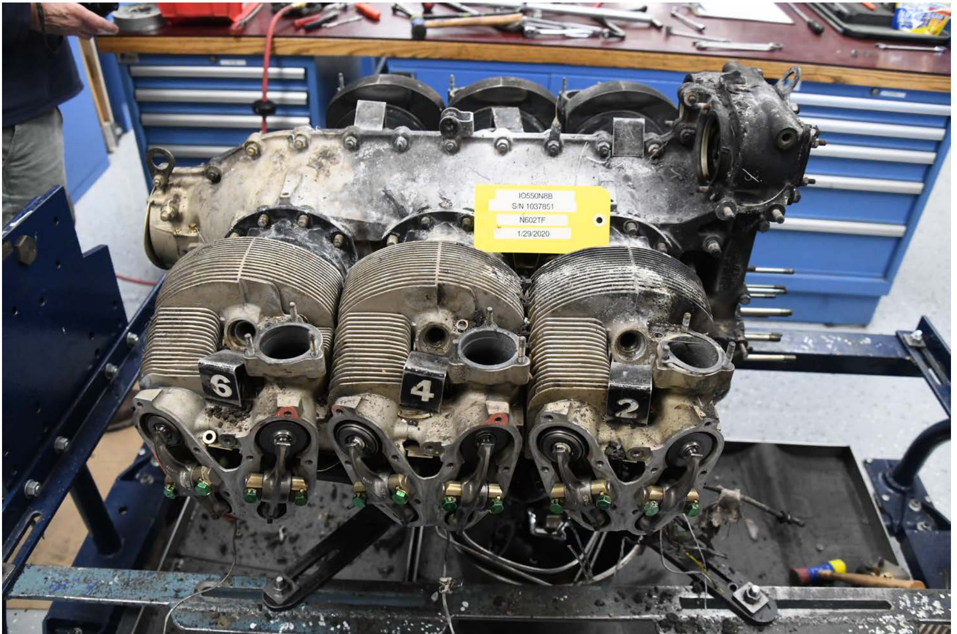
Photo 24 - Close up view of the even bank of engine cylinders.
