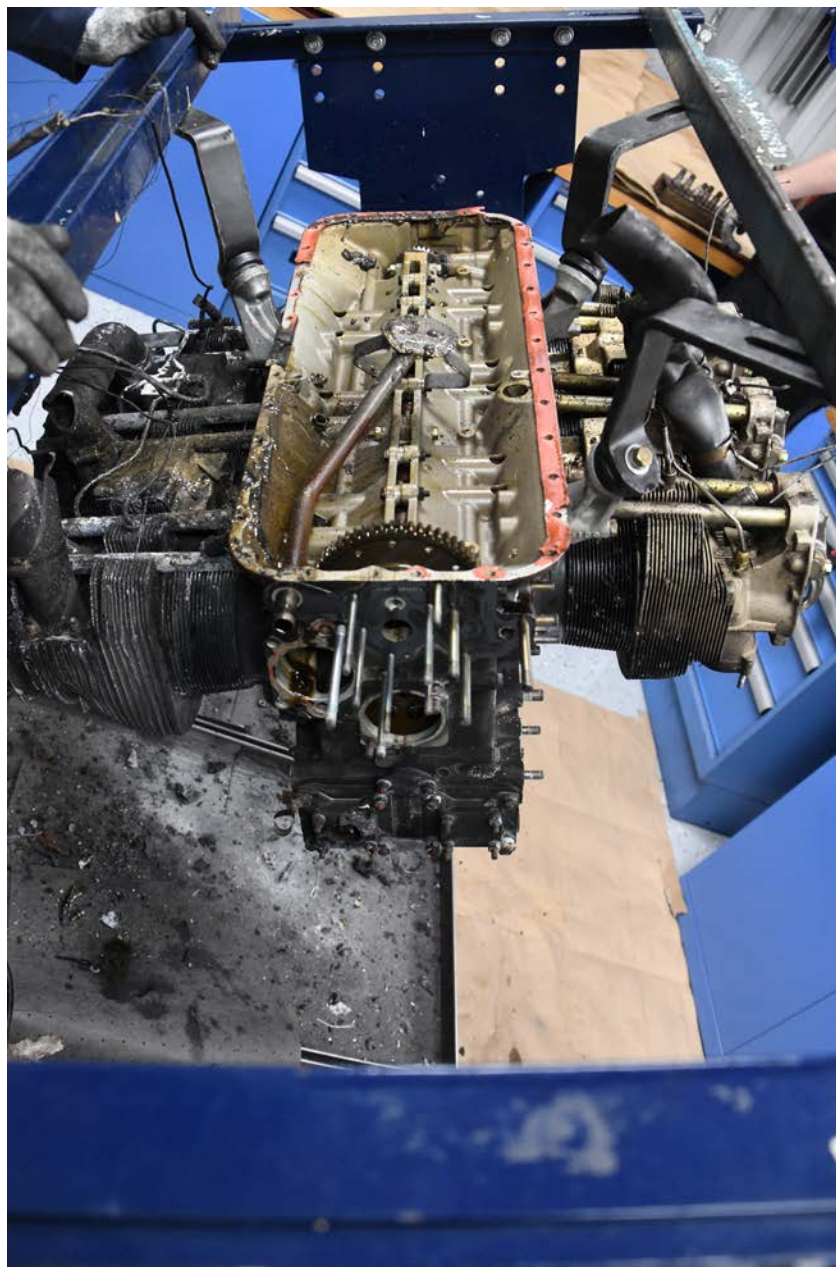
Photo 26 - View of the engine with the oil sump pan removed.
