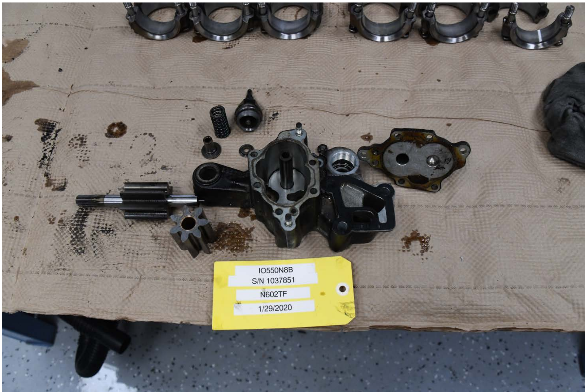
Photo 35 - View of the disassembled engine oil pump.
