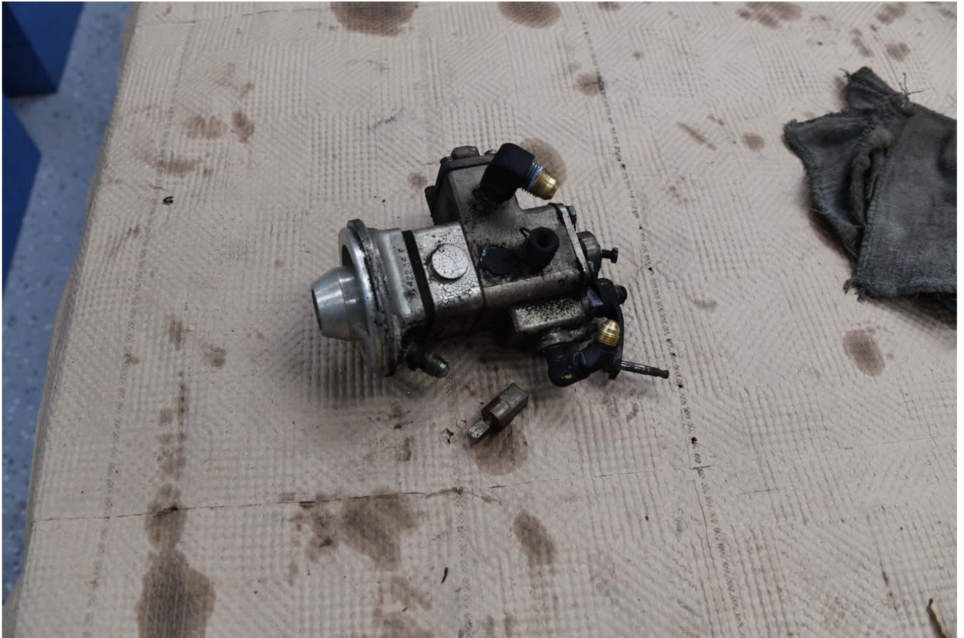
Photo 22 - Close up view of the engine driven fuel pump and its intact coupling.
