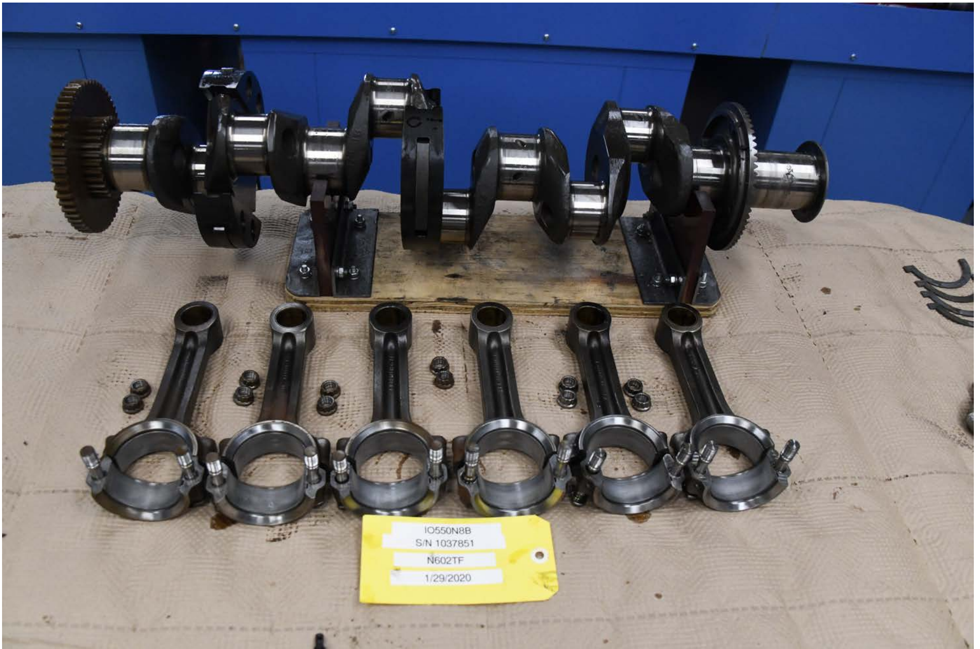
Photo 36 - View of the disassembled engine crankshaft and connecting rods.
