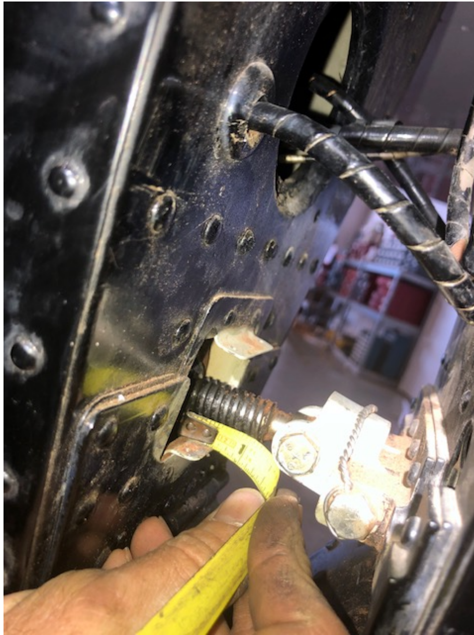
Photo 3 - Supplied view of the jackscrew with about 8 threads showing. Trim indicator is in the takeoff position.
