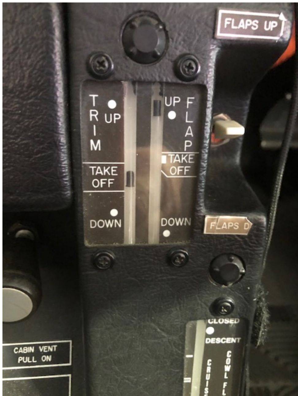
Photo 4 - Supplied view of the trim indicator in the takeoff position. The jackscrew has about 8 threads showing.
