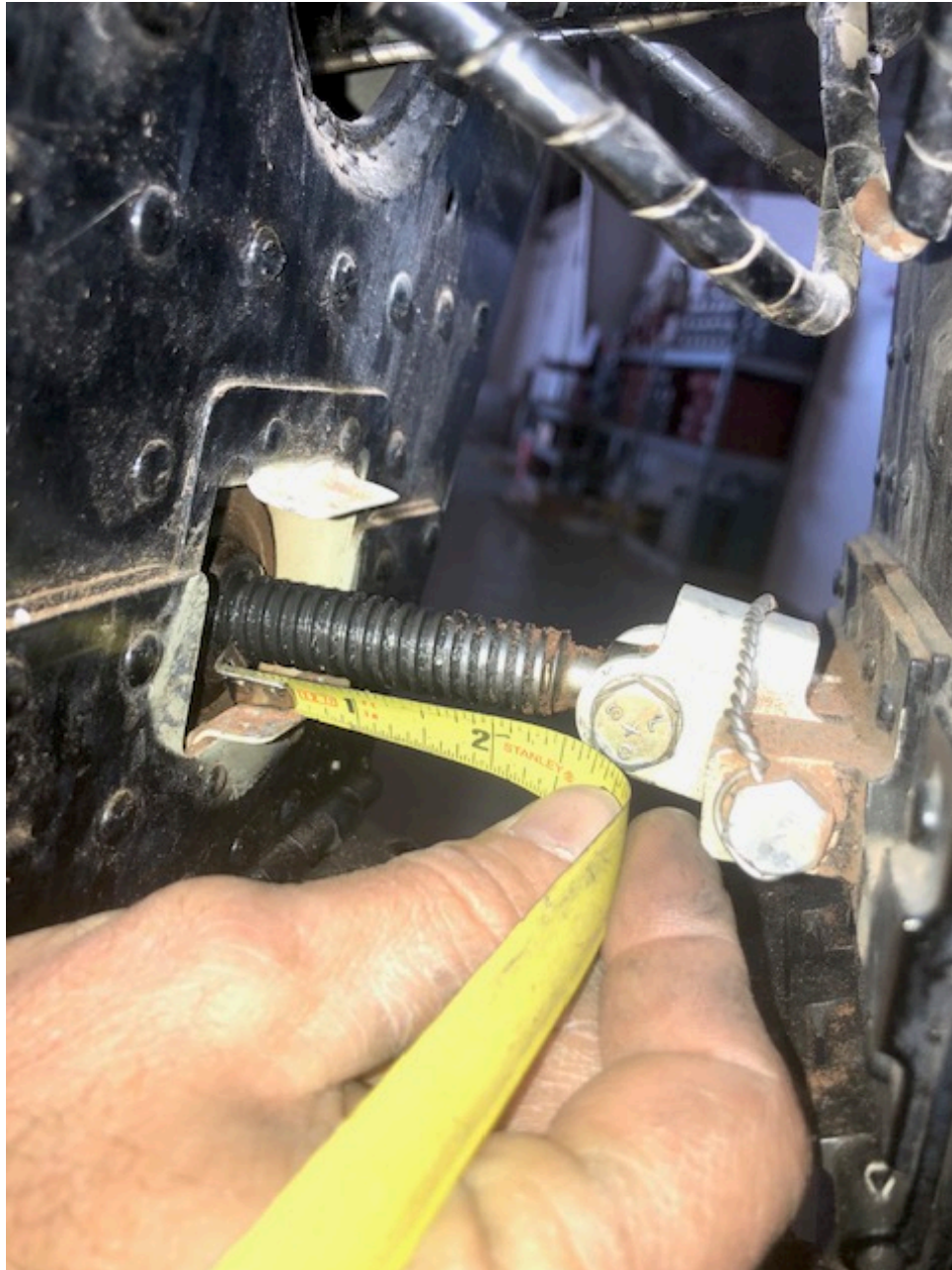
Photo 6 - Supplied view of the jackscrew at full extension.
