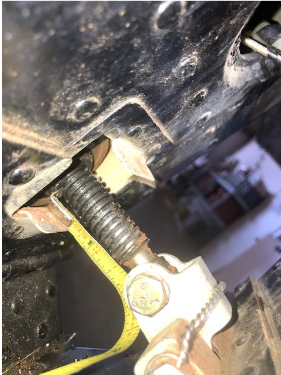
Photo 5 - Supplied view of the jackscrew with about 13 threads showing.
