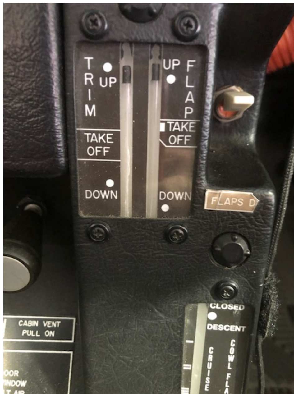
Photo 7 - Supplied view of the trim indicator in the full up position. The jack screw is at its full extension.
