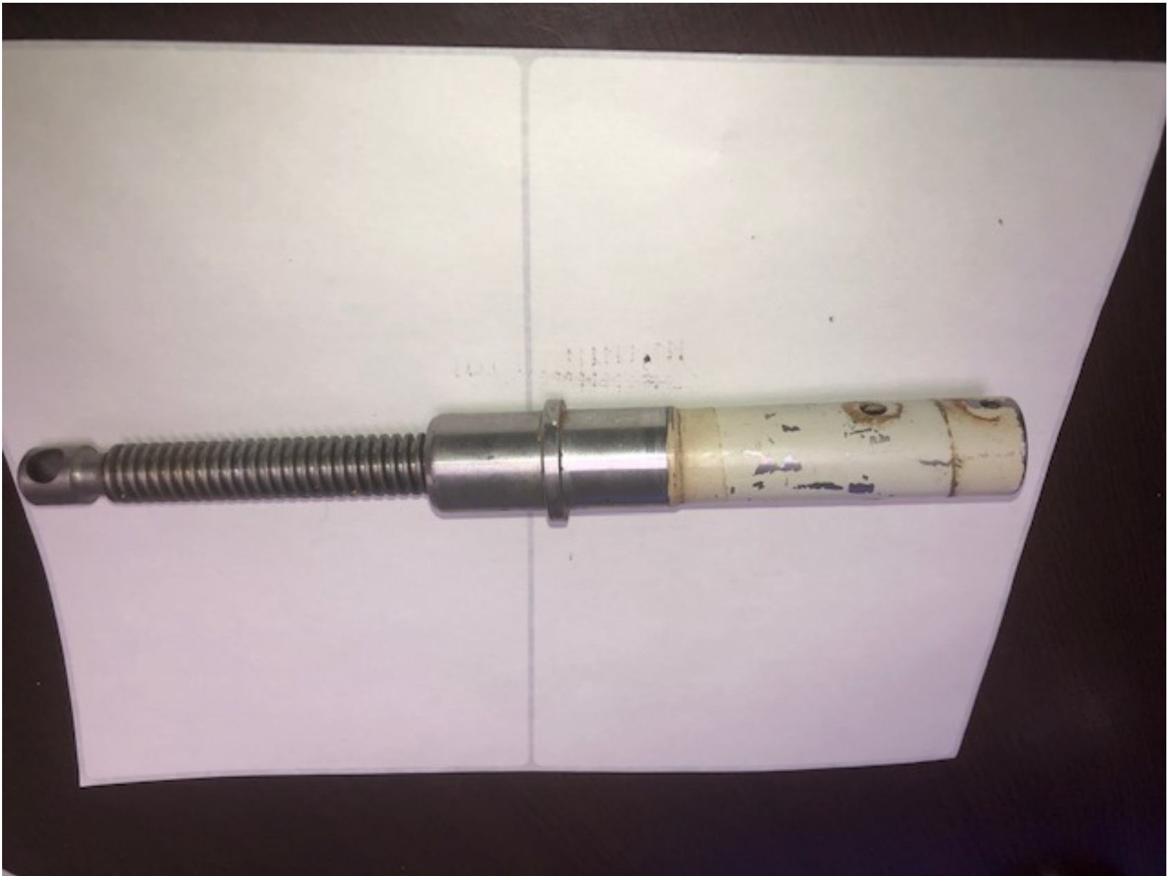
Photo 2 - Supplied view of the jackscrew in the trim system.
