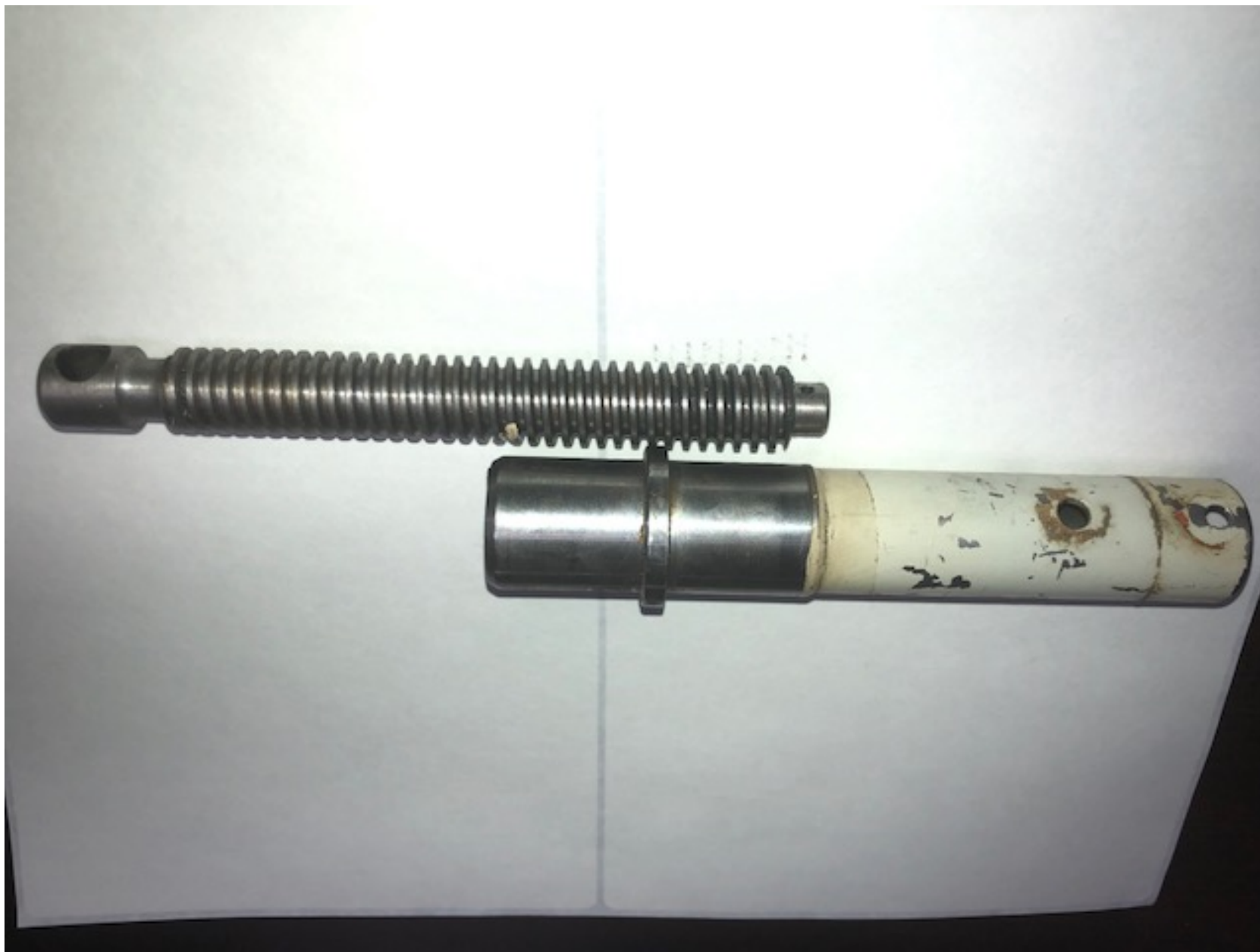
Photo 1 – Supplied view of the jackscrew in the trim system.
