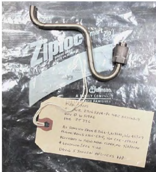
Figure 2. Shipping container (top) and the fractured tube (bottom left) and filter with remainder of tube still attached (bottom right) as received to the laboratory and removed from the packaging. No scale provided.
