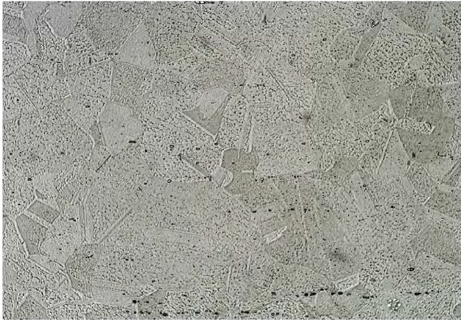
Figure 26. Detailed view showing the base metal microstructure. Etchant: Stainless No. 2.
