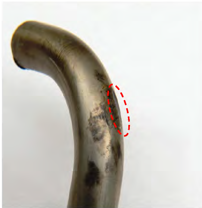
Figure 5. Detailed views showing the outer radius surface of the bend in the tube closest to the fracture. The tube exhibited a flat spot surrounded by patchy dark discoloration consistent with rub damage (red dashed outlined area).
