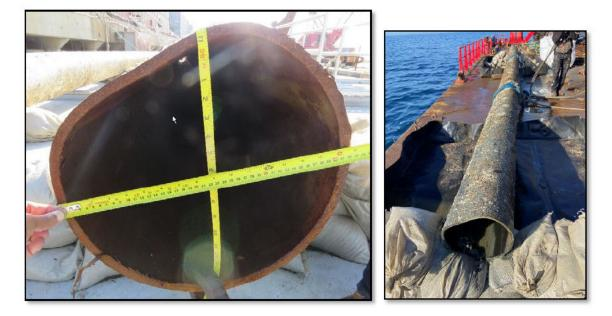
The anchor damage caused the spill. Specifically, metallurgical experts, including one retained by the *Beijing*, determined that a fatigue mechanism through cyclic loading caused the initial, *Danit*-caused crack to grow to a through-wall crack and leak on October 1, 2021.
