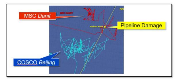
A reconstruction of the *Danit*'s Automatic Identification System ("AIS") data confirmed the vessel's location directly over the Pipeline with its anchor down:
