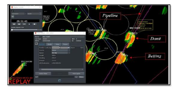
As the vessels' anchors dragged along the seafloor, they hooked the Pipeline and bent a 4,000-foot section of it. The anchors damaged and displaced the Pipeline by up to 105 feet, stripping off its protective concrete casing in the process. This chart shows both the anchor drags in the sand, the Pipeline's plotted location, and the Pipeline's displaced location:<sup>27</sup>
