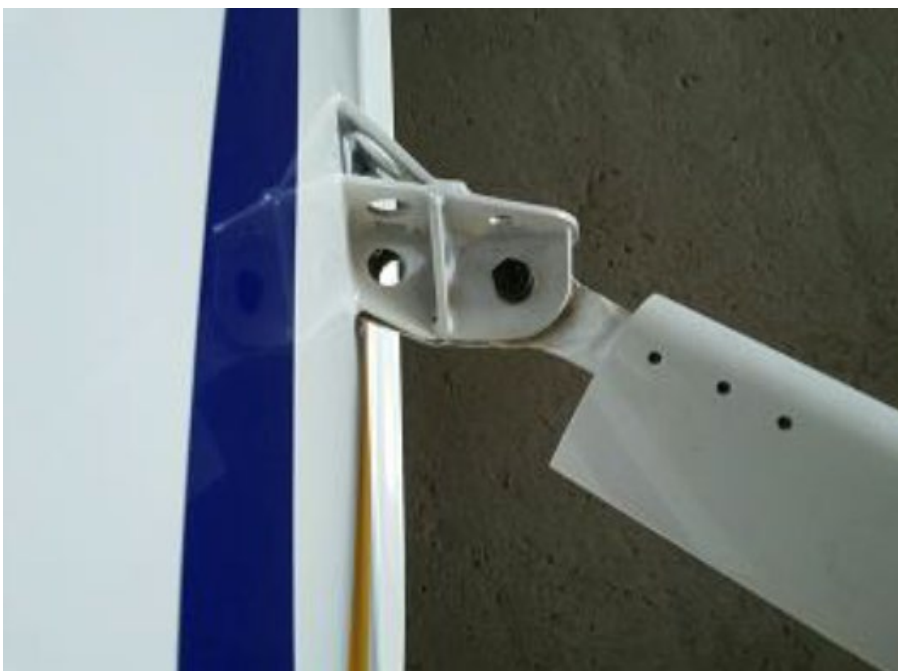
Figure 2: Lower wing strut attachment
