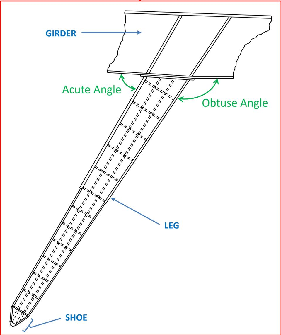
**Figure 3.** Schematic showing the outward facing side of a leg mating with a girder. (Schematic not to scale)
