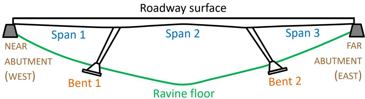
**Figure 1.** Plan view composite photo of the collapsed structure with the locations of the legs underneath the structure outlined and labeled (top), compared to schematics of the bridge in plan view (middle) and profile view (bottom).
