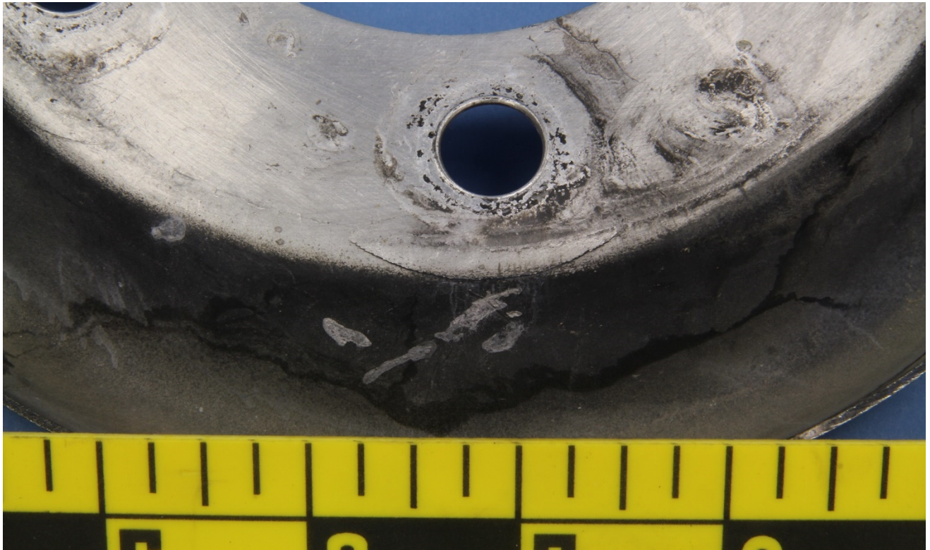
Figure 9 – View of the crack around the bolt hole #4.
