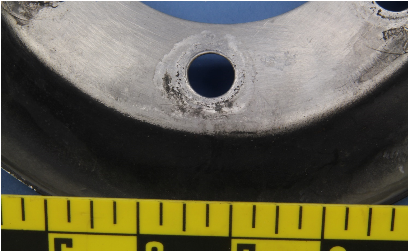
Figure 7 – View of the crack around the bolt hole #6.
