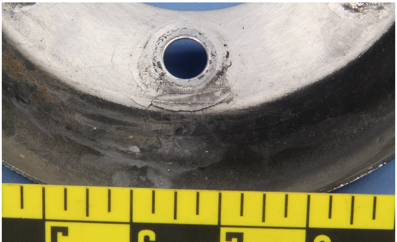
Figure 6 – View of the crack around the bolt hole #1.
