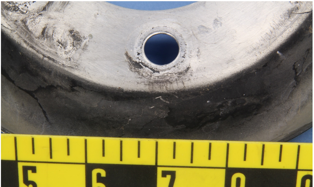
Figure 10 – View of the crack around the bolt hole #3.
