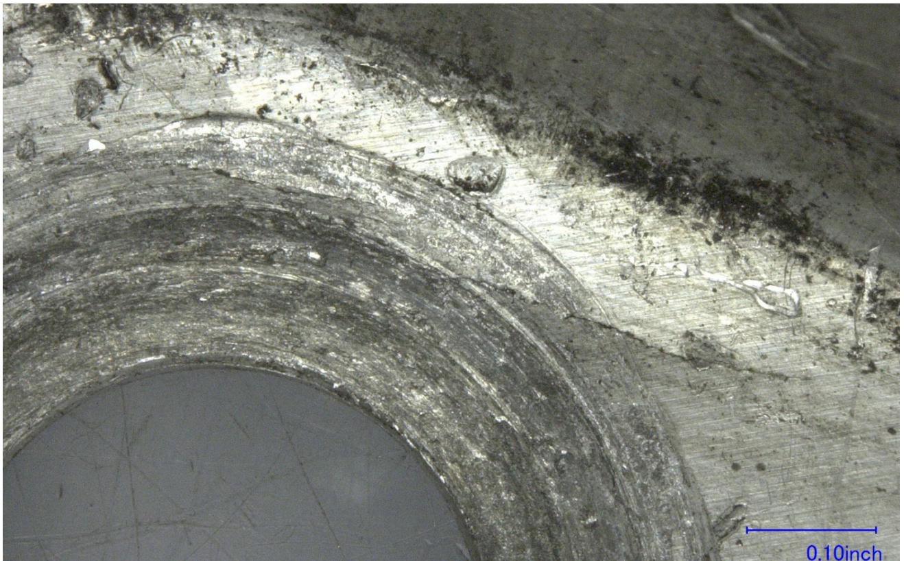
Figure 12 – Closer view of crack #3 around the bolt hole on the forward face.
