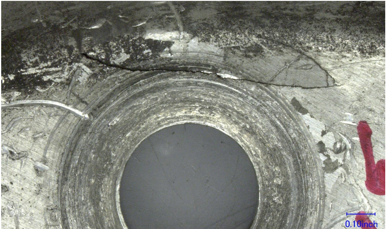
Figure 11 – Closer view of crack #1 on the forward side of the spinner.
