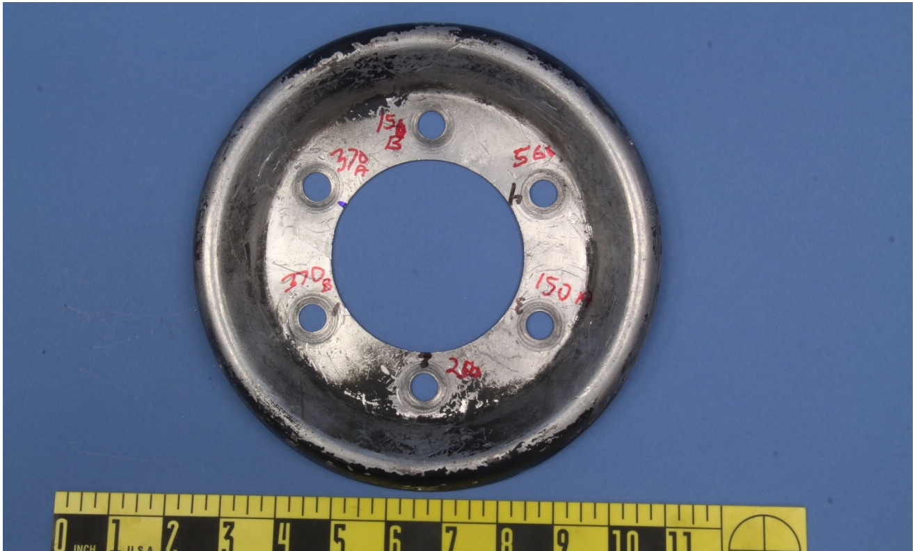
Figure 3 – View of the forward face of the spinner, after removing the bolts.
