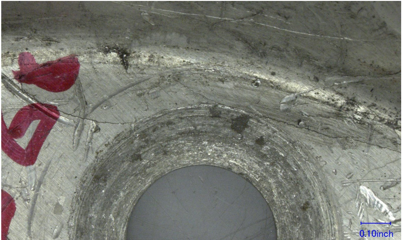
Figure 13 – Closer view of crack #4 from the forward face.
