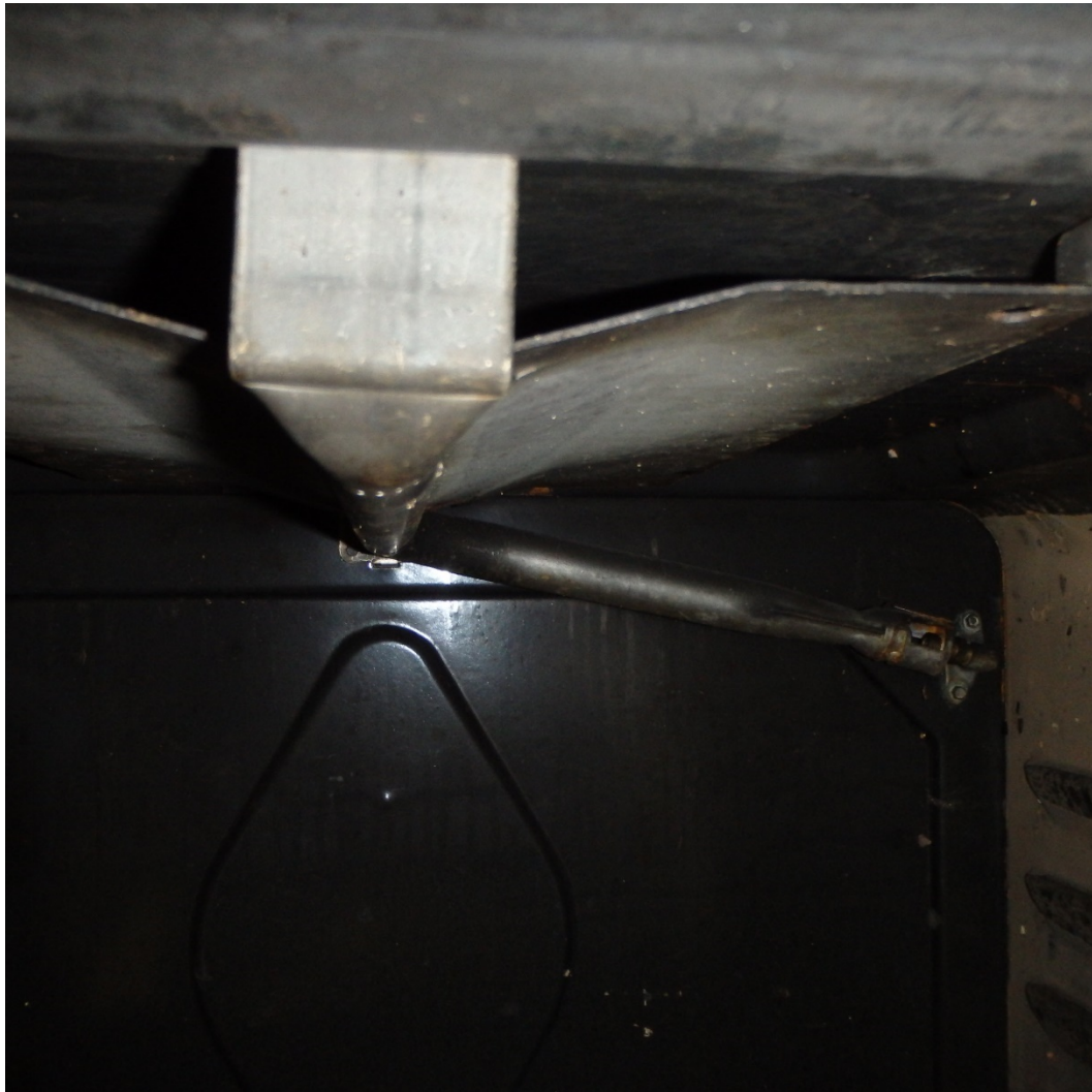
Figure 49. Pilot and glow bar of 3515 Durango Drive gas range. Photograph by DFR, June 2020.
