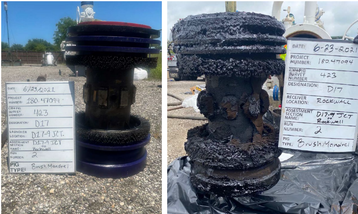
Figure 13. Run 2 Pre- and Post- Run Photographs (Courtesy of Atmos and Bobcat)
