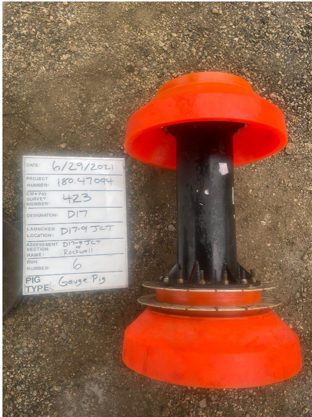
Figure 5. Photograph of gauge pig under umbrella prior to loading into the launcher. Taken 6/28/2021 at 3:28 PM. (Courtesy of Bobcat)
