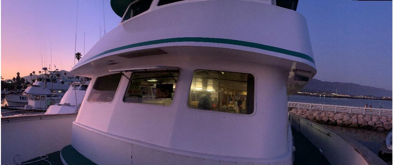
Figure 6. Preaccident photo of Conception forward salon windows. In this photo the center window is open. However, during the accident, the window was closed and secured as the crew attempted to access the space. The port and starboard windows were not designed to be opened. (Source: T. Thompson)
