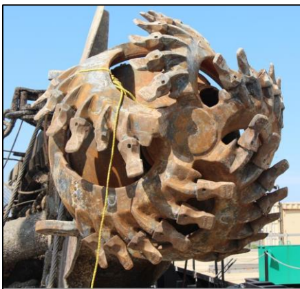
Figure 6. Waymon Boyd cutter-head postaccident. The yellow nylon line was attached during salvage and not part of original equipment (Source: US Coast Guard)
