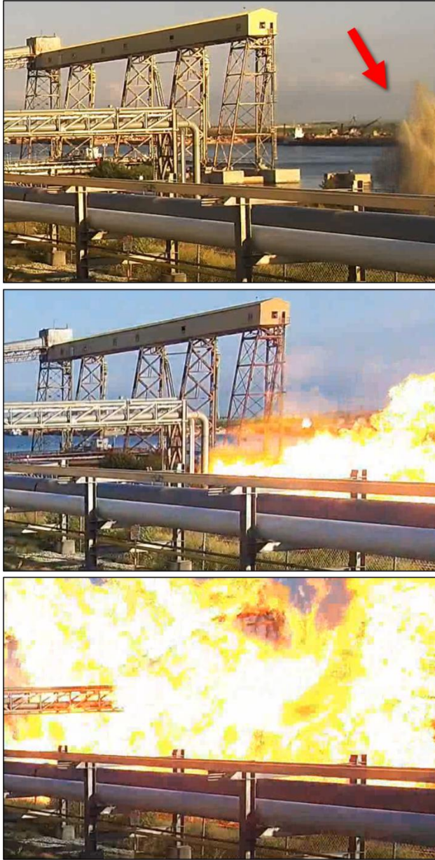
Figure 8. Screen captures from security camera footage showing, from top to bottom, the water and gas eruption prior to the explosion (as noted by red arrow), the initial explosion, and the ensuing fireball. The Waymon Boyd is outside of the frame of the camera. (Source: EPIC Crude Terminal Company)
