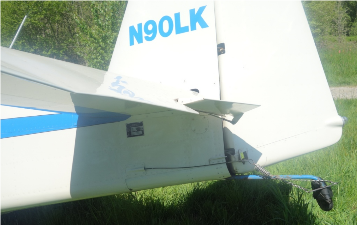
Figure 9 - Deflected Pitch Trim Tab
