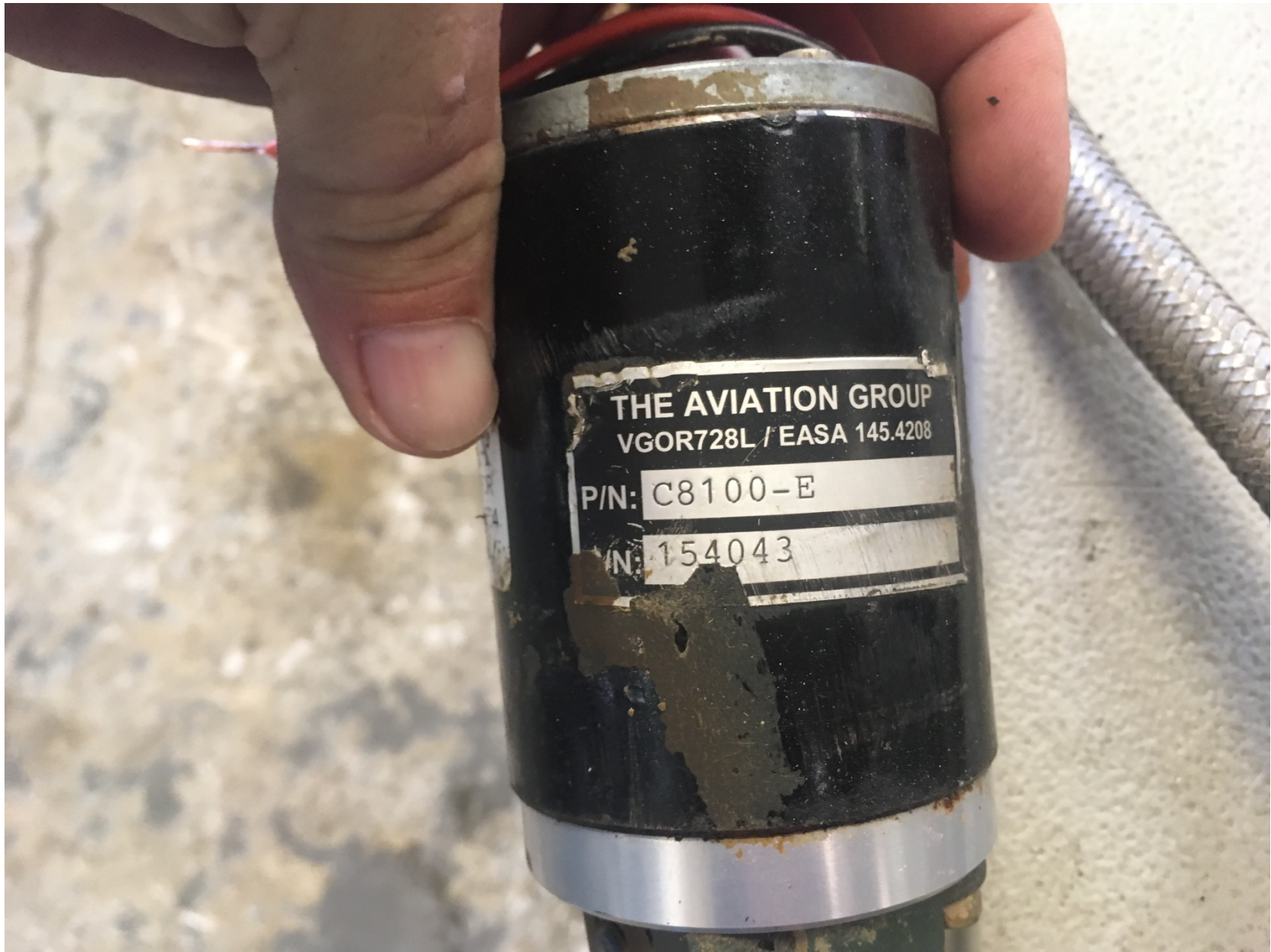
Photo 3 - View of the electric fuel pump. The label indicates part number C8100-E and serial number 154043.
