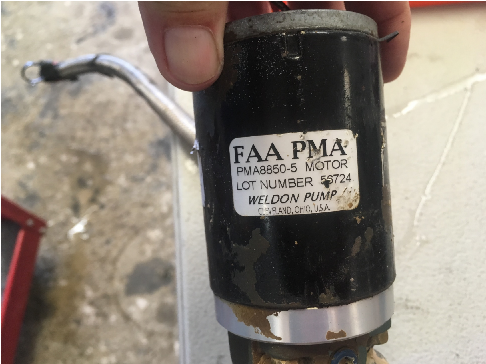
Photo 1 – View of the electric fuel pump.
