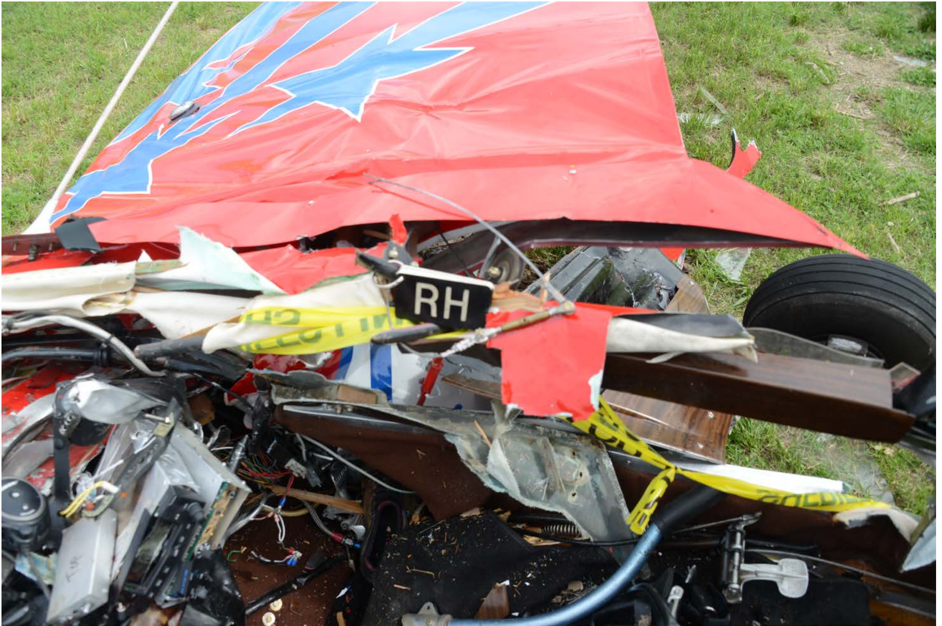
Photo 9 - View of a separated flight control cable exhibiting a broomstraw appearance.
