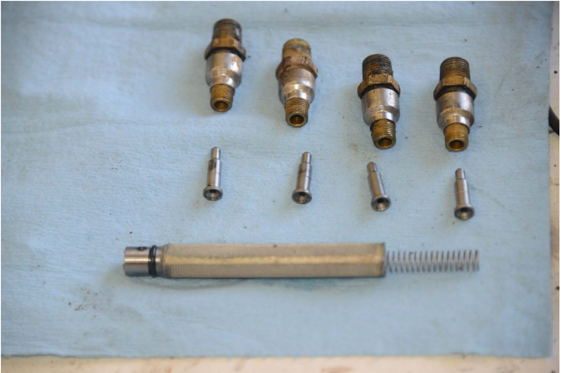
Photo 19 - View of the removed fuel injectors and fuel servo filter.
