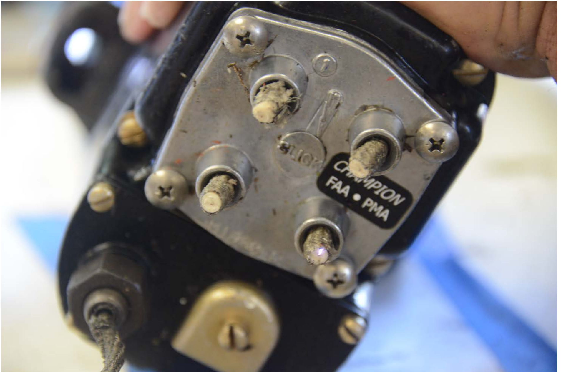
Photo 16 – Left magneto exhibiting a spark when its drive gear was rotated.
