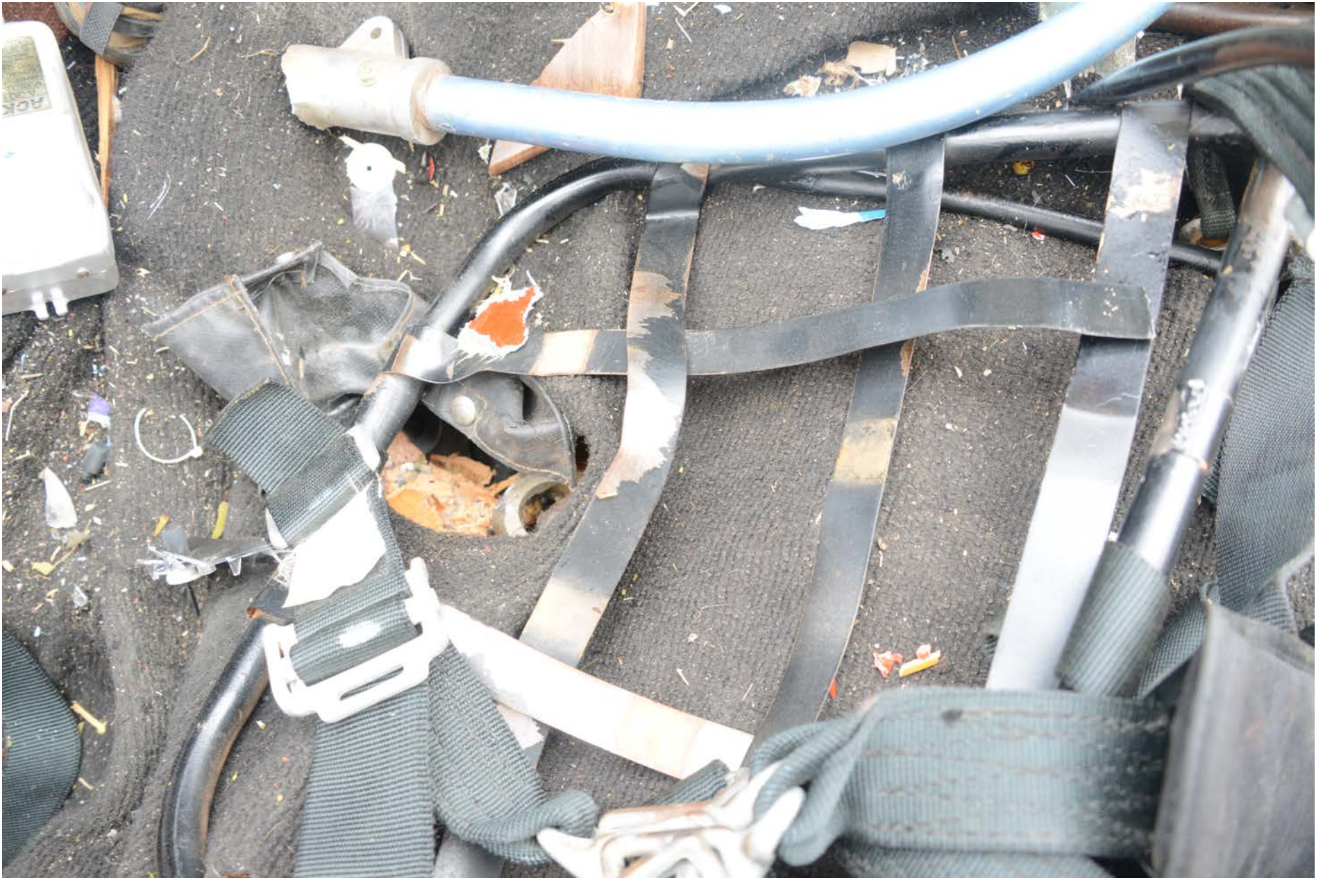
Photo 10 - View of the front control stick and an attached section of its stick socket as found separated from its stick socket assembly.
