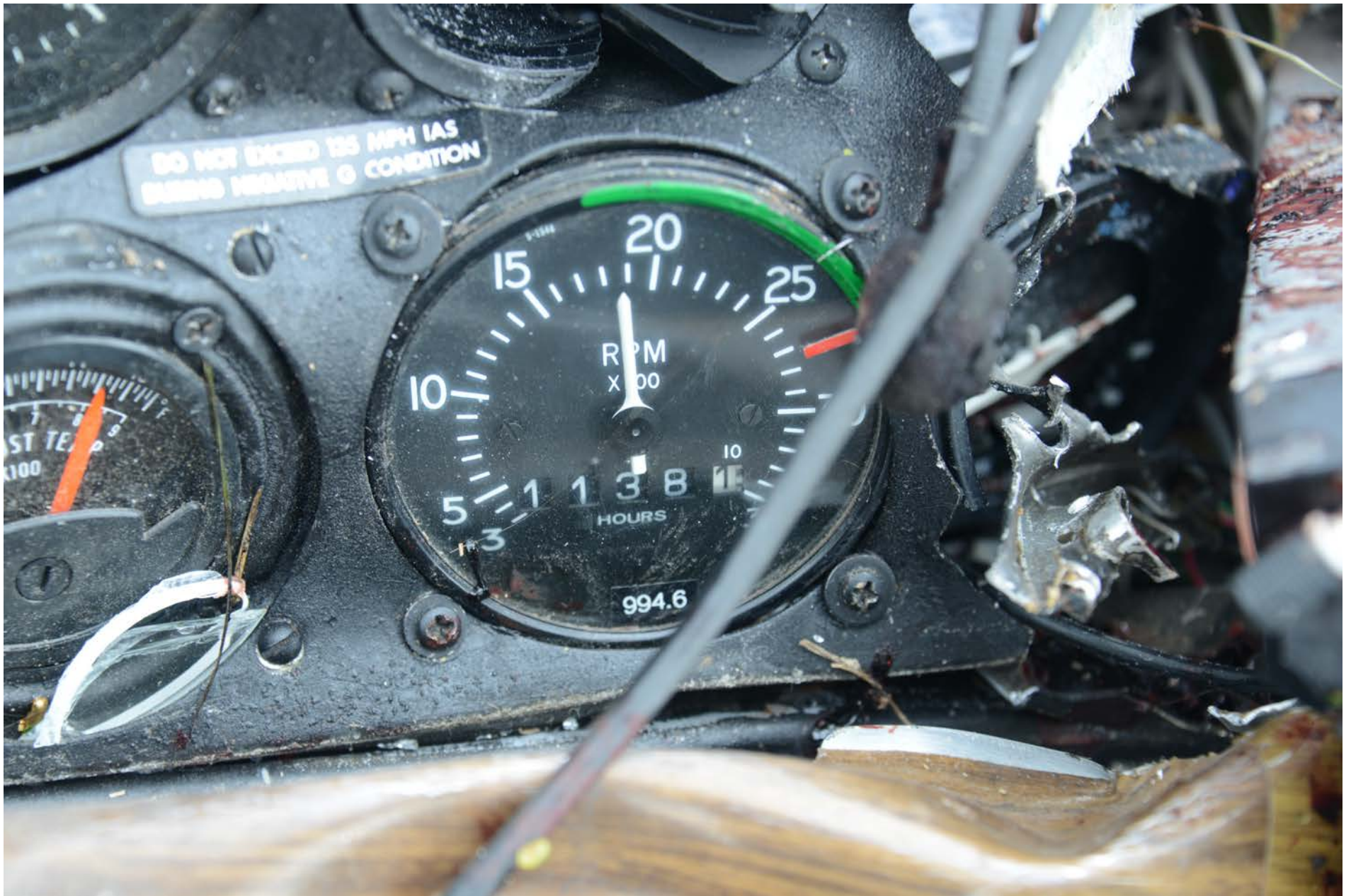
Photo 7 - View of the cockpit instruments to include a tachometer indicating about 1,875 RPM and 1138.1 hours.
