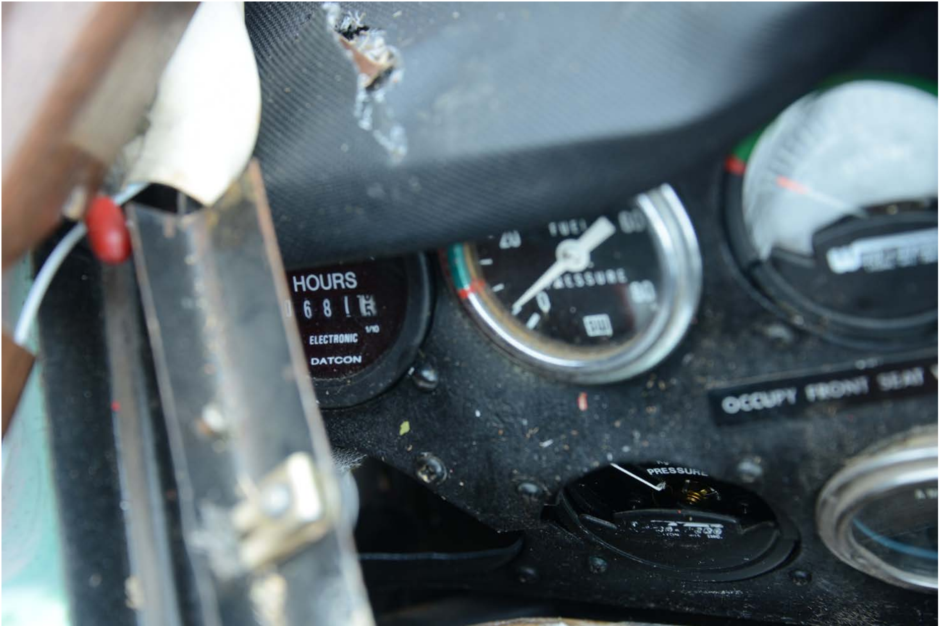
Photo 6 - View of the cockpit instruments to include an hour meter indicating 0681.5 hours.
