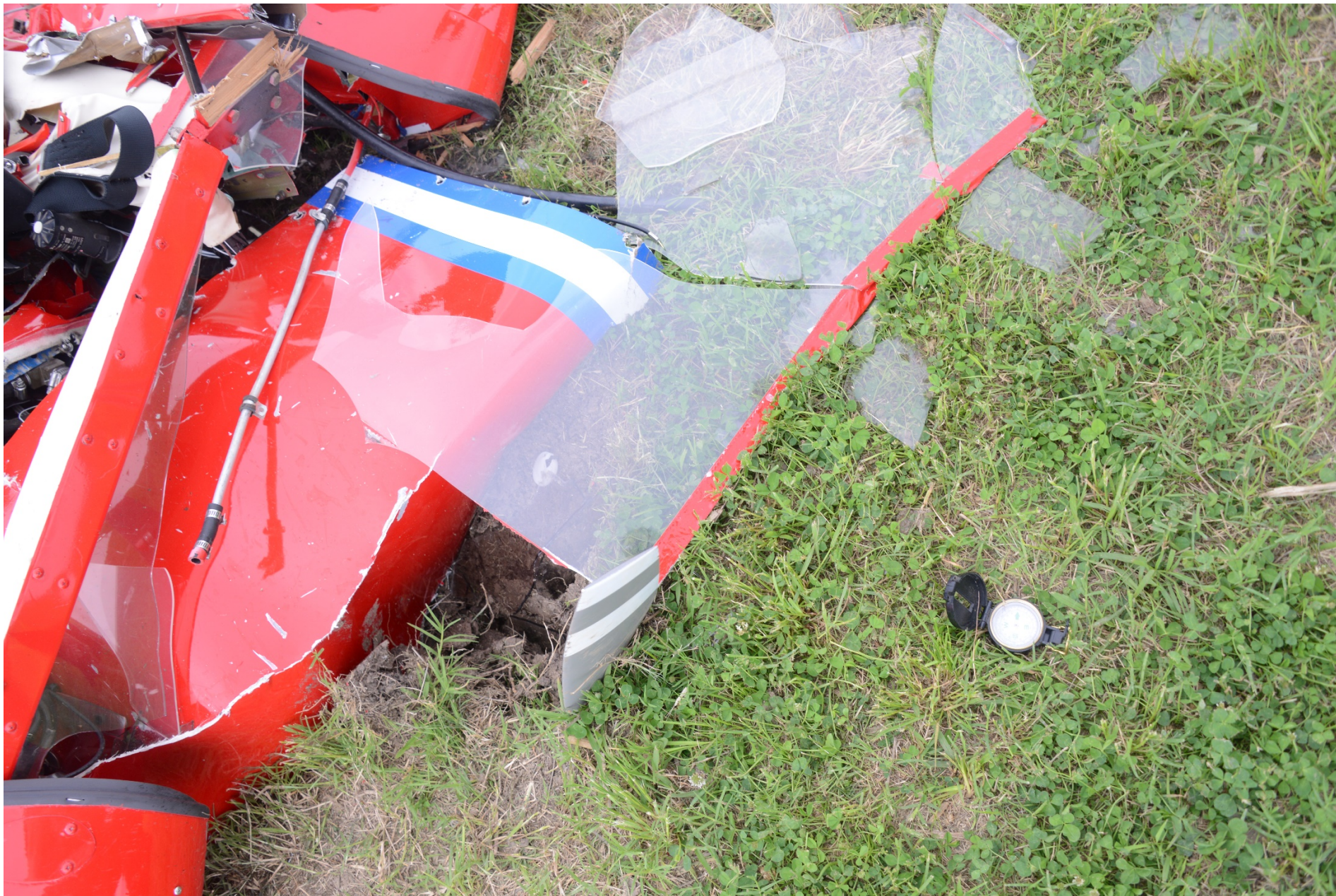
Photo 1 – View of the airplane nose impacted in terrain and a section of exposed propeller blade.
