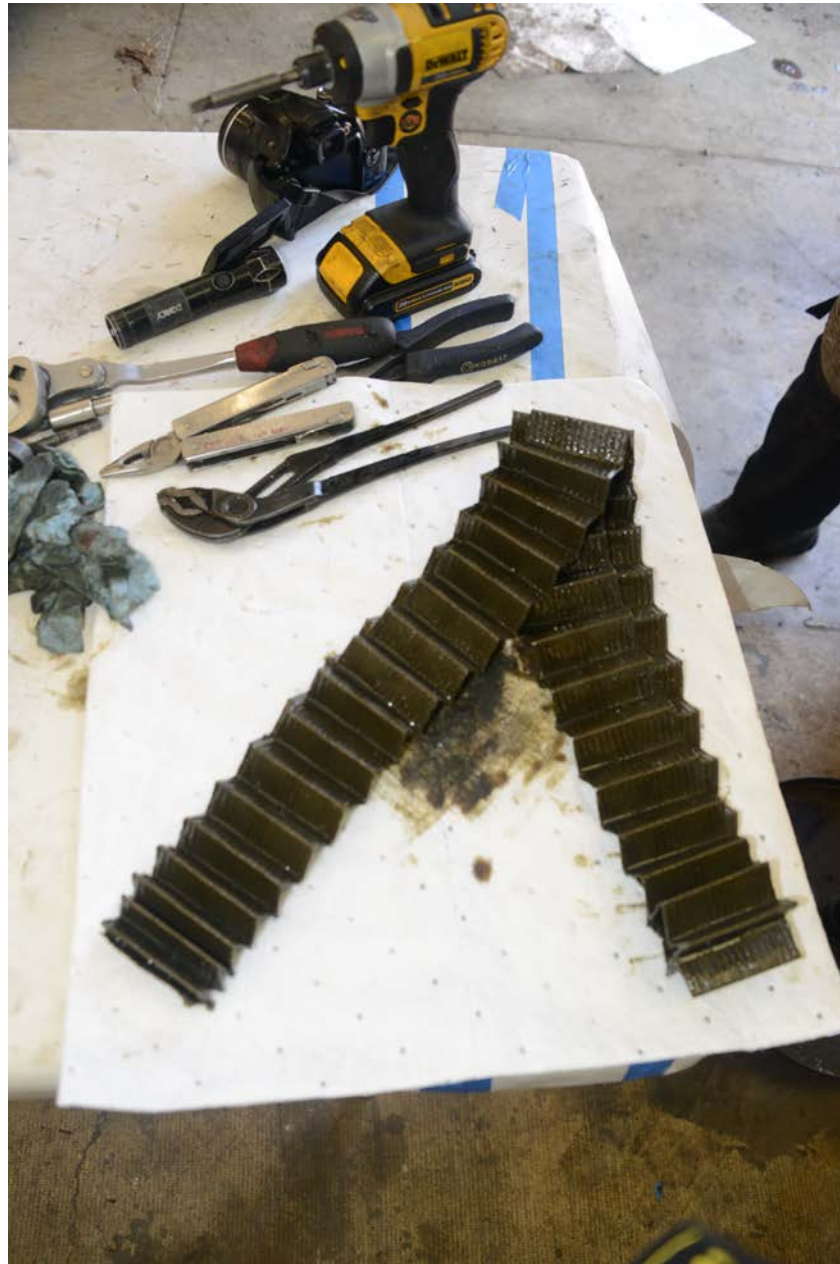
Photo 20 - View of the removed oil filter element.
