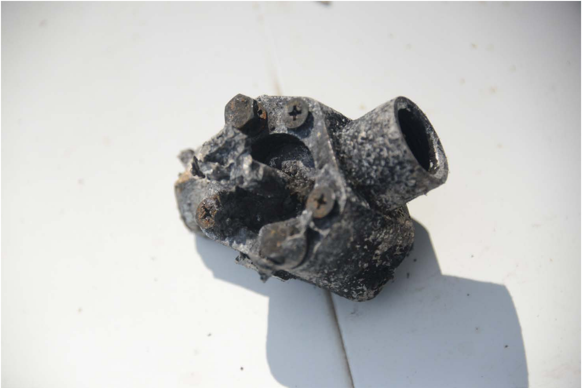
Photo 15 - View of the fuel selector valve.
