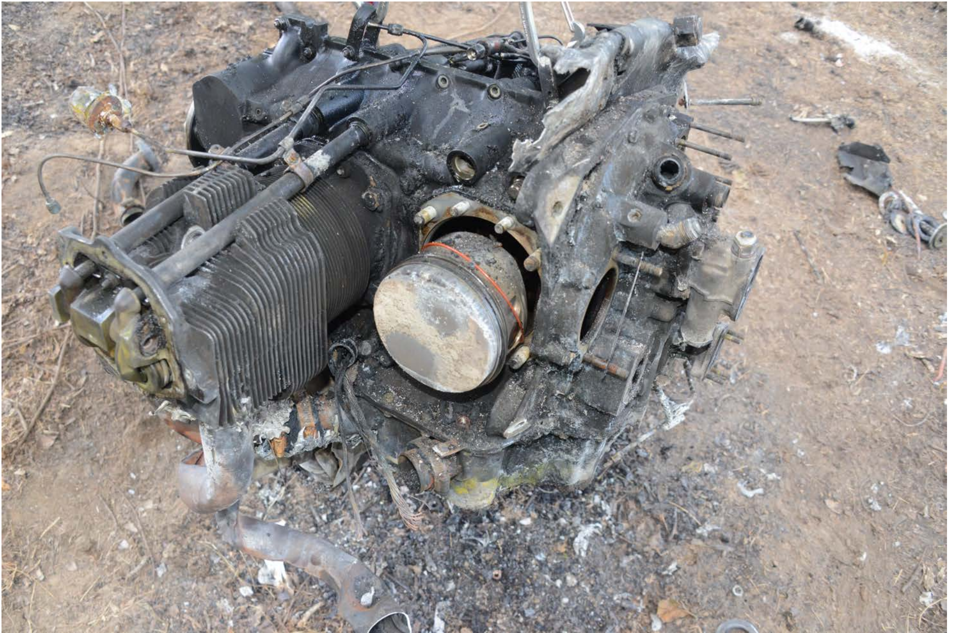
Photo 23 - View of the left rear side of the engine with the No. 4 cylinder removed.
