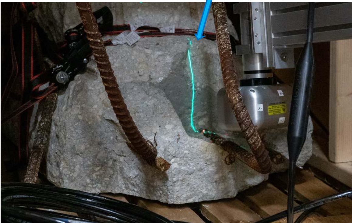
Figure 6: Macro photos of a laser scan of the flat area on the bottom of Member 12. The green line in the bottom image is the laser projected onto the surface.
