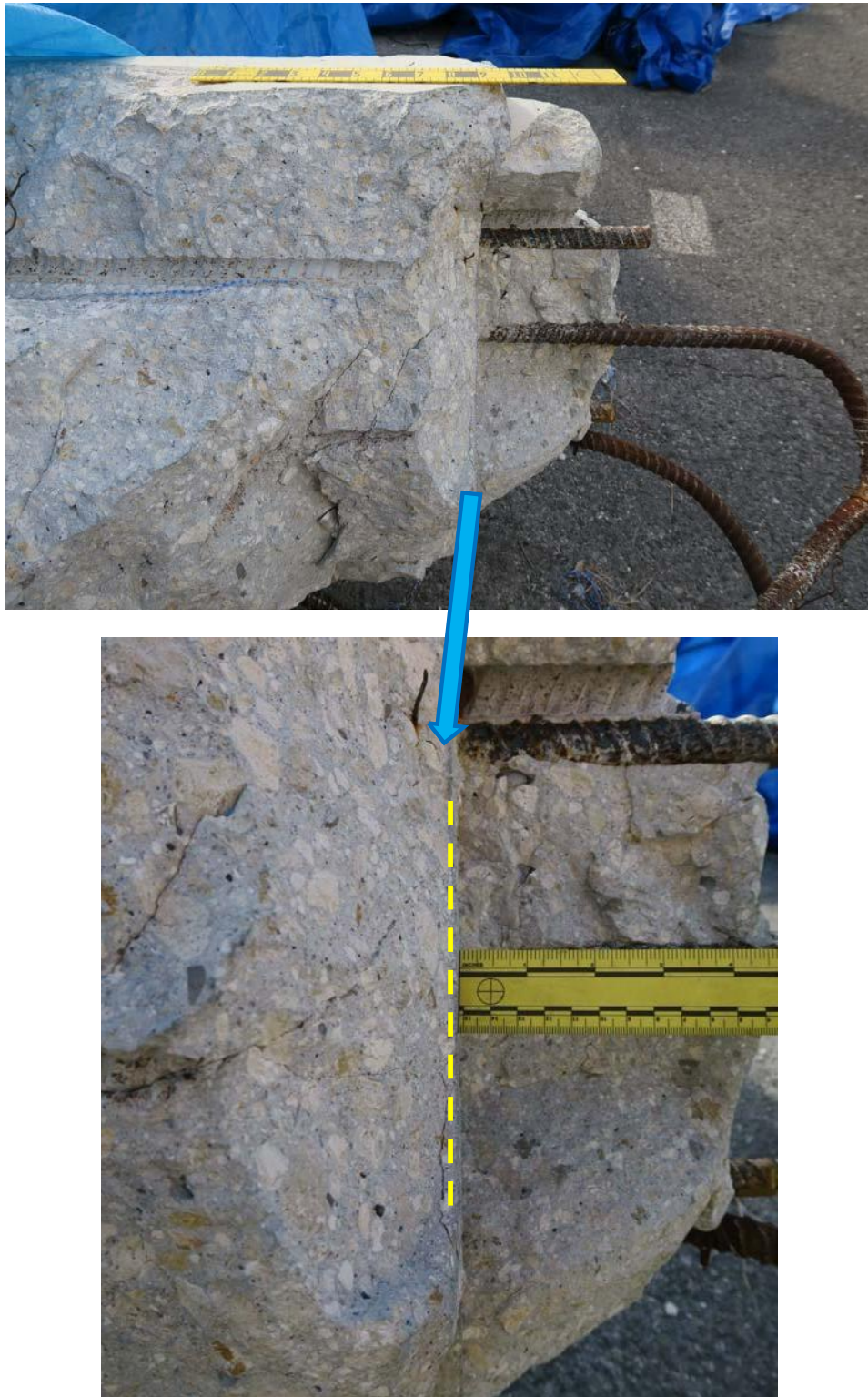
Figure 4: Macro photos of the bottom of Member 12 viewed in profile. The yellow dotted line indicates the straight plane of the flat area observed.
