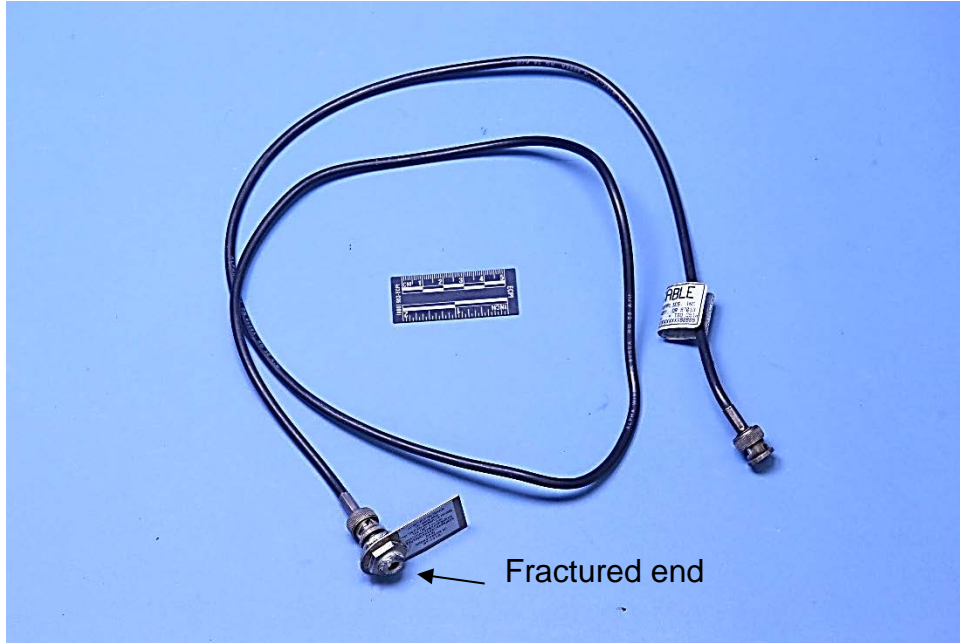
Figure 1. As-received ELT antenna cable with fractured section that attaches to the antenna at the airframe.
