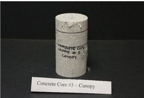
(c) Concrete Core #3 – Canopy: Front
