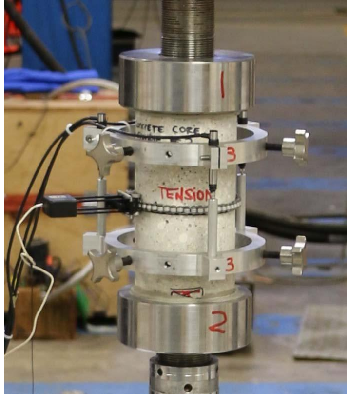
Figure 11. Close-up view of concrete tension test sample in the test machine
