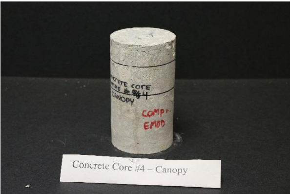
(e) Concrete Core #4 – Canopy: Front
