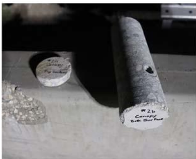
Figure 10: Photos showing the actual locations where concrete core samples for materials testing were taken from the canopy on-scene.
