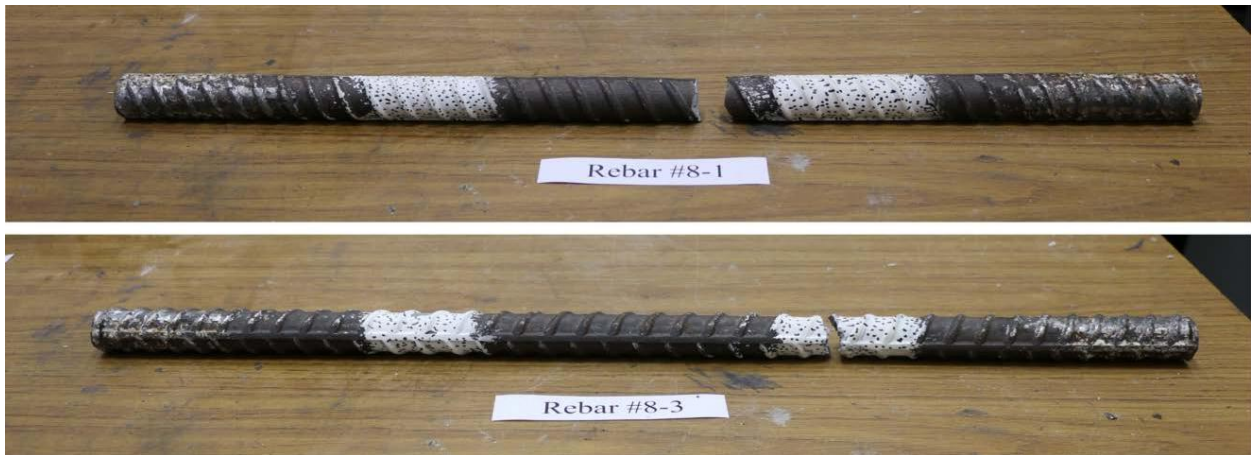
Figure 46. Photographs of fractured #8 bar specimens
