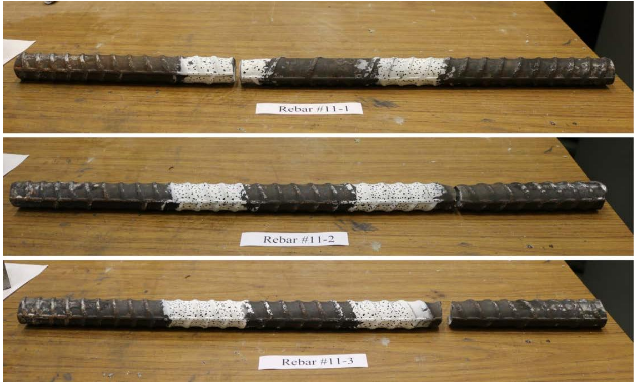
Figure 47. Photographs of fractured #11 bar specimens
