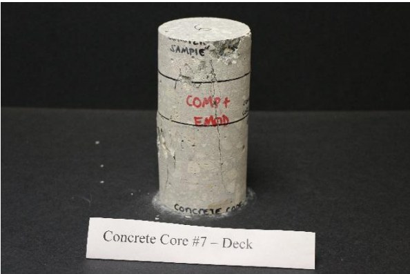
(e) Concrete Core #7 – Deck: Front
