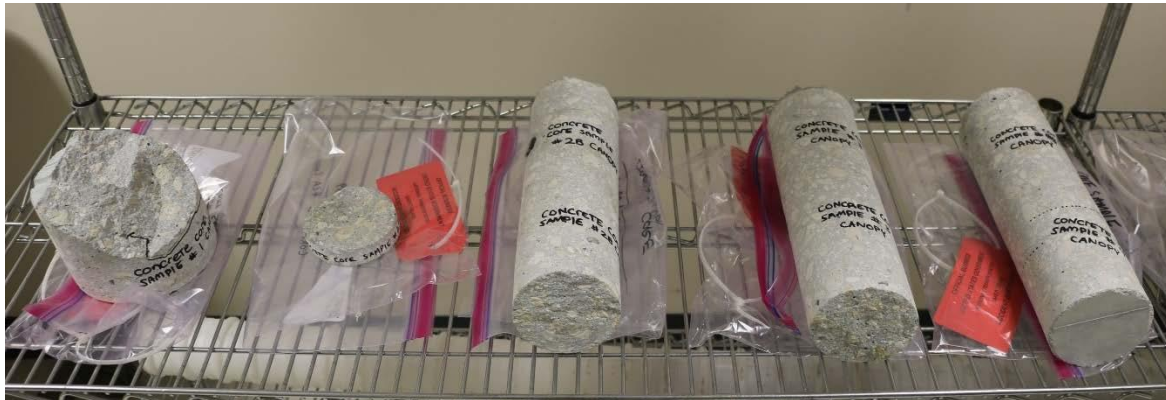
Figure 4. Concrete core samples extracted from the canopy of the bridge, from left-to-right, Core #1 – Canopy, #2A – Canopy, #2B – Canopy, #3 – Canopy, and #4 – Canopy
