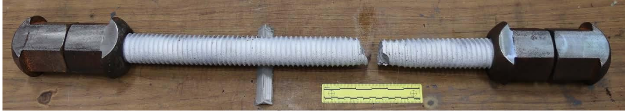
Figure 35. Photo of fractured Diagonal 11 bar
