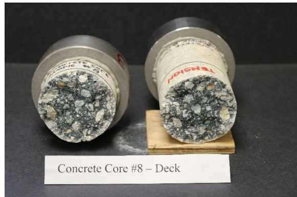
(b) Fracture surface
