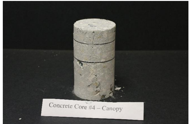
(f) Concrete Core #4 – Canopy: Back
