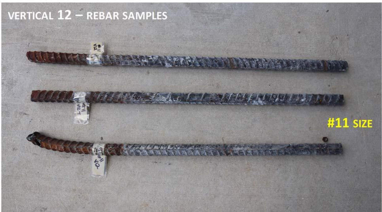
Figure 16: The top photo shows the location in Vertical 12 where the bars shown in the bottom photo were removed at the FDOT yard. The bars were sent to TFHRC for testing.
