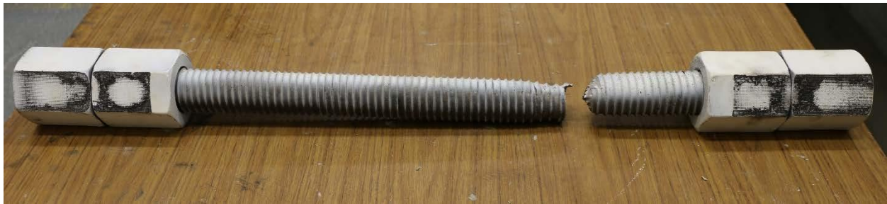
Figure 36. Photo of fractured virgin bar
