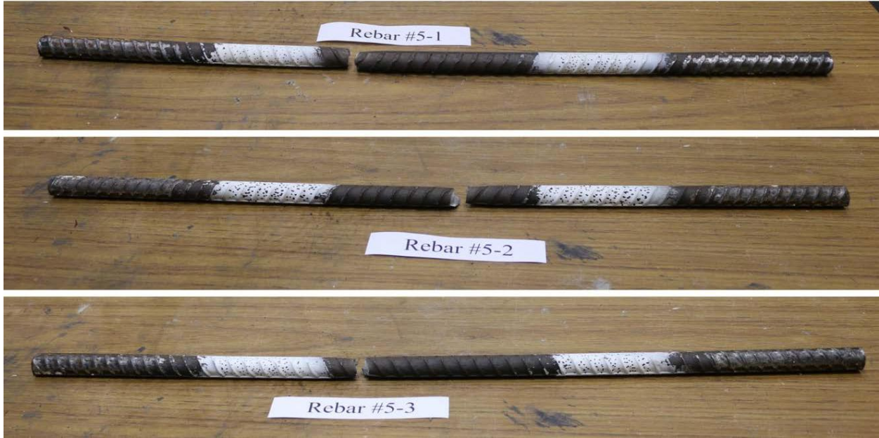
Figure 45. Photographs of fractured #5 bar specimens
