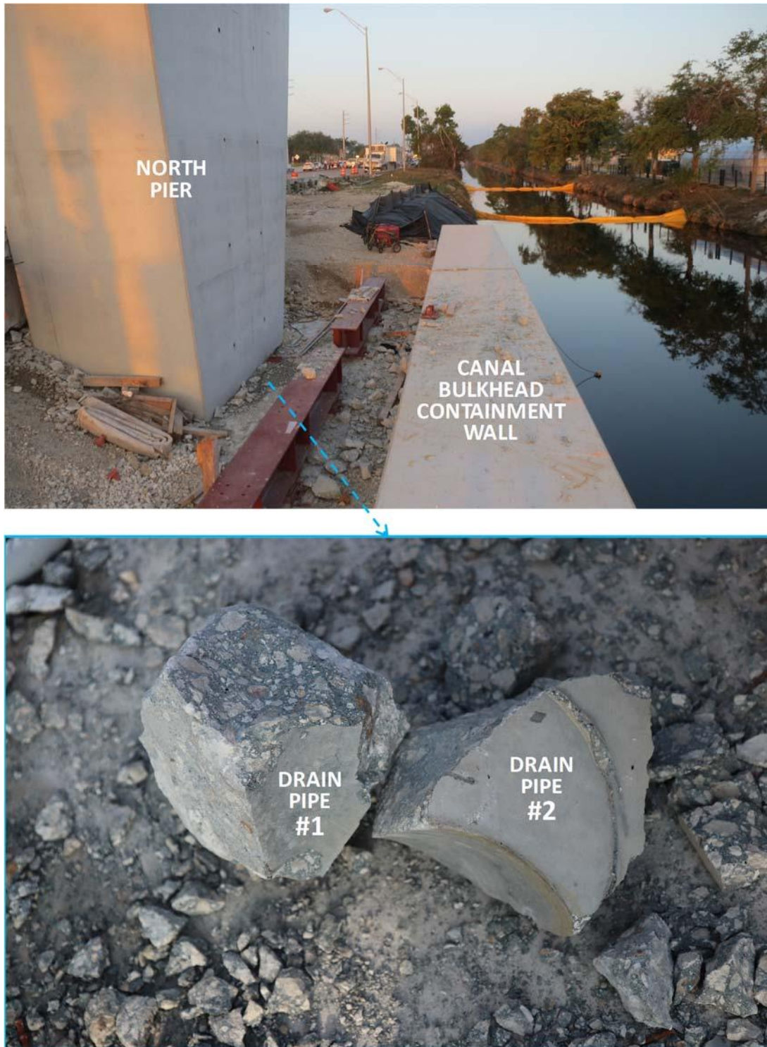
Figure 13: (Top) Photo showing the general location where two pieces of concrete with smooth geometrical features were found on the north side of the collapse site, between the north pier and the canal bulkhead containment wall. (Bottom) Photo showing the two pieces of concrete after handling and visual inspection.
