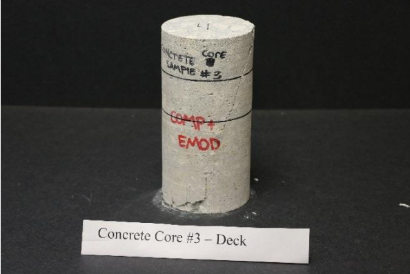
(a) Concrete Core #3 – Deck: Front
