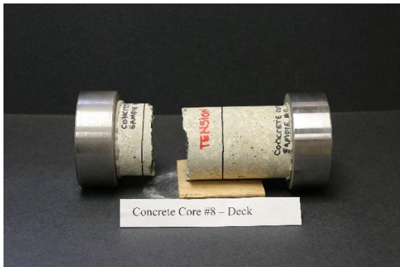
(a) Fracture location
