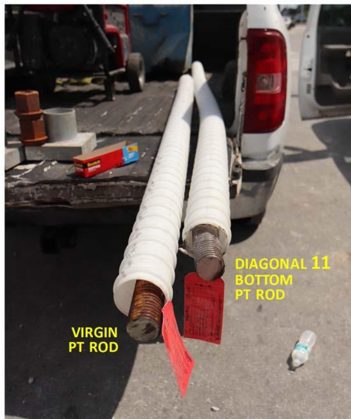
Figure 14: Photos showing the on-scene removal of the bottom PT rod from Diagonal 11 (top) and the two PT rods shipped to TFHRC for testing (bottom).
