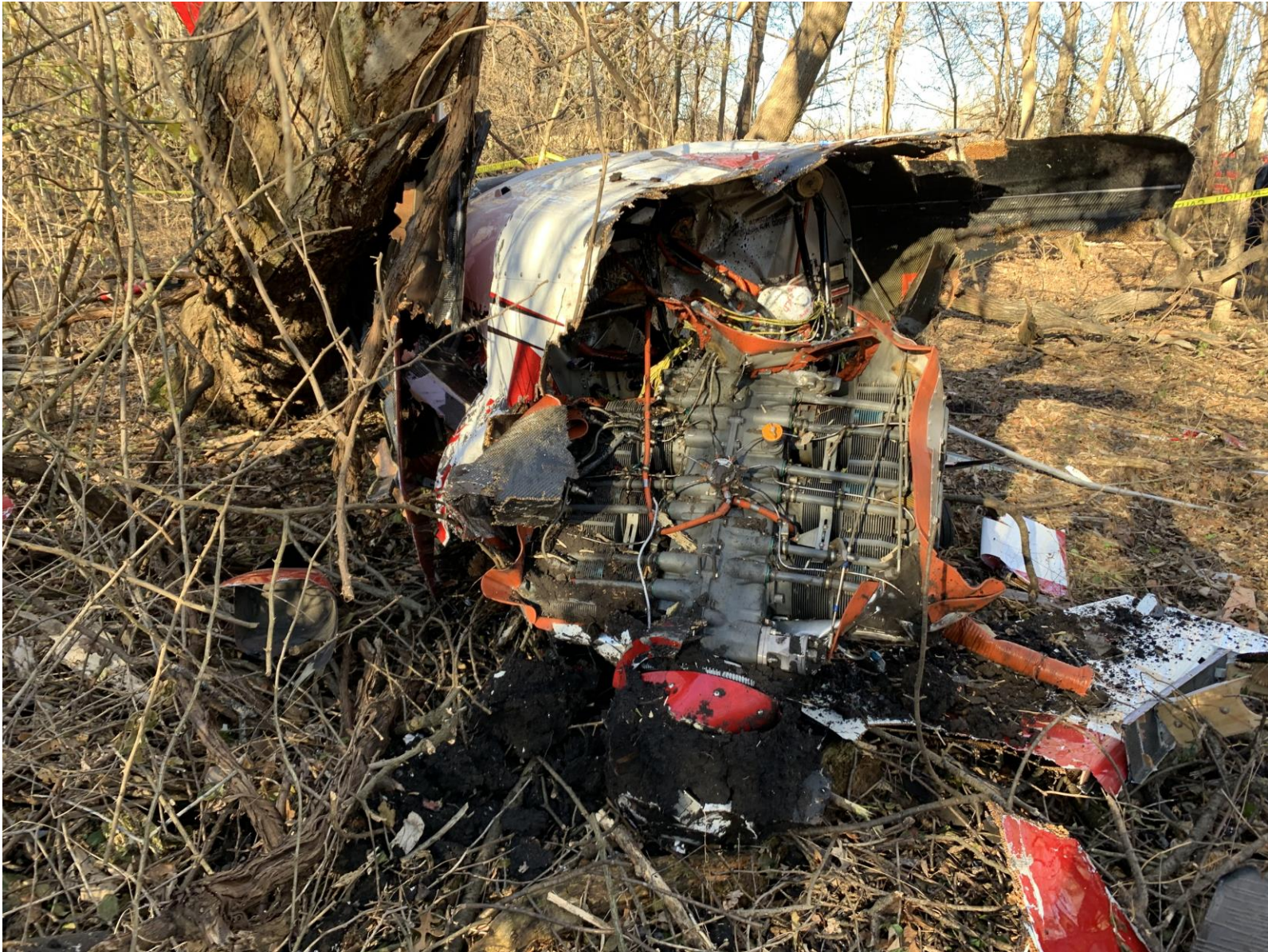
Photograph 4 - Engine at Accident Site
