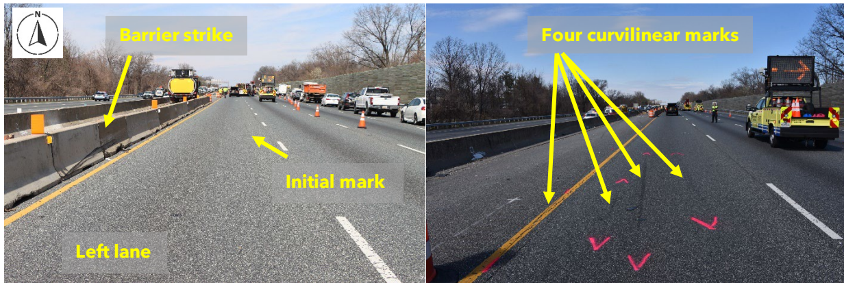
Figure 10. Images taken by MSP investigators depicting the roadway evidence. Image on the left shows the initial tire friction mark. The image on the right shows the four curvilinear friction marks. (Source: MSP modified by NTSB)
