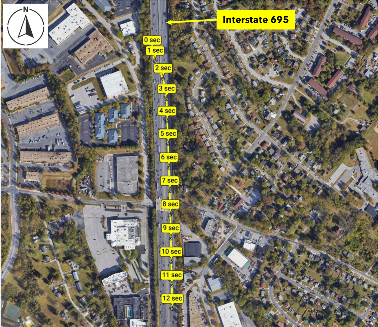
Figure 7. Image of northbound I-695 leading up to an including the area of the collision. Overlaid on the image is the positioning data associated with the Acura. (Source: Google Earth edited by NTSB)
