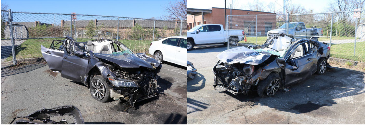
Figure 2. Images showing the damage to the Acura TLX. The image on the right shows the damage to the front left and left side. The image on the left shows the damage to the front right and right side.
