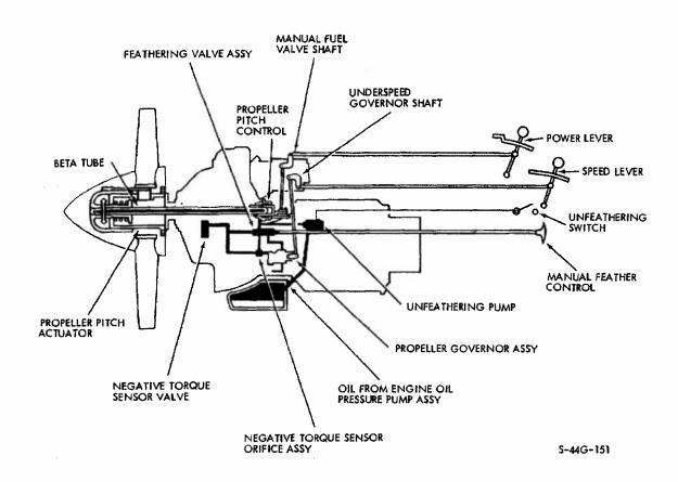
(Codes BA-BD) Simplified Power Management and Torque Sensing Diagram (Typical) Figure 5
