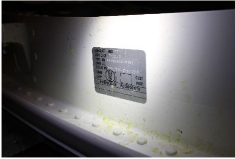
Figure 5. Left photo: LH MED plug Data Plate. Right photo: Markings on accident airplane [NTSB Photos]
