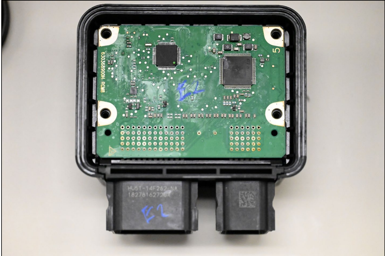
Figure 2: Exemplar 3's MCU installed into Exemplar 2
