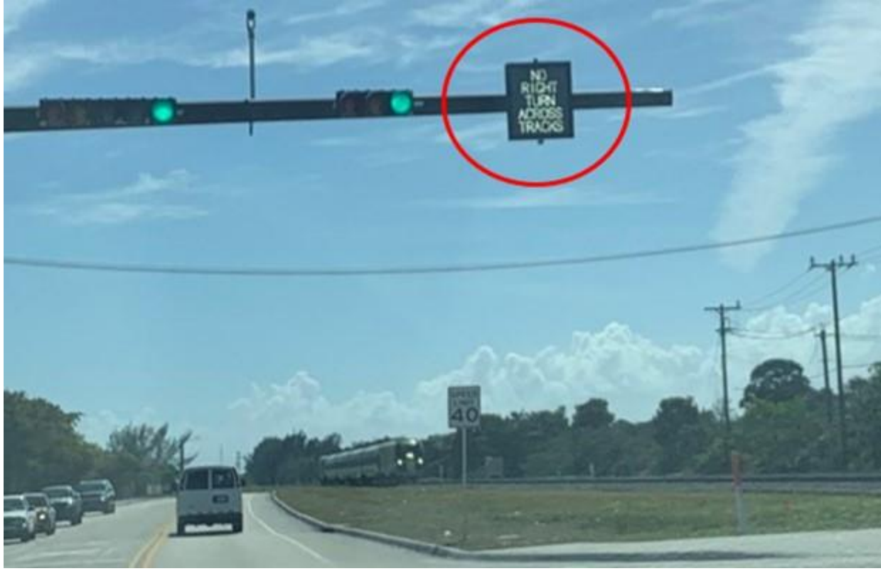
Railroad Signal and Highway Factors Photo 2 – View of Hidden Valley Boulevard grade crossing illustrating text only prohibition sign indicating “ No Right Turn Across Tracks ” with the Brightline passenger train shown in the background looking to the south
