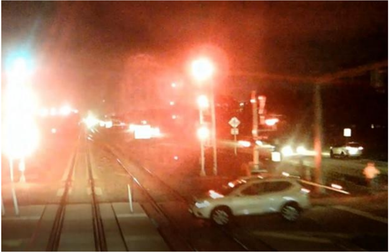
Railroad Signal and Highway Factors Photo 1 – View of freight train video and the gate down and fully lowered behind the SUV at the Lindell Boulevard grade crossing looking to the north (Source: Florida East Coast Railway)
