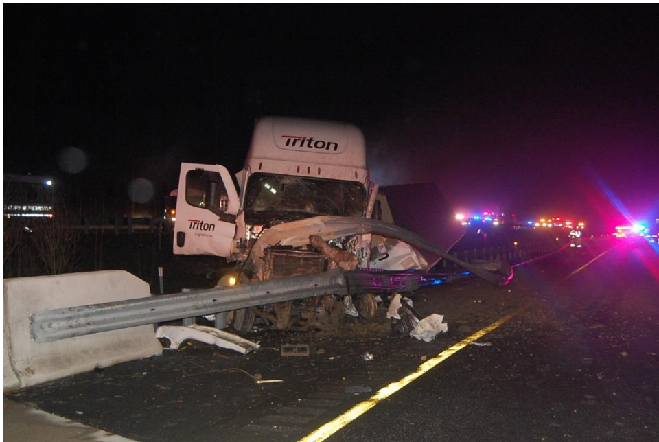
Highway Factors Photo 1 – View of strong post blocked-out W-beam guardrail that contained the Freightliner combination vehicle within the median standing in the leftmost travel lane in the westbound direction looking to the northwest (Source: Virginia State Police)
