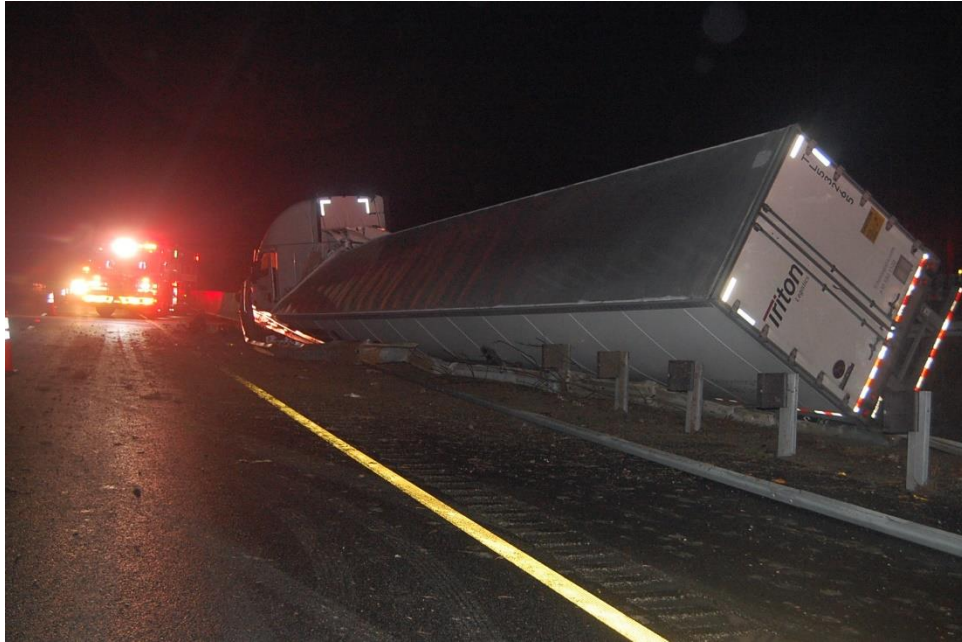
Highway Factors Photo 3 – View of strong post blocked-out W-beam guardrail that contained the Freightliner combination vehicle within the median standing in the leftmost travel lane in the westbound direction looking to the southeast (Source: Virginia State Police)
