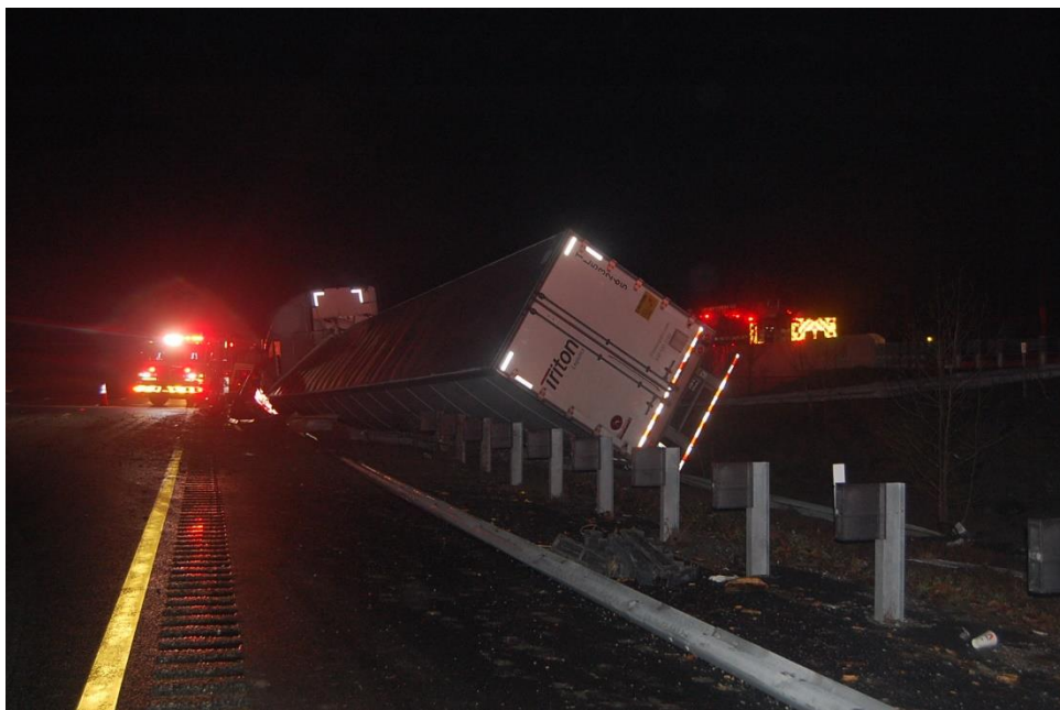
Highway Factors Photo 4 – View of strong post blocked-out W-beam guardrail that contained the Freightliner combination vehicle within the median standing in the paved shoulder adjacent to the leftmost travel lane in the westbound direction looking to the southeast (Source: Virginia State Police)
