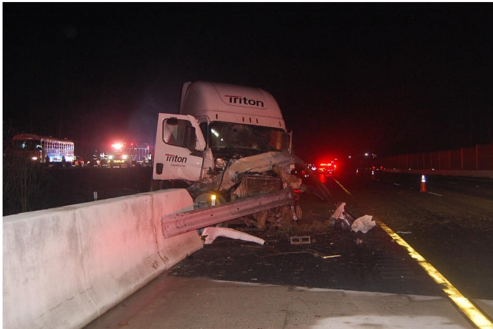
Highway Factors Photo 2 – View of strong post blocked-out W-beam guardrail that contained the Freightliner combination vehicle within the median standing in the paved shoulder adjacent to the leftmost travel lane in the westbound direction looking to the northwest (Source: Virginia State Police)
