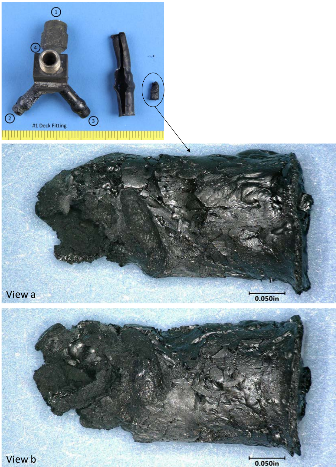
Figure 8 Images of the plug submitted with the #1 deck drain fitting. Most likely this plug was removed from port 2 as indicated in Figure 4.
