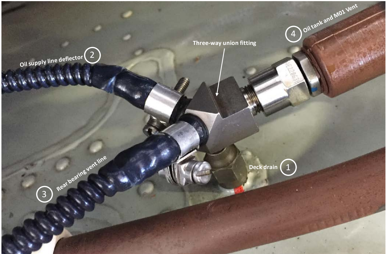
Figure 3 Typical engine deck drain fitting (also known as a three-way union fitting) showing the function and numbering scheme for each port on the deck fitting.
