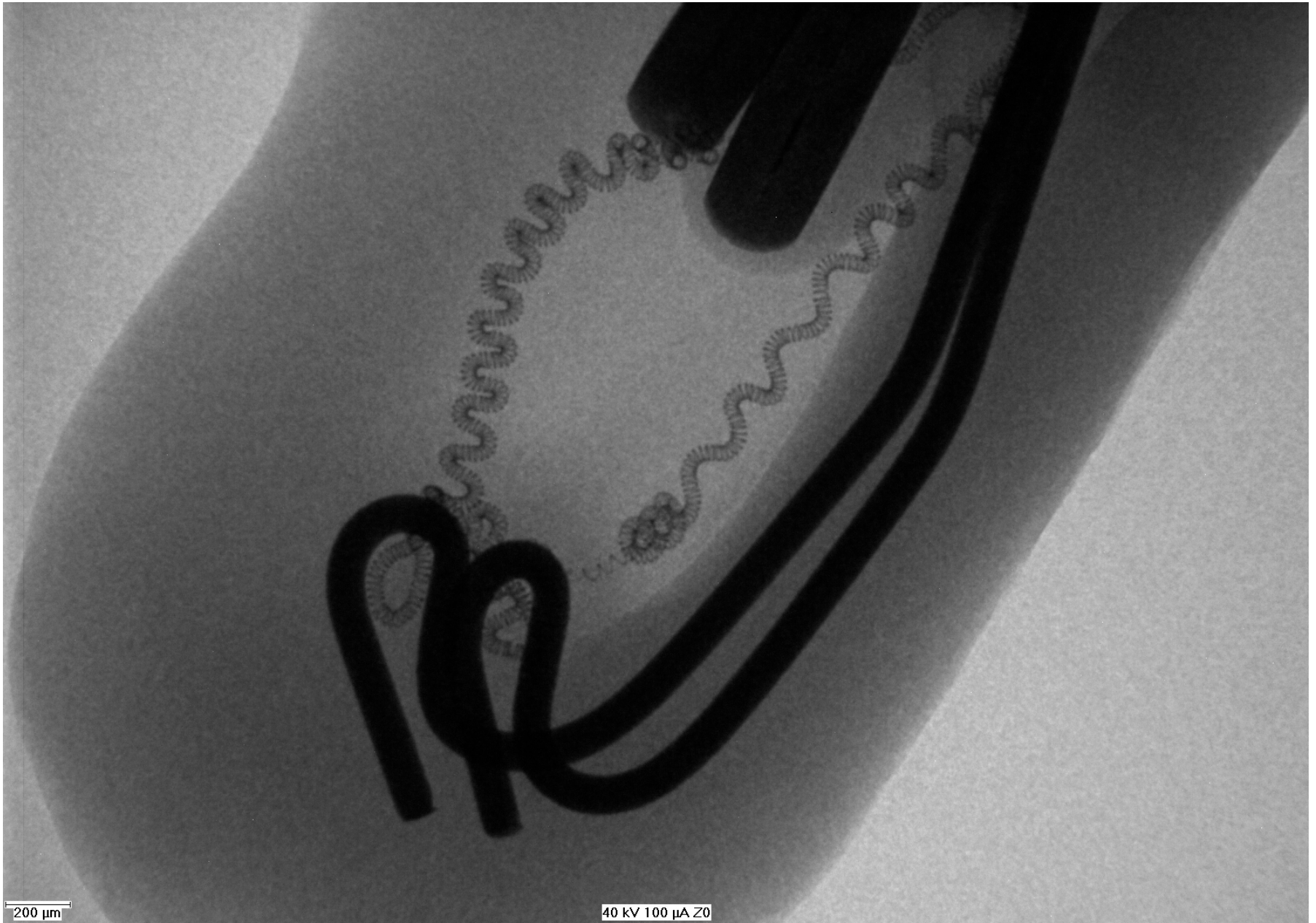
Photo 5 - X-ray radiograph of a light bulb filament and posts.
