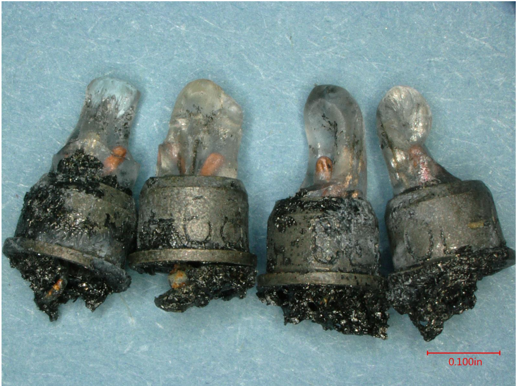
Photo 1 – Four light bulbs from the #2 FIRE light located on the cockpit instrument panel, magnified 20x.
