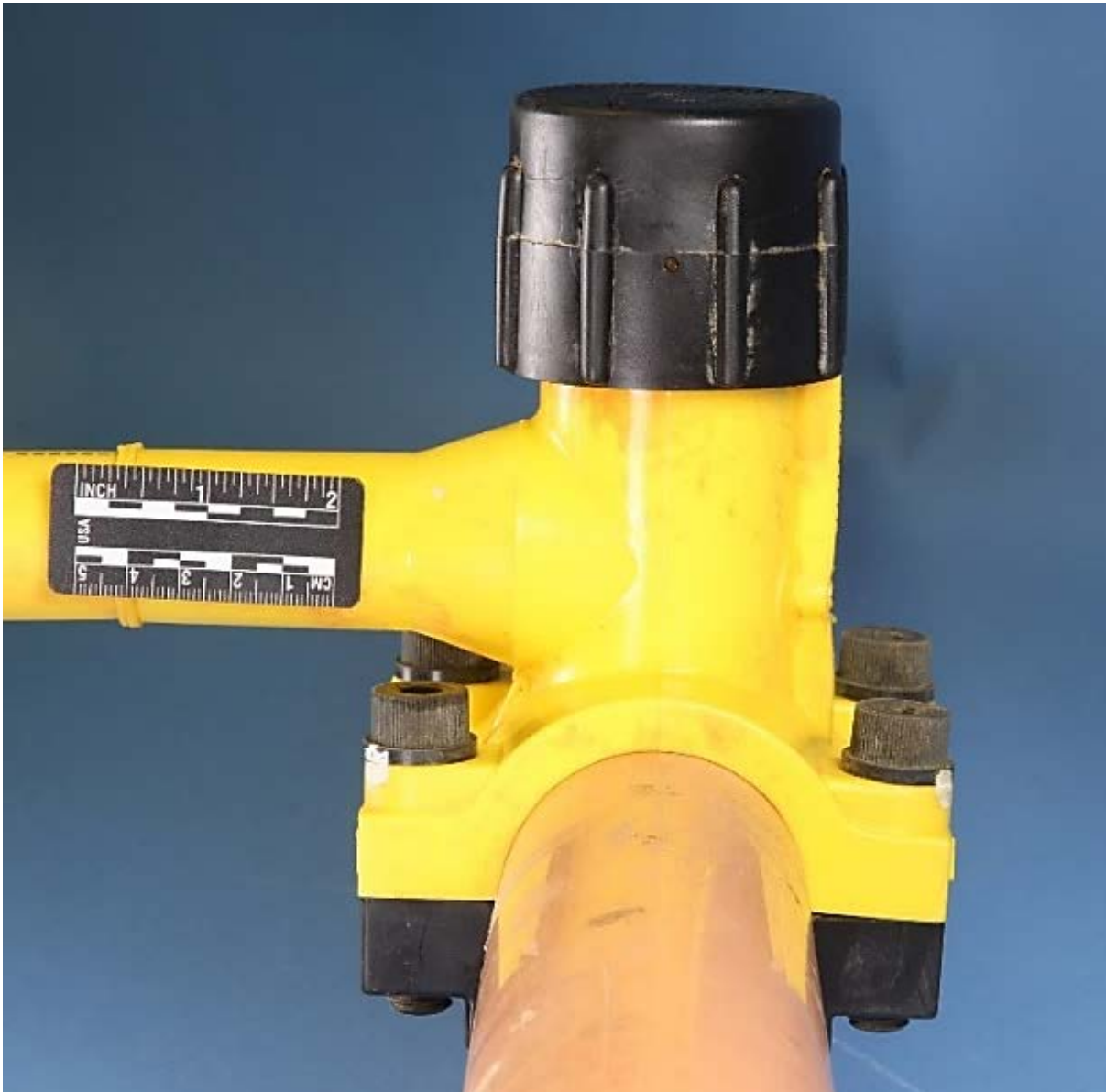
Figure 23. Photograph of the tee assembly from dwelling 201 showing the side view.
