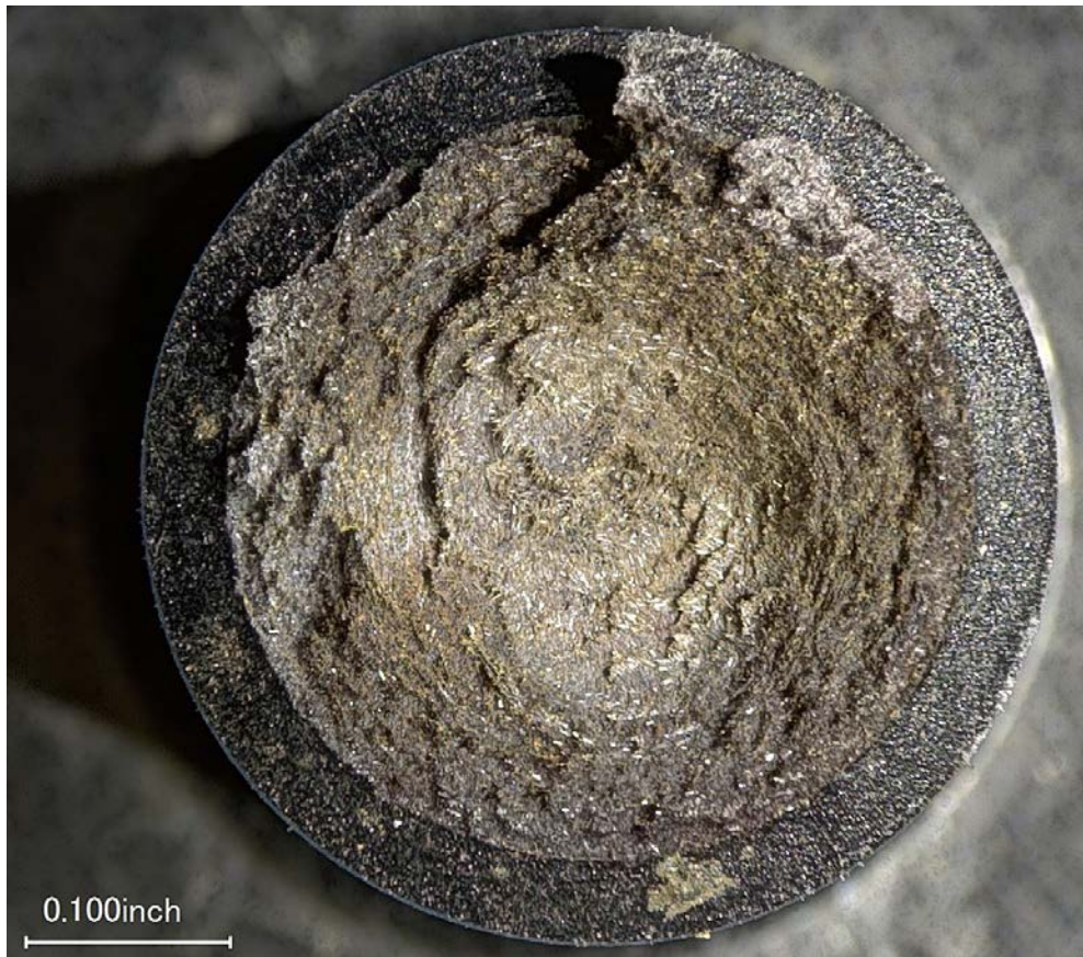
Figure 11. Fracture face of Nylon bolt "2" after ultrasonic cleaning.
