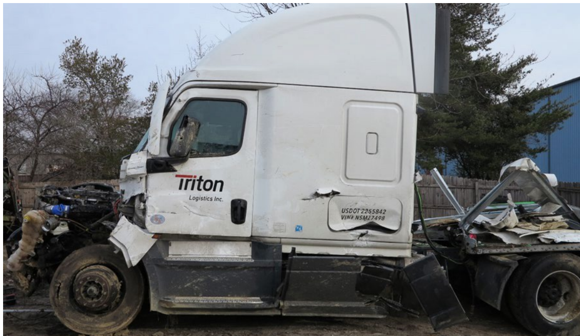
Photo 8. The damage sustained to the left side of the truck-tractor.
