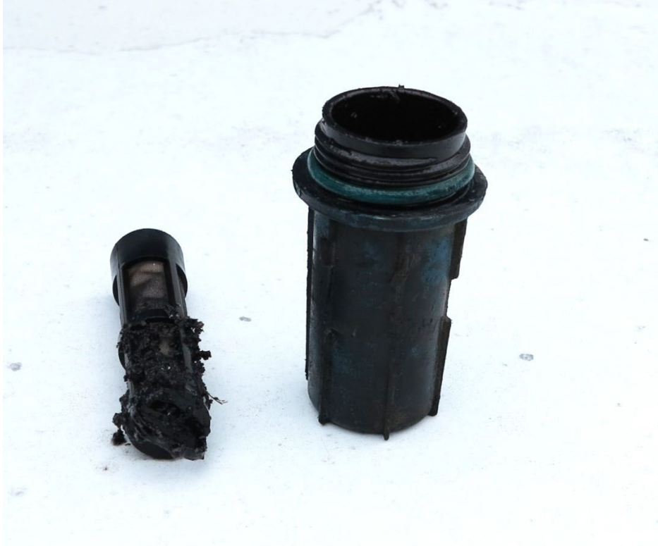
Photo 5. The partially blocked prescreen fuel filter from the bus.
