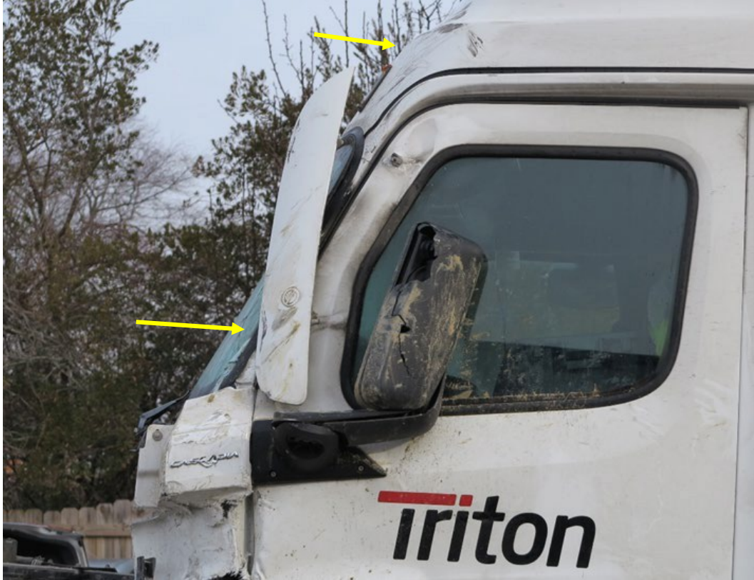
Photo 9. The arrows are pointing to some paint transfer from the bus.
