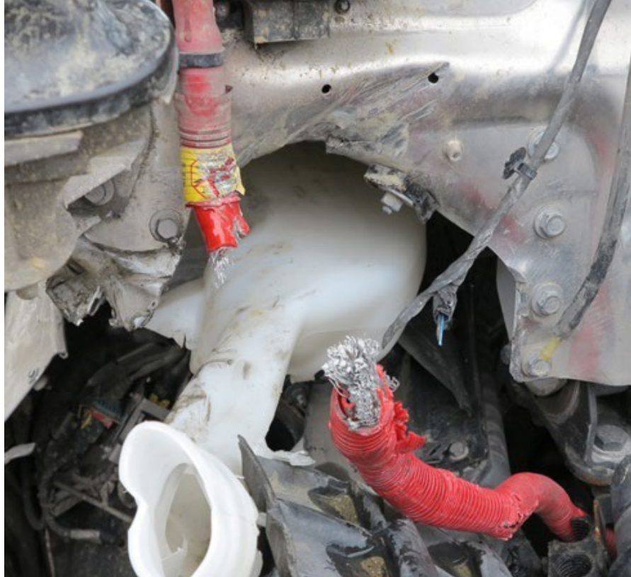
Photo 7. The severed power cable to the vehicle control modules.
